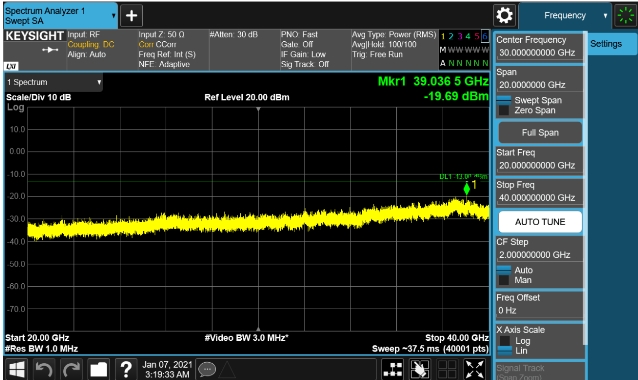
Plot 7-6. Conducted Spurious Plot (NR Band n77 PC2 SRS-2 - 100MHz DFT-s-QPSK - RB Size 1, RB Offset 0 - Mid Channel)
