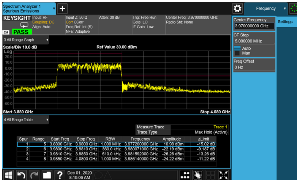
Plot 7-323. Upper ACP Plot (NR Band n77 - 60MHz CP-OFDM-QPSK – Full RB Configuration)
