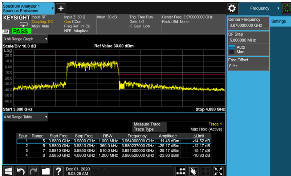
Plot 7-325. Upper ACP Plot (NR Band n77 - 50MHz CP-OFDM-QPSK – Full RB Configuration)
