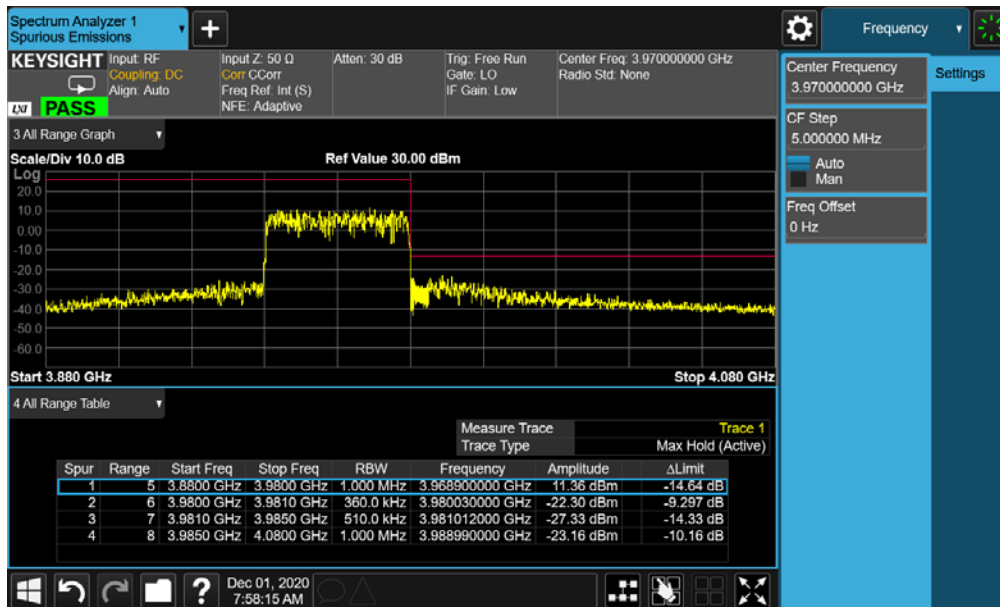
Plot 7-327. Upper ACP Plot (NR Band n77 - 40MHz CP-OFDM-QPSK – Full RB Configuration)
