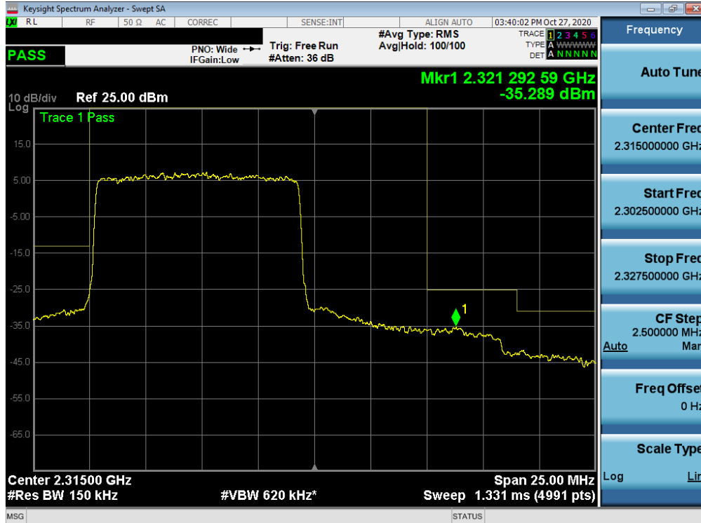
Plot 7-282. Upper ACP Plot (NR Band n30 - 10MHz CP-OFDM-QPSK – Full RB Configuration)
