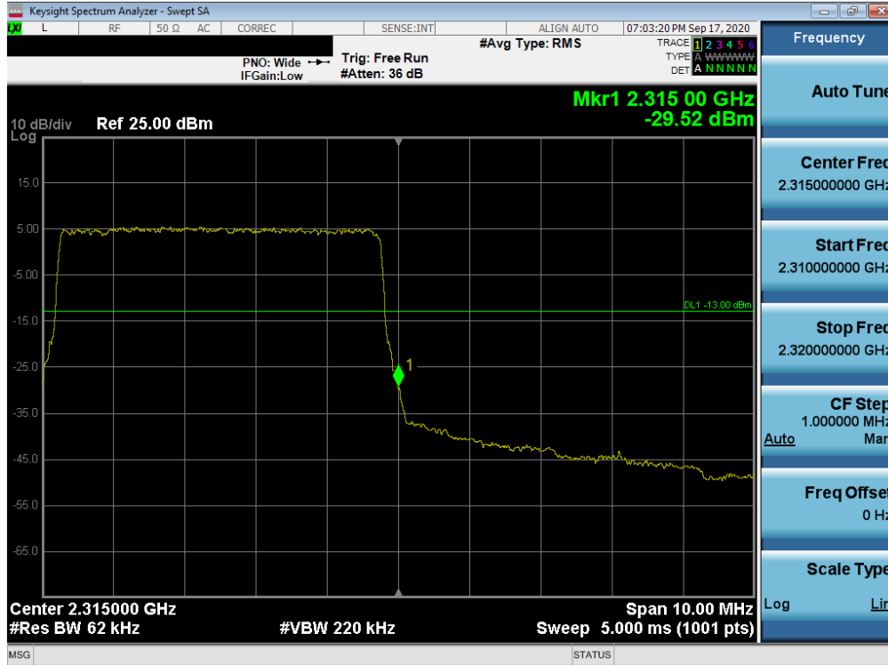
Plot 7-254. Upper Band Edge Plot (LTE Band 30 - 5MHz QPSK – Full RB Configuration)
