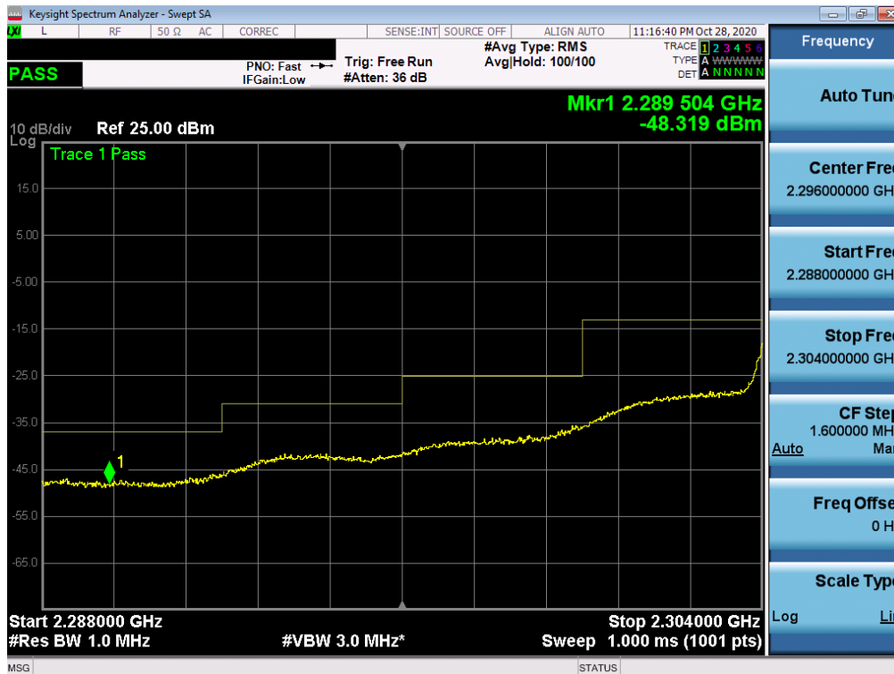
Plot 7-281. Lower ACP Plot (NR Band n30 - 10MHz CP-OFDM-QPSK – Full RB Configuration)
