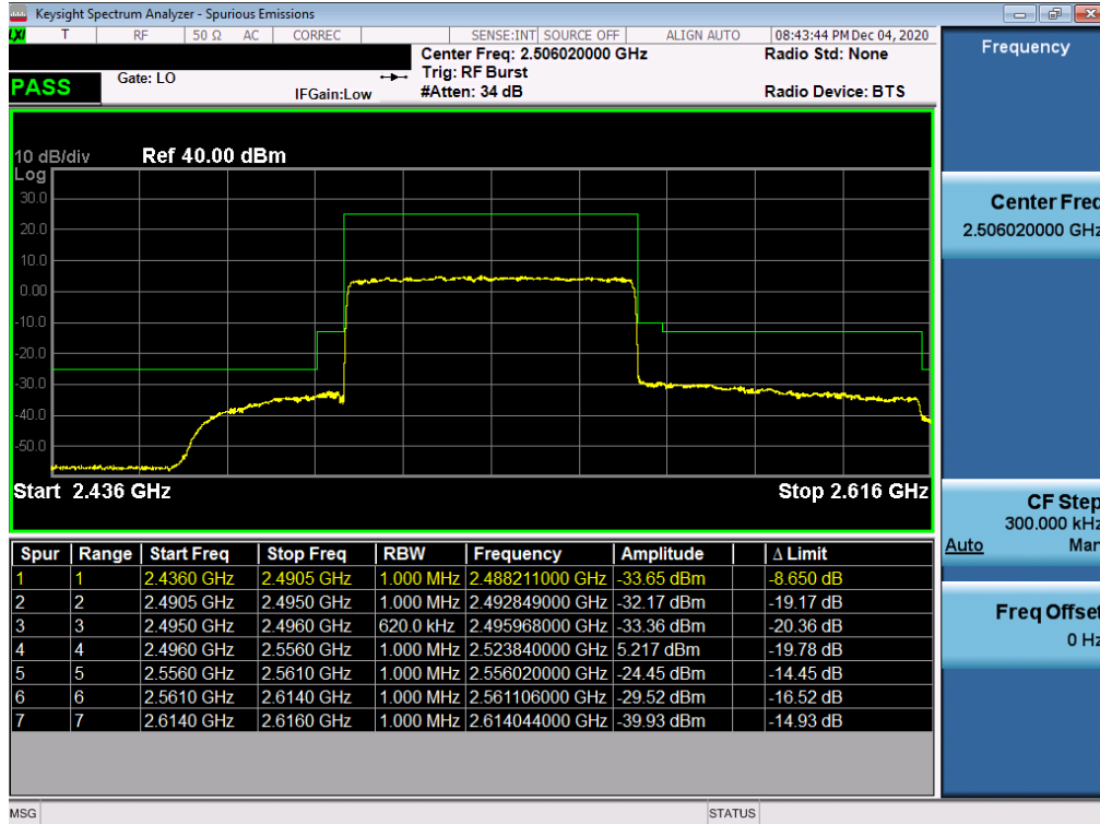
Plot 7-306. Lower ACP Plot (NR Band n41 PC3 – Antenna B - 60MHz CP-OFDM-QPSK – Full RB Configuration)
