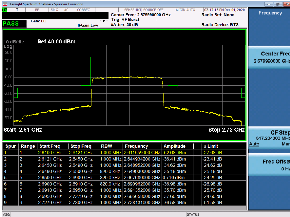
Plot 7-297. Upper ACP Plot (NR Band n41 - 40MHz CP-OFDM-QPSK – Full RB Configuration)
