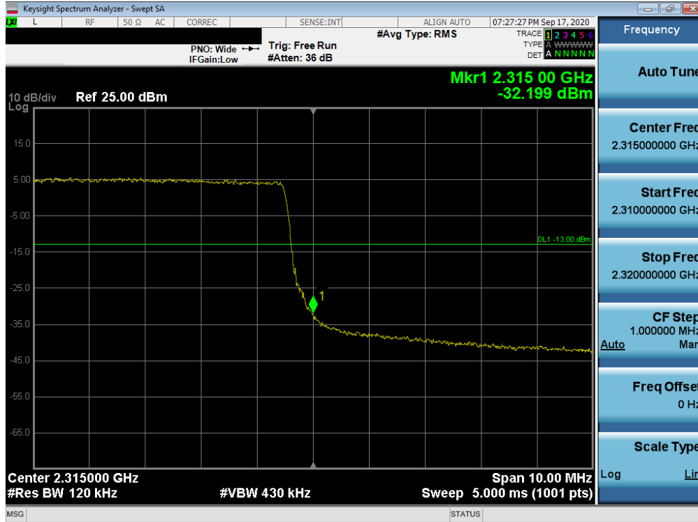
Plot 7-250. Upper Band Edge Plot (LTE Band 30 - 10MHz QPSK – Full RB Configuration)
