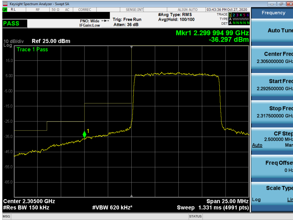
Plot 7-280. Lower ACP Plot (NR Band n30 - 10MHz CP-OFDM-QPSK – Full RB Configuration)
