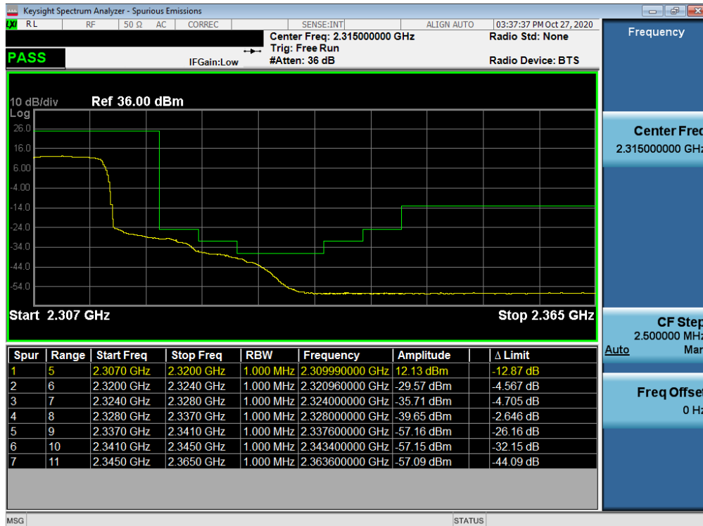
Plot 7-283. Upper ACP Plot (NR Band n30 - 10MHz CP-OFDM-QPSK – Full RB Configuration)
