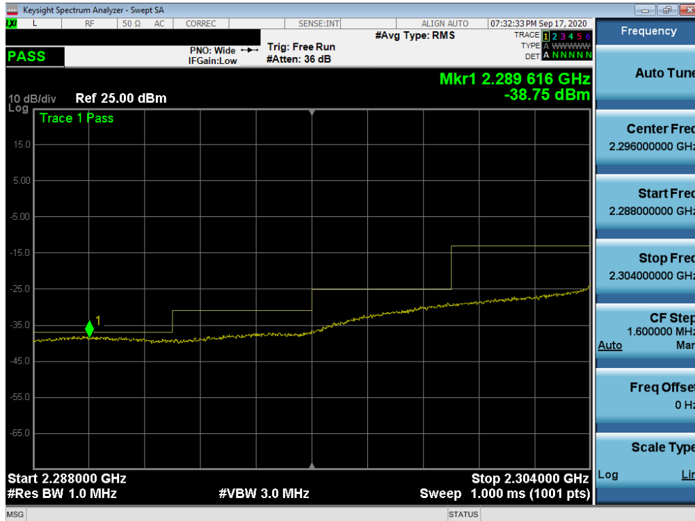
Plot 7-249. Extended Lower Band Edge Plot (LTE Band 30 - 10MHz QPSK – Full RB Configuration)
