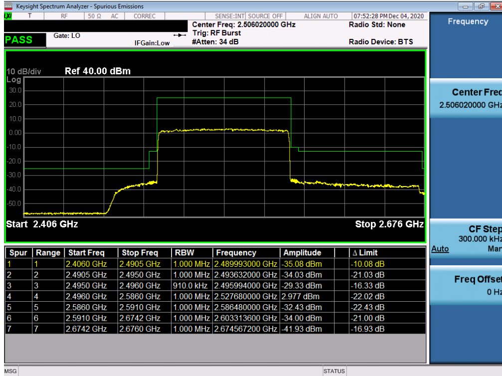
Plot 7-302. Lower ACP Plot (NR Band n41 PC3 – Antenna B - 90MHz CP-OFDM-QPSK – Full RB Configuration)
