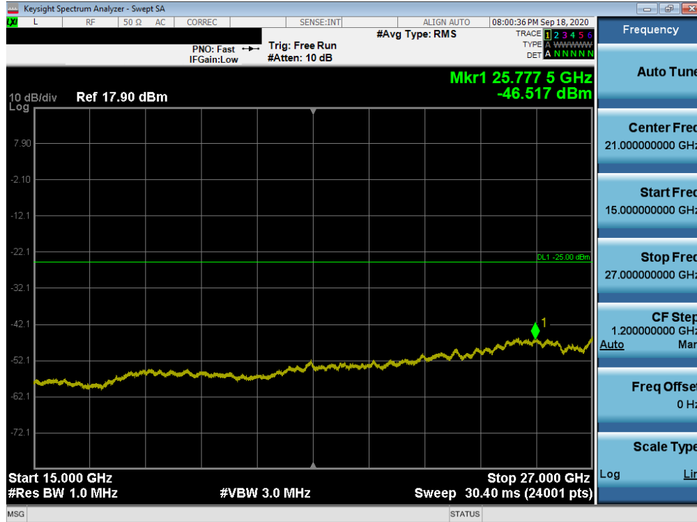
Plot 7-199. Conducted Spurious Plot (LTE Band 7 - 20MHz QPSK - RB Size 1, RB Offset 0 - High Channel)
