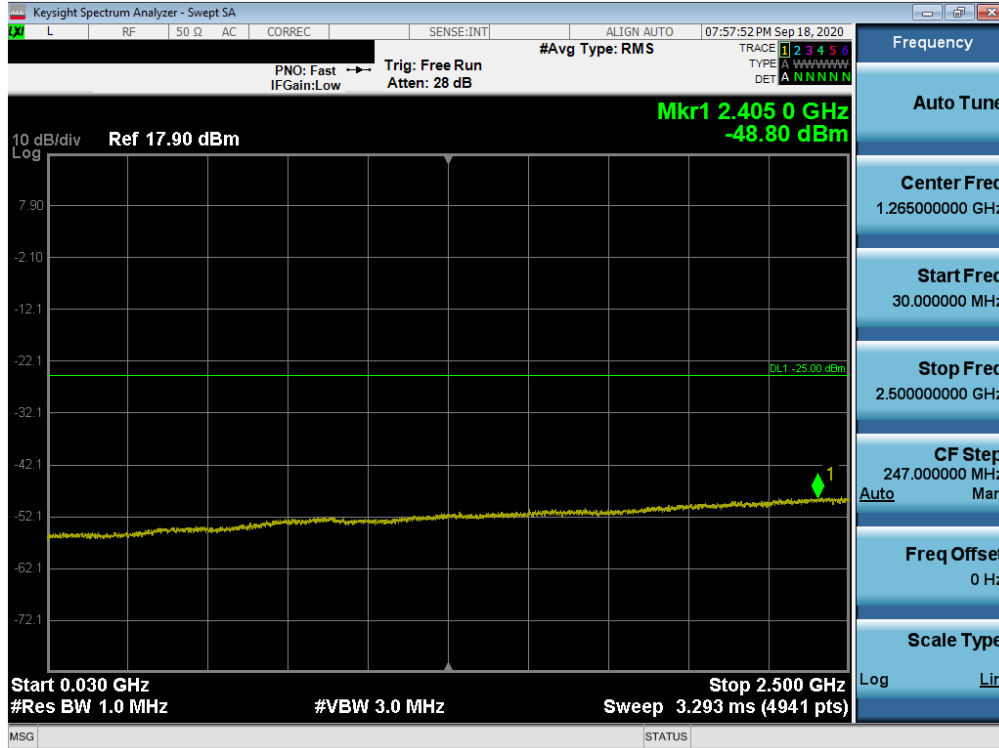
Plot 7-197. Conducted Spurious Plot (LTE Band 7 - 20MHz QPSK - RB Size 1, RB Offset 0 - High Channel)
