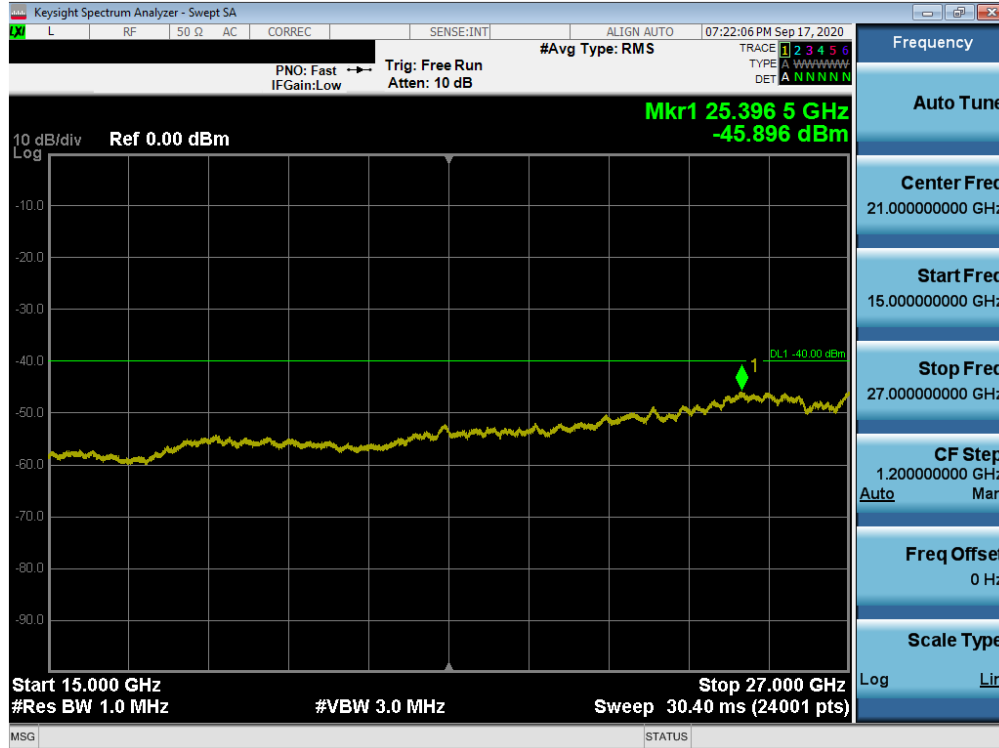
Plot 7-190. Conducted Spurious Plot (LTE Band 30 - 10MHz QPSK - RB Size 1, RB Offset 0)
