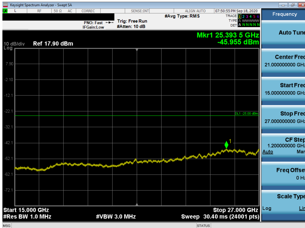
Plot 7-196. Conducted Spurious Plot (LTE Band 7 - 20MHz QPSK - RB Size 1, RB Offset 0 - Mid Channel)
