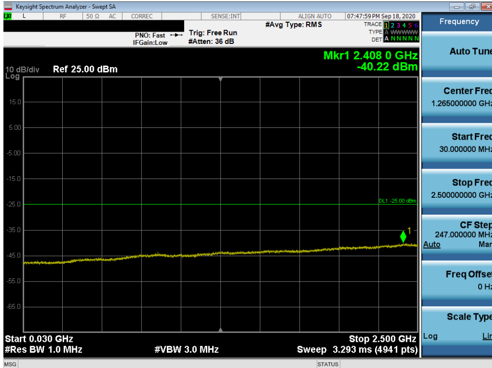
Plot 7-194. Conducted Spurious Plot (LTE Band 7 - 20MHz QPSK - RB Size 1, RB Offset 0 - Mid Channel)
