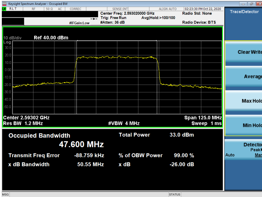
Plot 7-89. Occupied Bandwidth Plot (NR Band n41 - 50MHz QPSK - Full RB Configuration)
