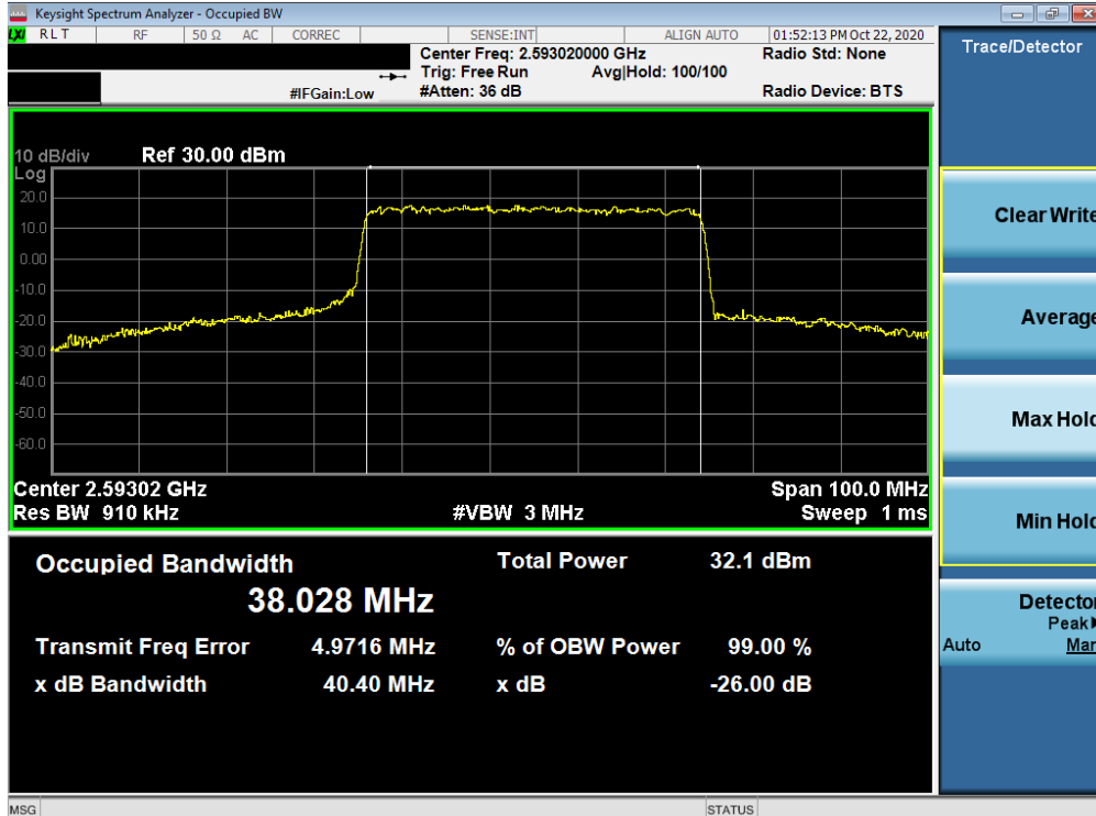
Plot 7-94. Occupied Bandwidth Plot (NR Band n41 - 40MHz QPSK - Full RB Configuration)
