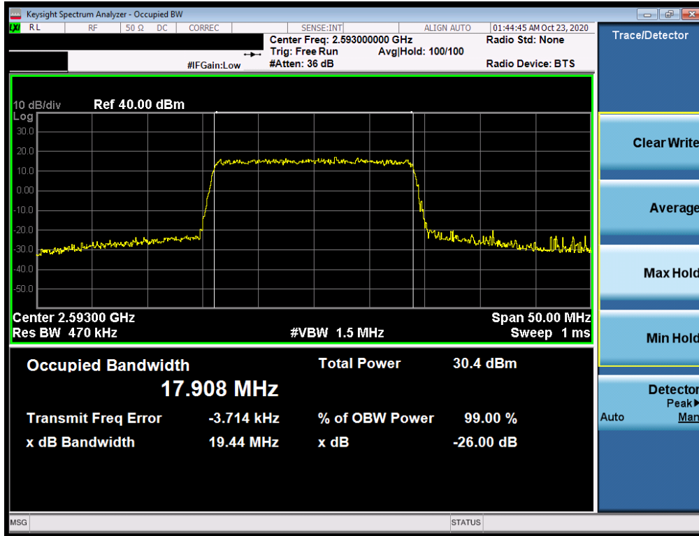
Plot 7-44. Occupied Bandwidth Plot (LTE Band 41(PC3)/38 - 20MHz 64-QAM - Full RB Configuration)
