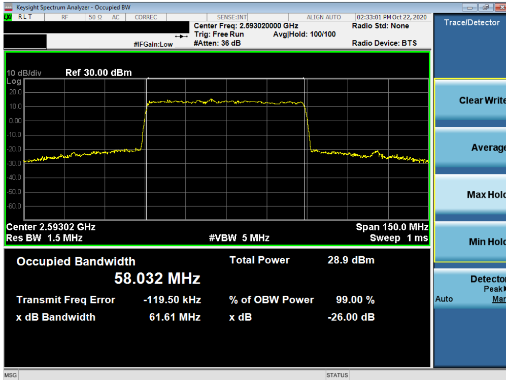
Plot 7-87. Occupied Bandwidth Plot (NR Band n41 - 60MHz 256-QAM - Full RB Configuration)
