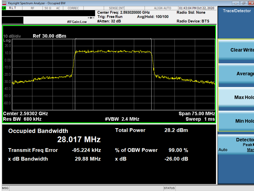
Plot 7-102. Occupied Bandwidth Plot (NR Band n41 - 30MHz 256-QAM - Full RB Configuration)
