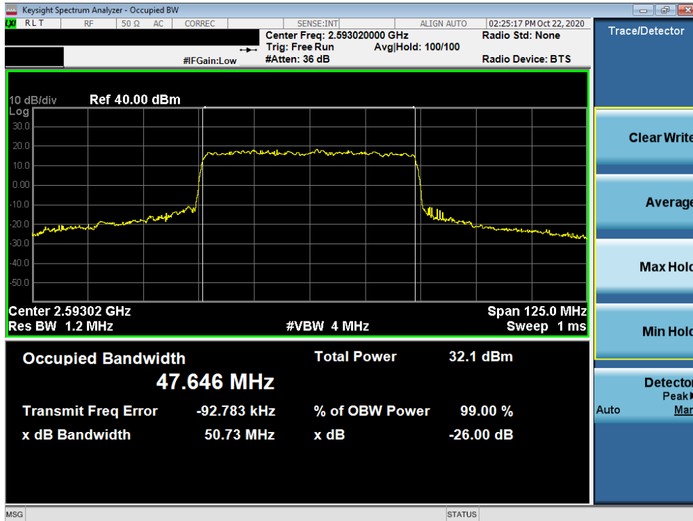
Plot 7-91. Occupied Bandwidth Plot (NR Band n41 - 50MHz 64-QAM - Full RB Configuration)
