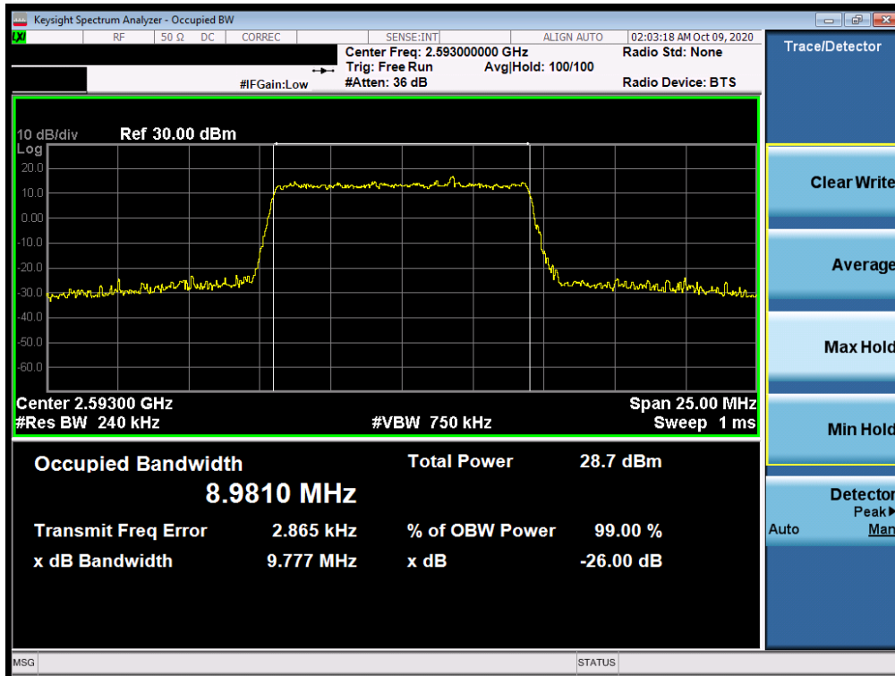
Plot 7-37. Occupied Bandwidth Plot (LTE Band 41(PC2) - 10MHz 256-QAM - Full RB Configuration)
