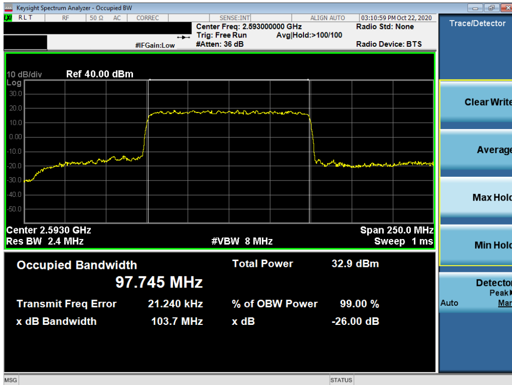
Plot 7-69. Occupied Bandwidth Plot (NR Band n41 - 100MHz QPSK - Full RB Configuration)
