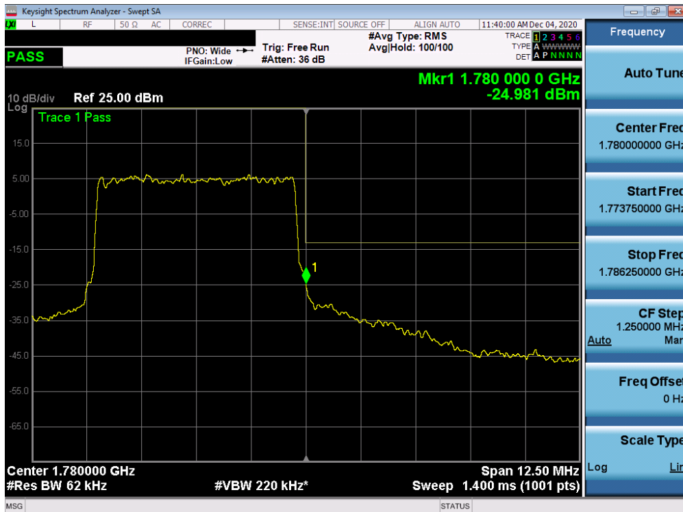
Plot 7-313. Upper Band Edge Plot (NR Band n66 Ant I – 5.0MHz - Full RB)
