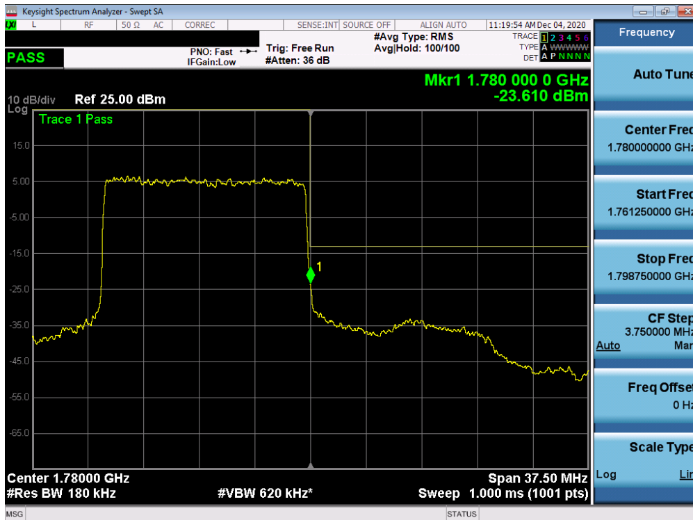
Plot 7-309. Upper Band Edge Plot (NR Band n66 Ant I – 15.0MHz - Full RB)
