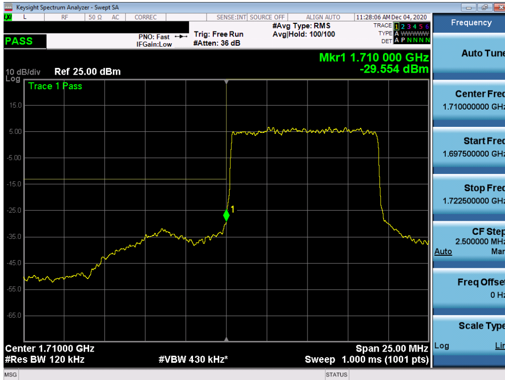
Plot 7-310. Lower Band Edge Plot (NR Band n66 Ant I – 10.0MHz - Full RB)
