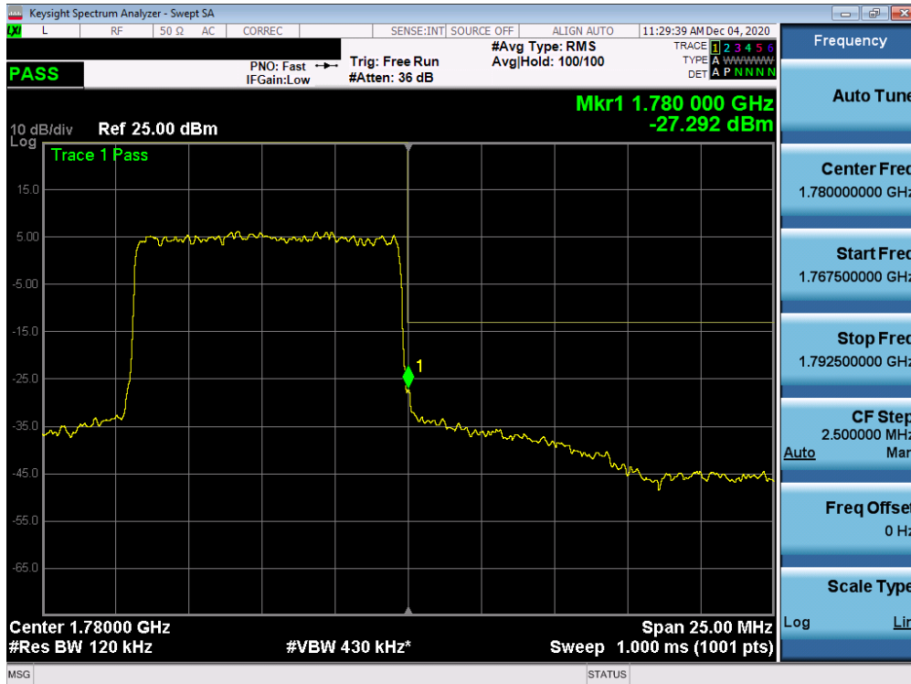
Plot 7-311. Upper Band Edge Plot (NR Band n66 Ant I – 10.0MHz - Full RB)
