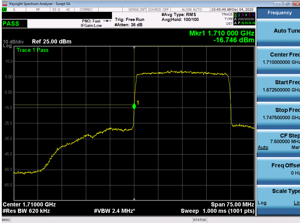
Plot 7-304. Lower Band Edge Plot (NR Band n66 Ant I – 30.0MHz - Full RB)
