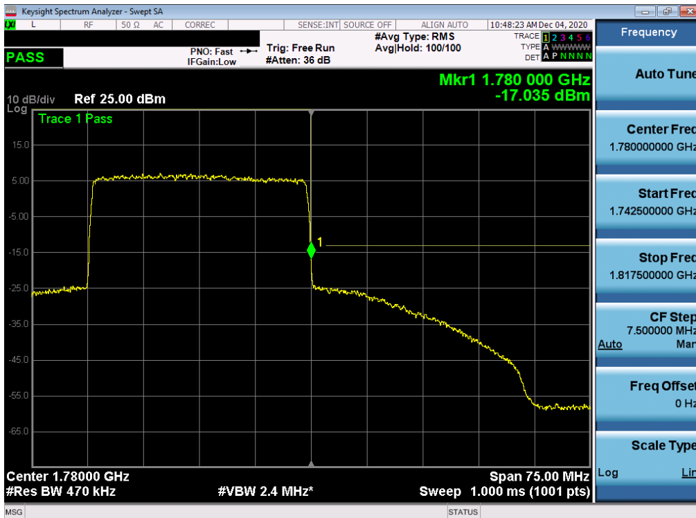
Plot 7-305. Upper Band Edge Plot (NR Band n66 Ant I – 30.0MHz - Full RB)
