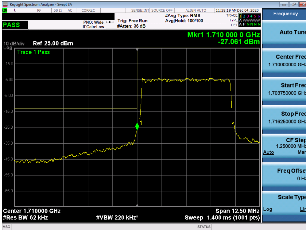
Plot 7-312. Lower Band Edge Plot (NR Band n66 Ant I – 5.0MHz - Full RB)
