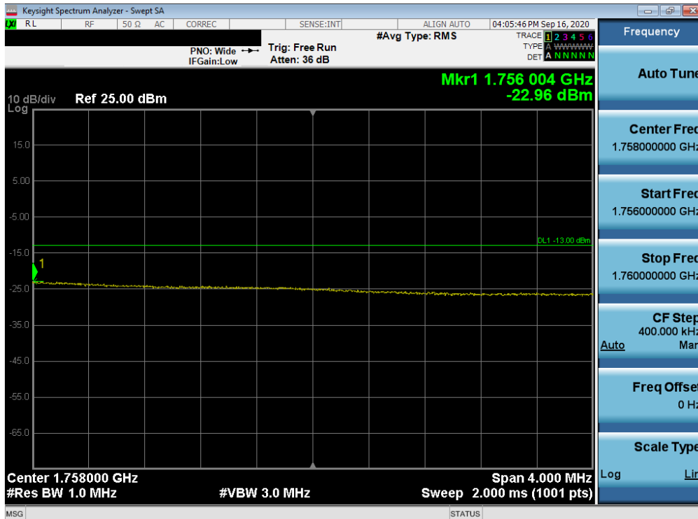
Plot 7-227. Upper Extended Band Edge Plot (LTE Band 4 - 15MHz QPSK – Full RB Configuration)
