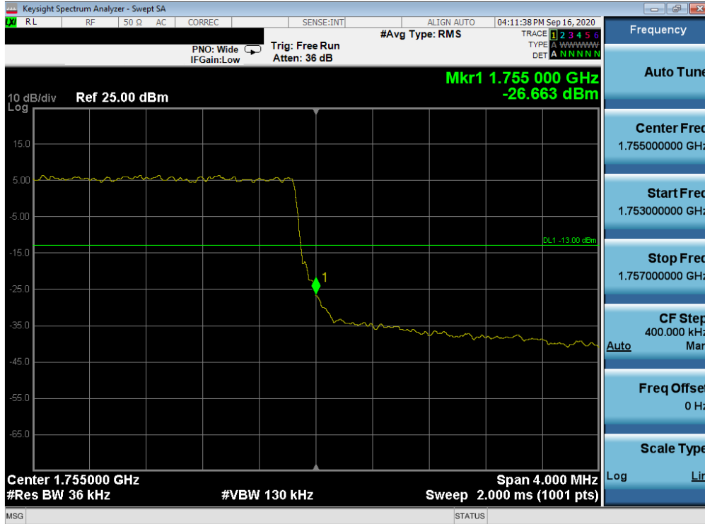
Plot 7-244. Upper Band Edge Plot (LTE Band 4 - 3MHz QPSK – Full RB Configuration)
