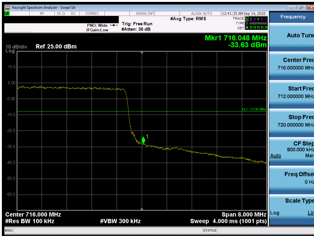
Plot 7-255. Upper Band Edge Plot (LTE Band 12 - 10MHz QPSK – Full RB Configuration)
