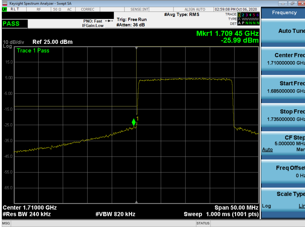
Plot 7-286. Lower Band Edge Plot (NR Band n66 Ant A – 20.0MHz - Full RB)
