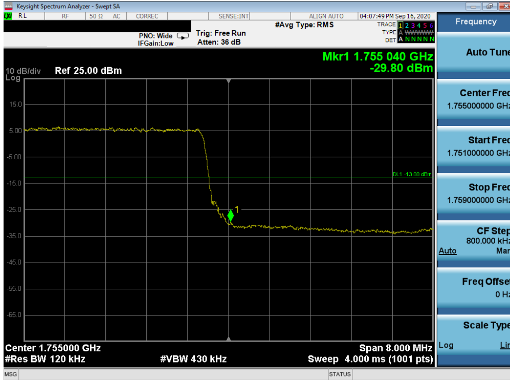
Plot 7-232. Upper Band Edge Plot (LTE Band 4 - 10MHz QPSK – Full RB Configuration)
