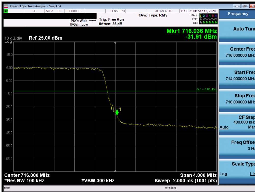
Plot 7-257. Upper Band Edge Plot (LTE Band 12 - 5MHz QPSK – Full RB Configuration)
