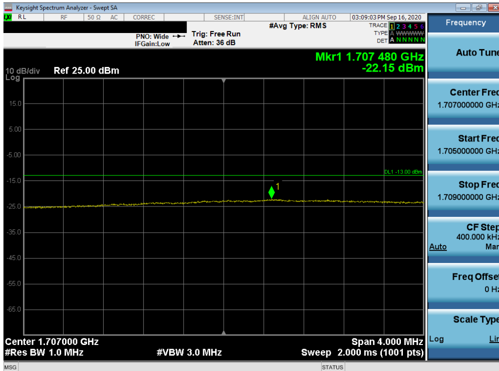
Plot 7-225. Lower Extended Band Edge Plot (LTE Band 66/4 - 15MHz QPSK – Full RB Configuration)
