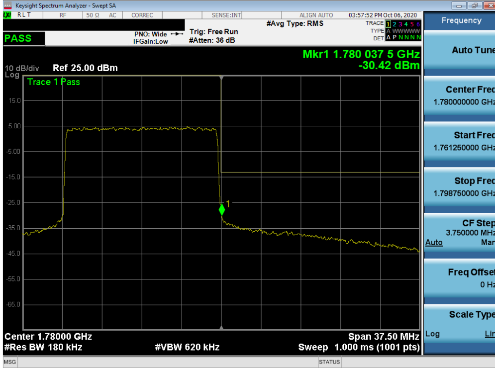
Plot 7-292. Upper Band Edge Plot (NR Band n66 Ant A – 15.0MHz - Full RB)
