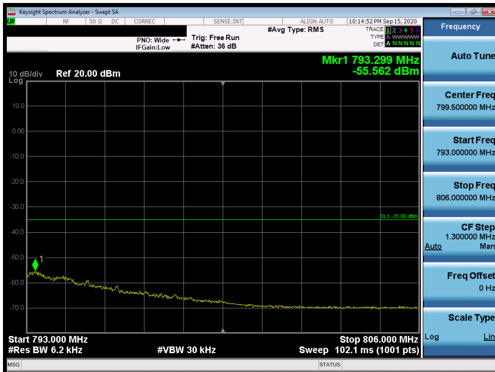
Plot 7-269. Upper Emission Mask Plot (LTE Band 13 - 5MHz QPSK – Full RB Configuration)
