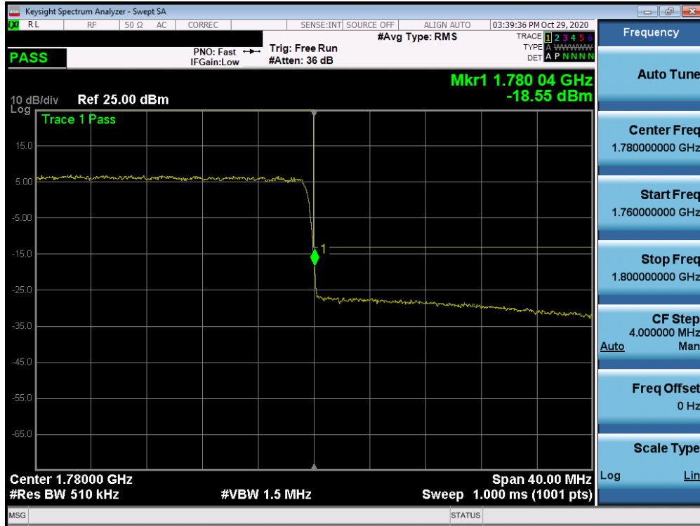
Plot 7-280. Upper Band Edge Plot (NR Band n66 Ant A – 40.0MHz - Full RB)
