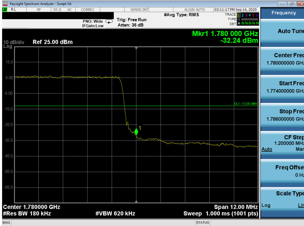
Plot 7-228. Upper Band Edge Plot (LTE Band 66 - 15MHz QPSK – Full RB Configuration)
