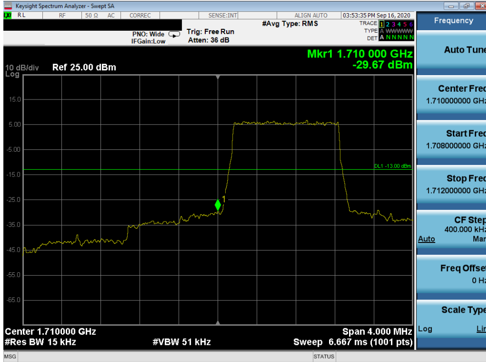
Plot 7-248. Lower Band Edge Plot (LTE Band 66/4 – 1.4MHz QPSK – Full RB Configuration)
