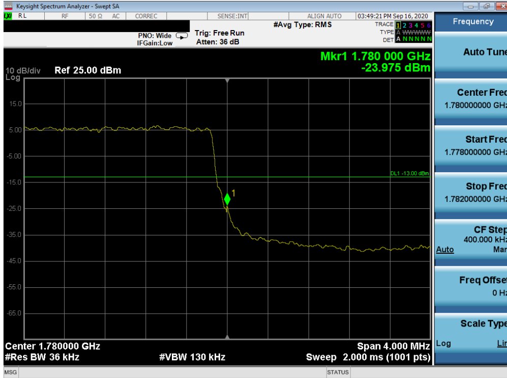
Plot 7-246. Upper Band Edge Plot (LTE Band 66 - 3MHz QPSK – Full RB Configuration)
