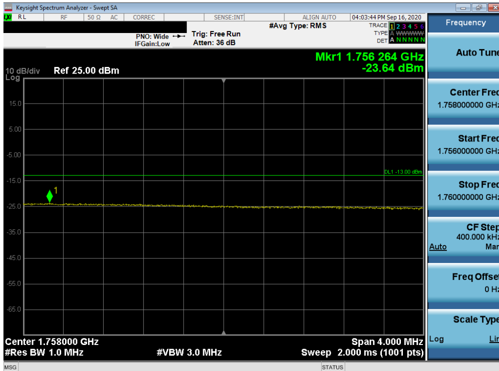
Plot 7-221. Upper Extended Band Edge Plot (LTE Band 4 - 20MHz QPSK – Full RB Configuration)
