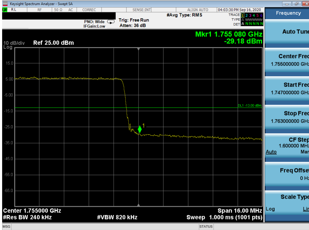
Plot 7-220. Upper Band Edge Plot (LTE Band 4 - 20MHz QPSK – Full RB Configuration)
