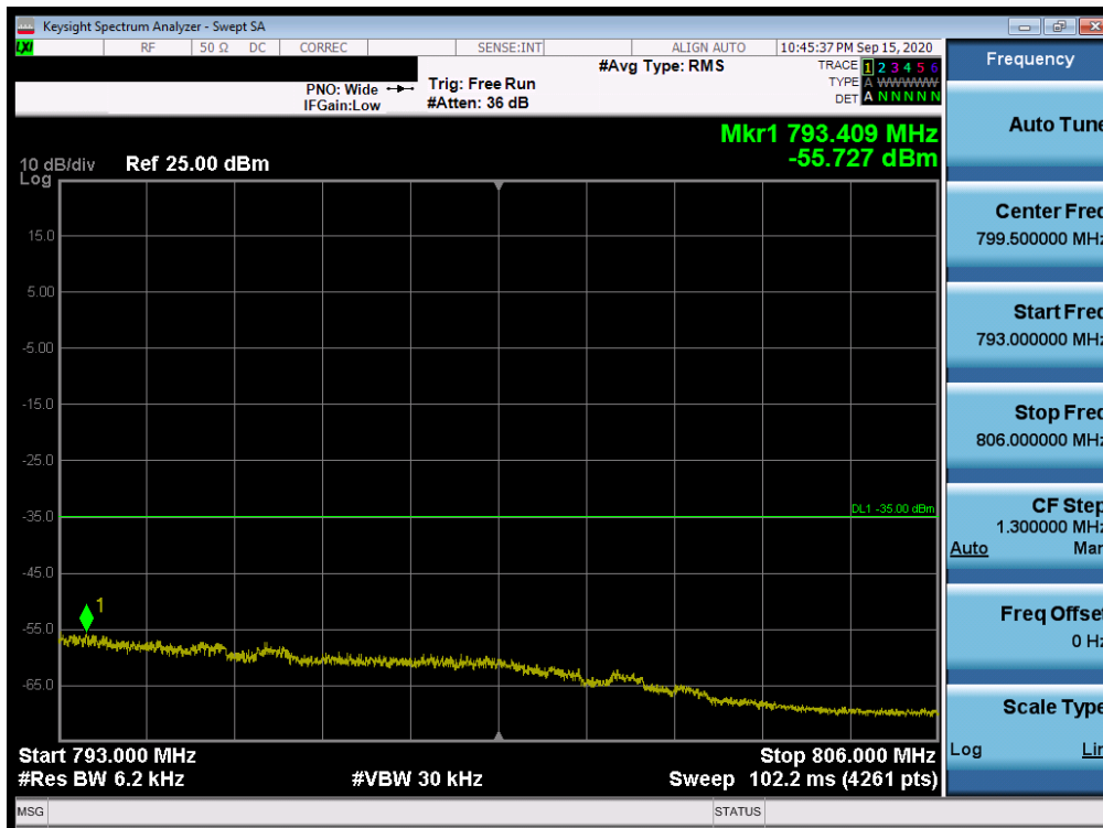
Plot 7-265. Upper Emission Mask Plot (LTE Band 13 - 10MHz QPSK – Full RB Configuration)
