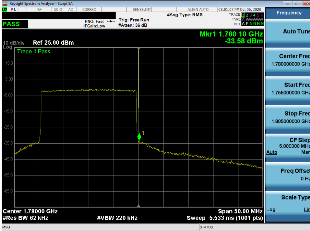
Plot 7-288. Upper Band Edge Plot (NR Band n66 Ant A – 20.0MHz - Full RB)
