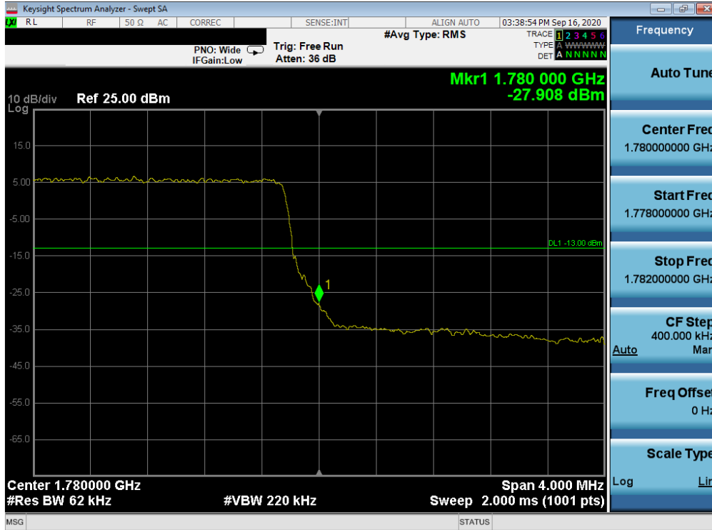
Plot 7-240. Upper Band Edge Plot (LTE Band 66 - 5MHz QPSK – Full RB Configuration)
