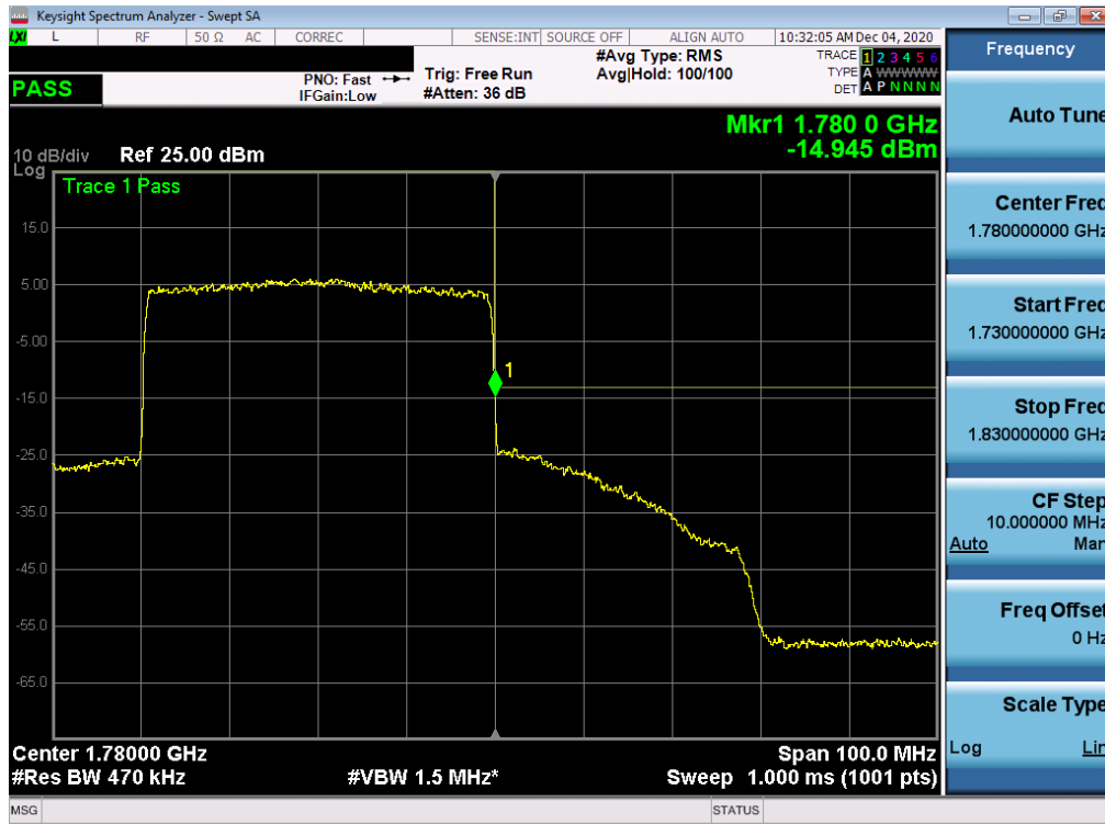
Plot 7-303. Upper Band Edge Plot (NR Band n66 Ant I – 40.0MHz - Full RB)
