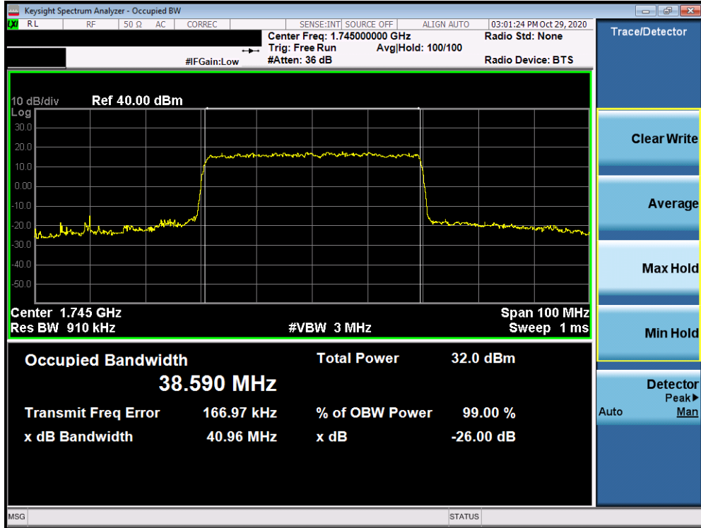
Plot 7-102. Occupied Bandwidth Plot (NR Band n66 - 40.0MHz CP-OFDM 16QAM - Full RB ANTENNA A)
