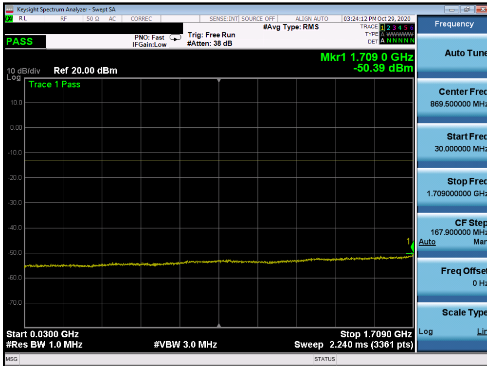
Plot 7-170. Conducted Spurious Plot (NR Band n66 - 40.0MHz - RB Size 1, RB Offset 0 - Low Channel)
