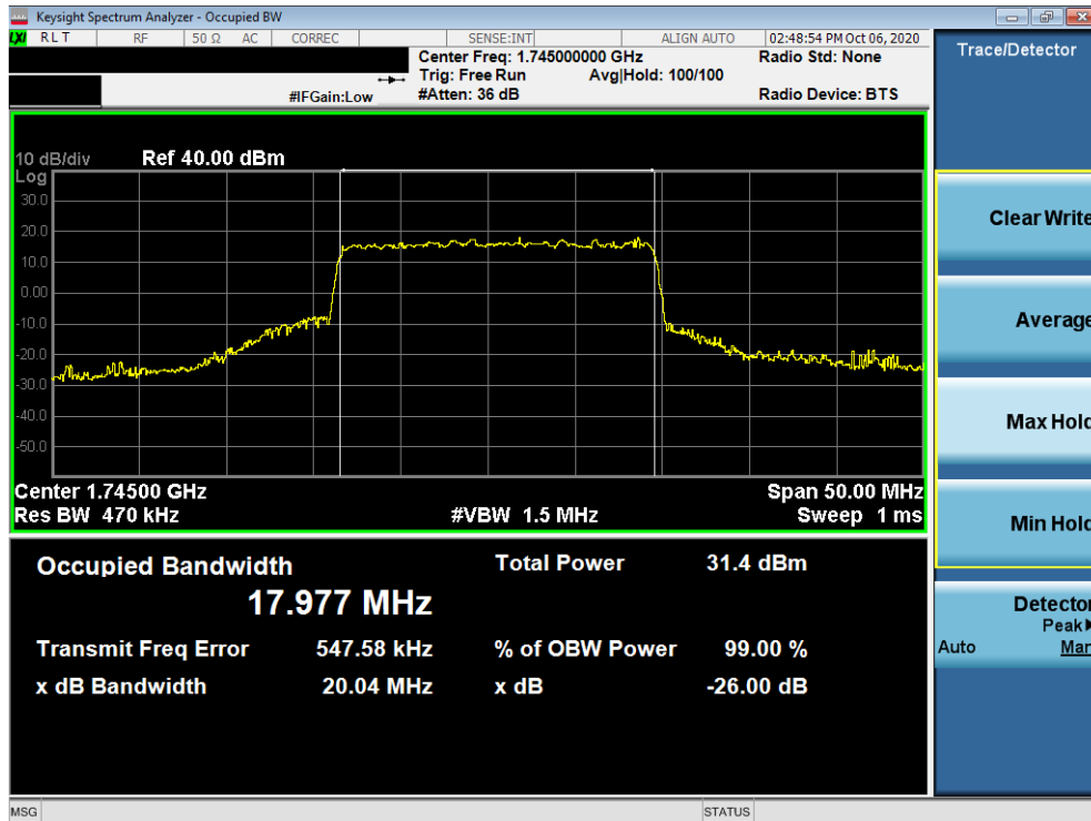
Plot 7-111. Occupied Bandwidth Plot (NR Band n66 - 20.0MHz CP-OFDM QPSK - Full RB ANTENNA A)
