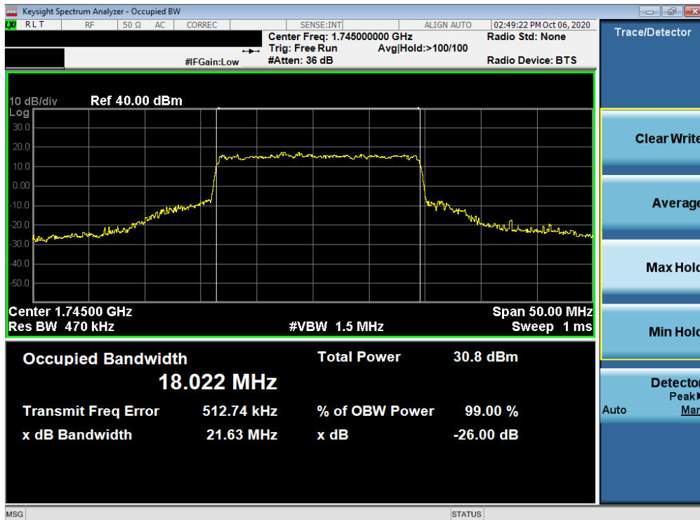
Plot 7-113. Occupied Bandwidth Plot (NR Band n66 - 20.0MHz CP-OFDM 64QAM - Full RB ANTENNA A)
