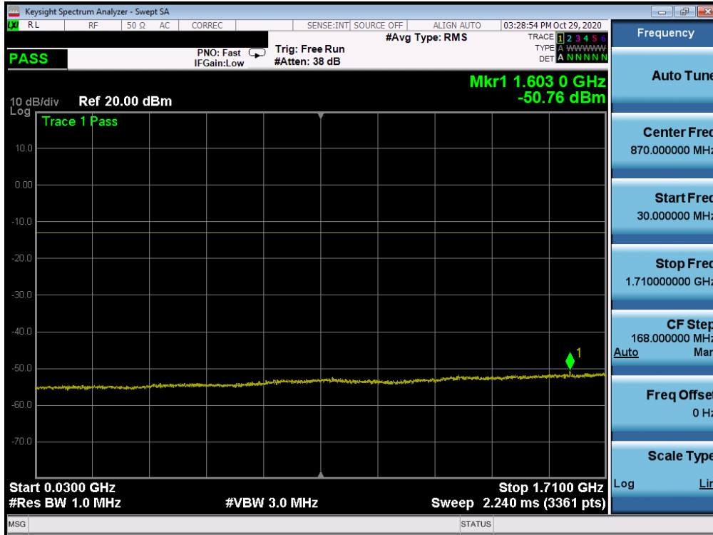
Plot 7-176. Conducted Spurious Plot (NR Band n66 - 40.0MHz - RB Size 1, RB Offset 0 - High Channel)
