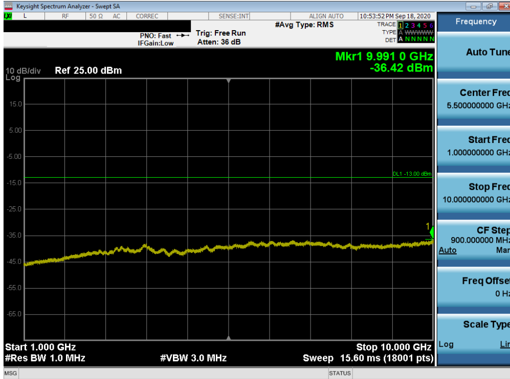
Plot 7-181. Conducted Spurious Plot (LTE Band 71 - 20MHz QPSK - RB Size 1, RB Offset 0 - Low Channel)
