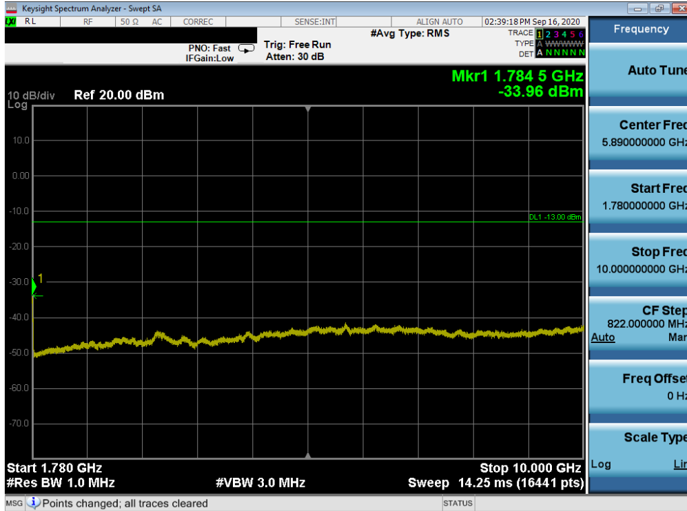
Plot 7-165. Conducted Spurious Plot (LTE Band 66/4 - 20MHz QPSK - RB Size 1, RB Offset 0 - Mid Channel)
