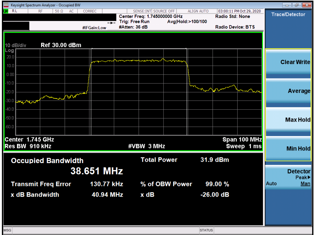
Plot 7-100. Occupied Bandwidth Plot (NR Band n66 - 40.0MHz DFT-s-OFDM BPSK - Full RB ANTENNA A)
