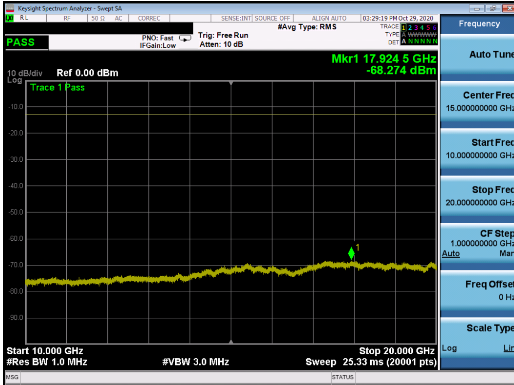
Plot 7-178. Conducted Spurious Plot (NR Band n66 - 40.0MHz - RB Size 1, RB Offset 0 - High Channel)
