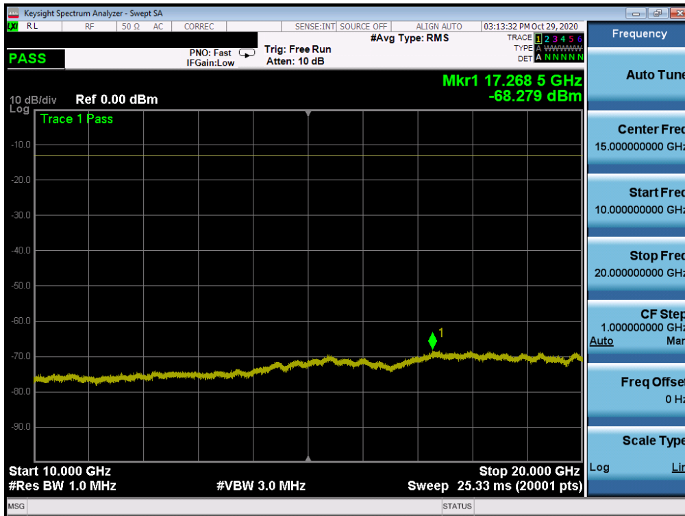
Plot 7-175. Conducted Spurious Plot (NR Band n66 - 40.0MHz - RB Size 1, RB Offset 0 - Mid Channel)
