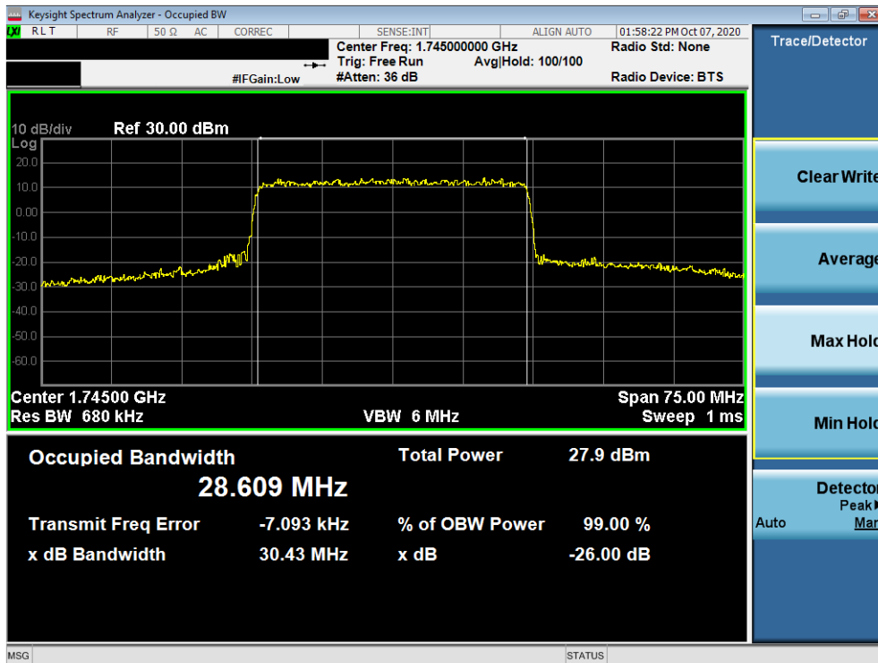
Plot 7-109. Occupied Bandwidth Plot (NR Band n66 - 30.0MHz CP-OFDM 256QAM - Full RB ANTENNA A)
