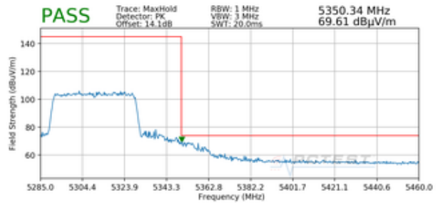
Plot 7-320. Radiated Upper Band Edge Plot SISO ANT2 (Peak – UNII Band 2A)
