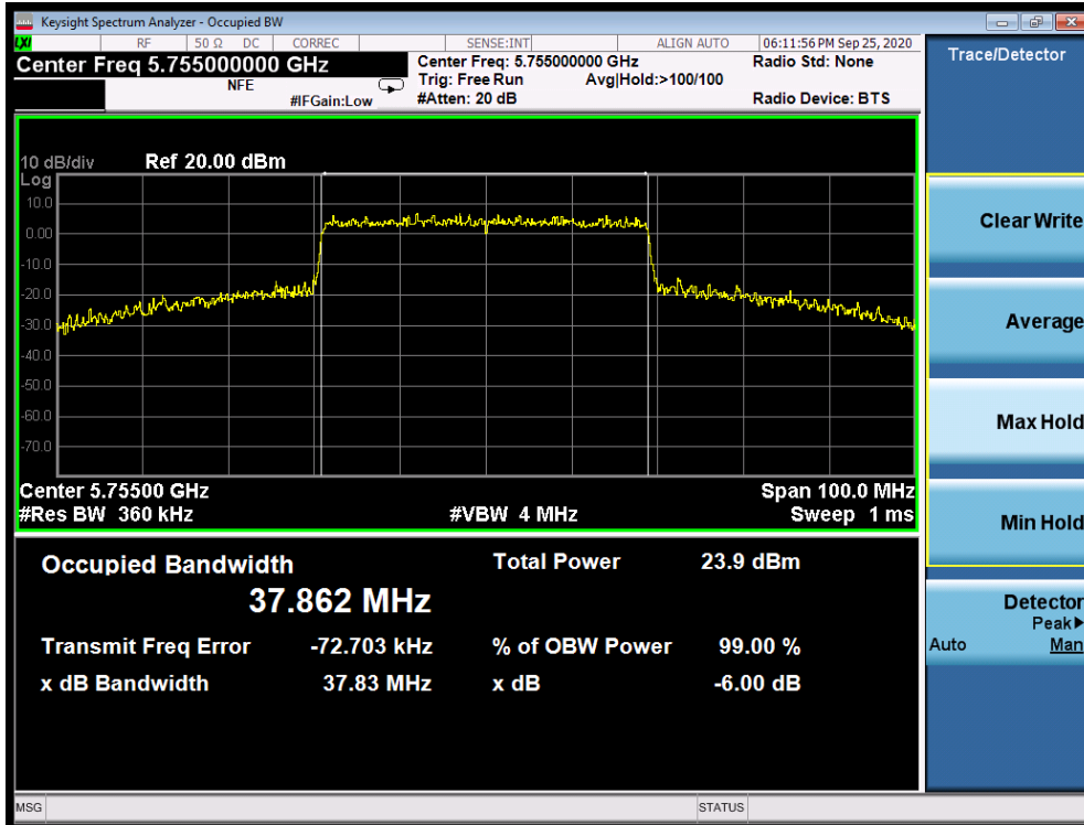
Plot 7-126. 6dB Bandwidth Plot SISO ANT2 (40MHz BW 802.11ax (UNII Band 3) – Ch. 151)
