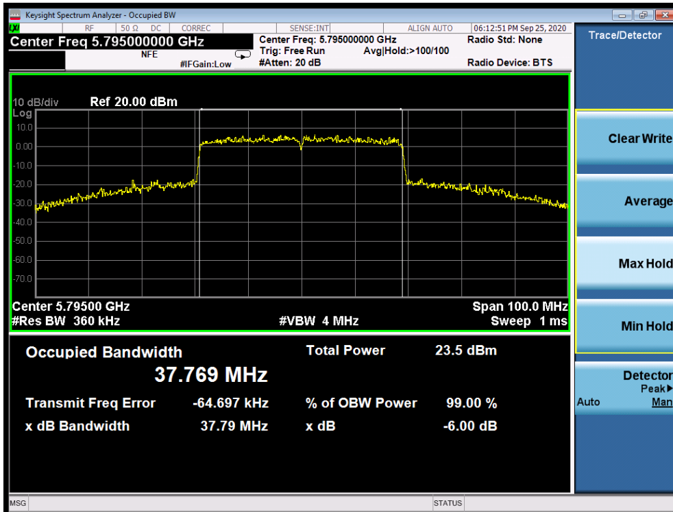
Plot 7-127. 6dB Bandwidth Plot SISO ANT2 (40MHz BW 802.11ax (UNII Band 3) – Ch. 151)
