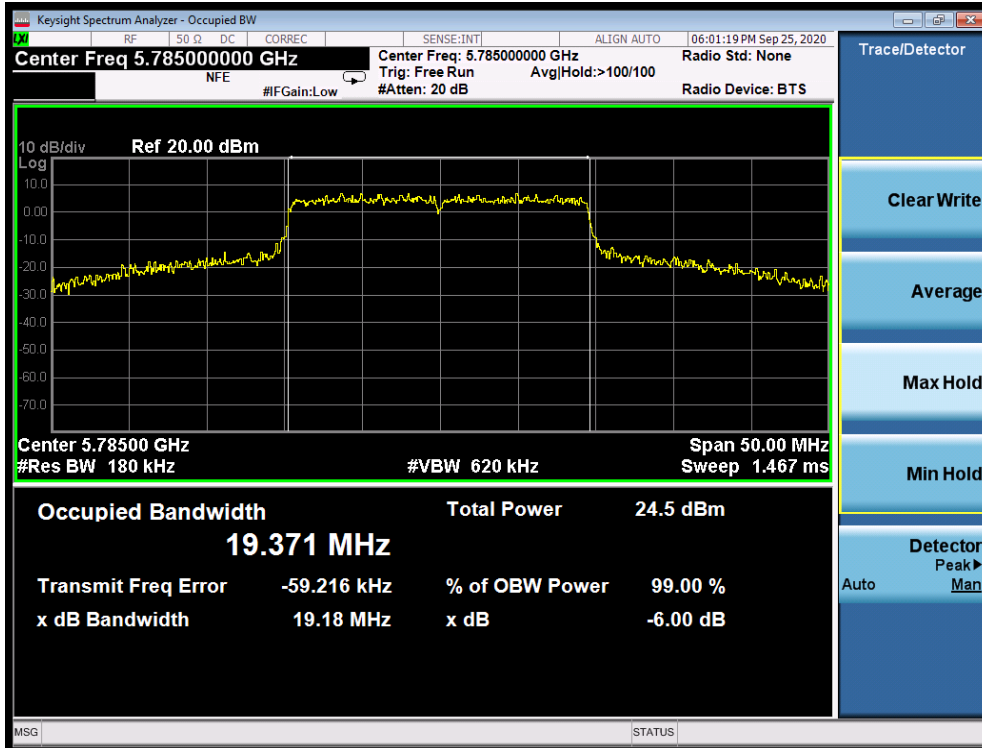
Plot 7-122. 6dB Bandwidth Plot SISO ANT2 (20MHz BW 802.11ax (UNII Band 3) – Ch. 157)
