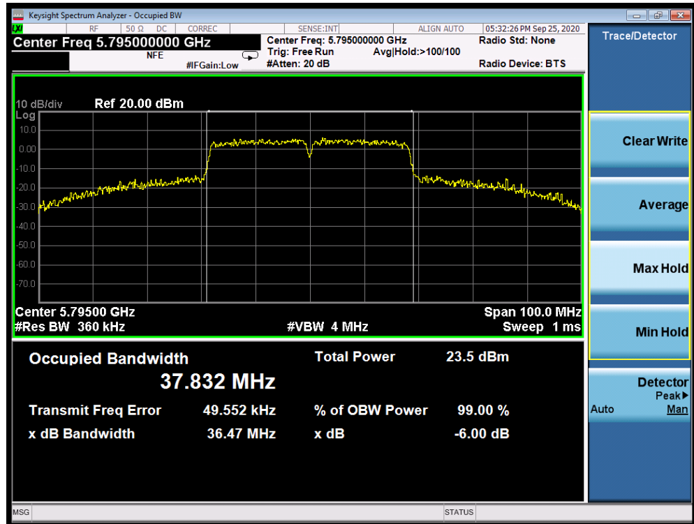
Plot 7-110. 6dB Bandwidth Plot SISO ANT1 (40MHz BW 802.11n (UNII Band 3) – Ch. 159)
