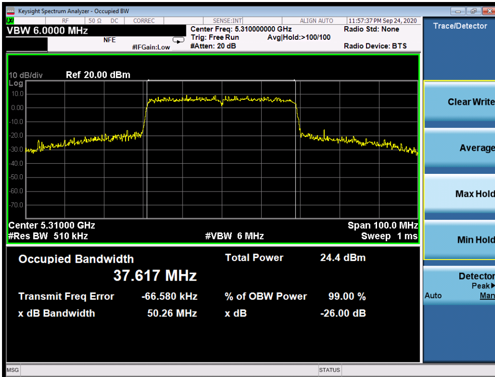
Plot 7-76. 26dB Bandwidth Plot SISO ANT2 (40MHz BW 802.11ax (UNII Band 2a) – Ch. 62)
