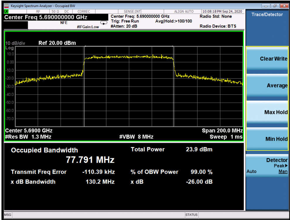
Plot 7-48. 26dB Bandwidth Plot SISO ANT1 (80MHz BW 802.11ax (UNII Band 2C) – Ch. 138)
