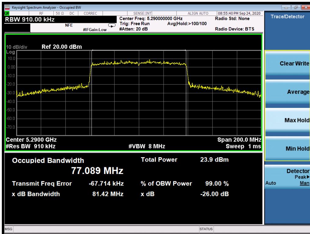
Plot 7-78. 26dB Bandwidth Plot SISO ANT2 (80MHz BW 802.11ax (UNII Band 2A) – Ch. 58)
