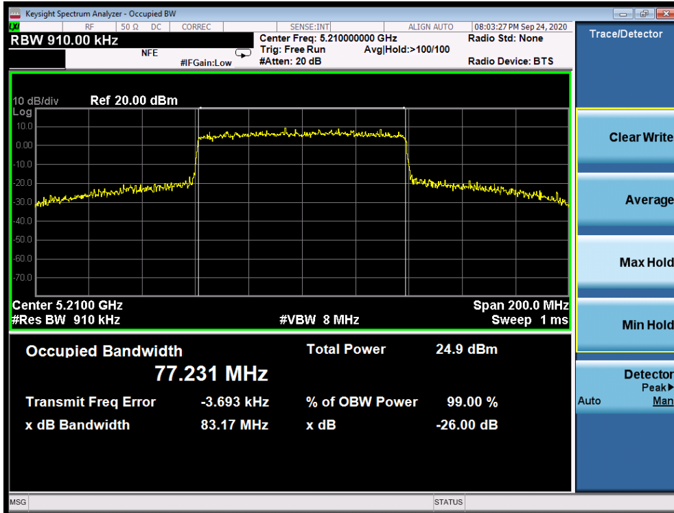
Plot 7-12. 26dB Bandwidth Plot SISO ANT1 (80MHz BW 802.11ax (UNII Band 1) – Ch. 42)
