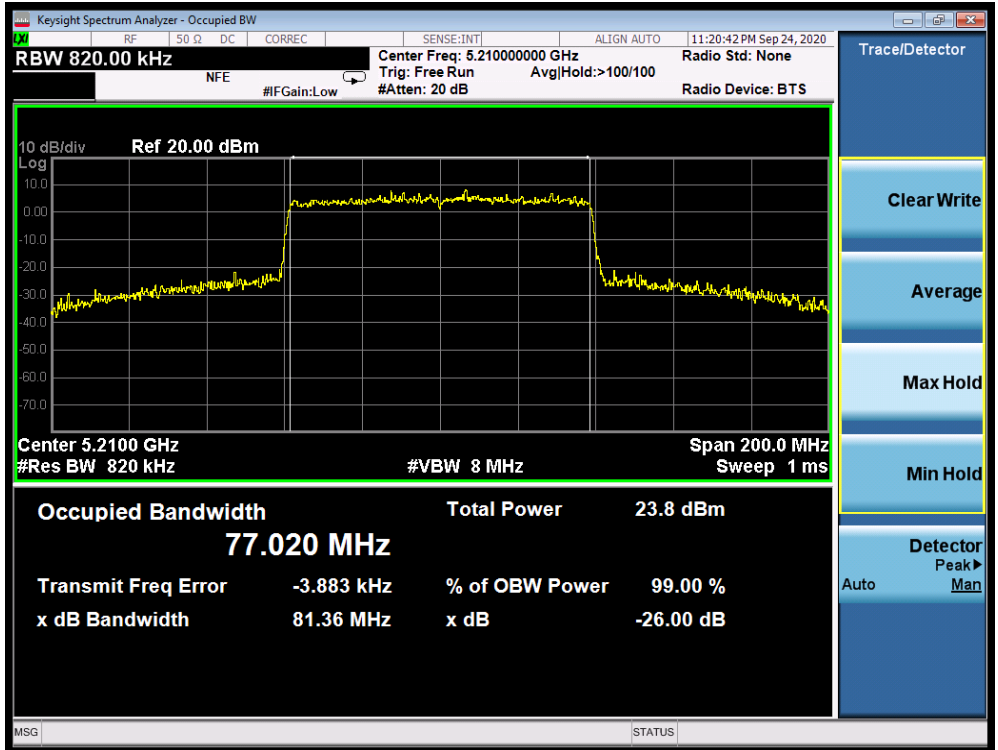
Plot 7-63. 26dB Bandwidth Plot SISO ANT2 (80MHz BW 802.11ax (UNII Band 1) – Ch. 42)
