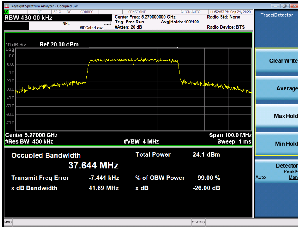
Plot 7-75. 26dB Bandwidth Plot SISO ANT2 (40MHz BW 802.11ax (UNII Band 2a) – Ch. 54)
