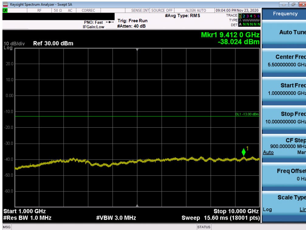
Plot 7-36. Conducted Spurious Plot (LTE Band 14 - 10MHz QPSK - RB Size 1, RB Offset 0)
