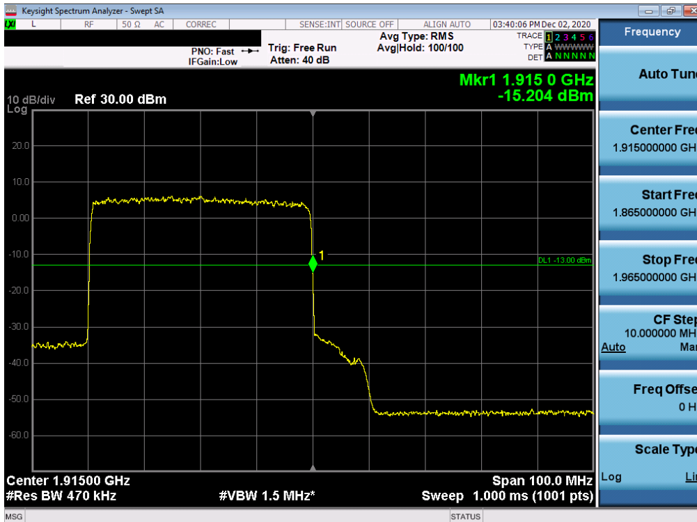
Plot 7-230. Upper Band Edge Plot (NR Band n25 Ant I– 40.0MHz DFT-s-OFDM-QPSK - Full RB)
