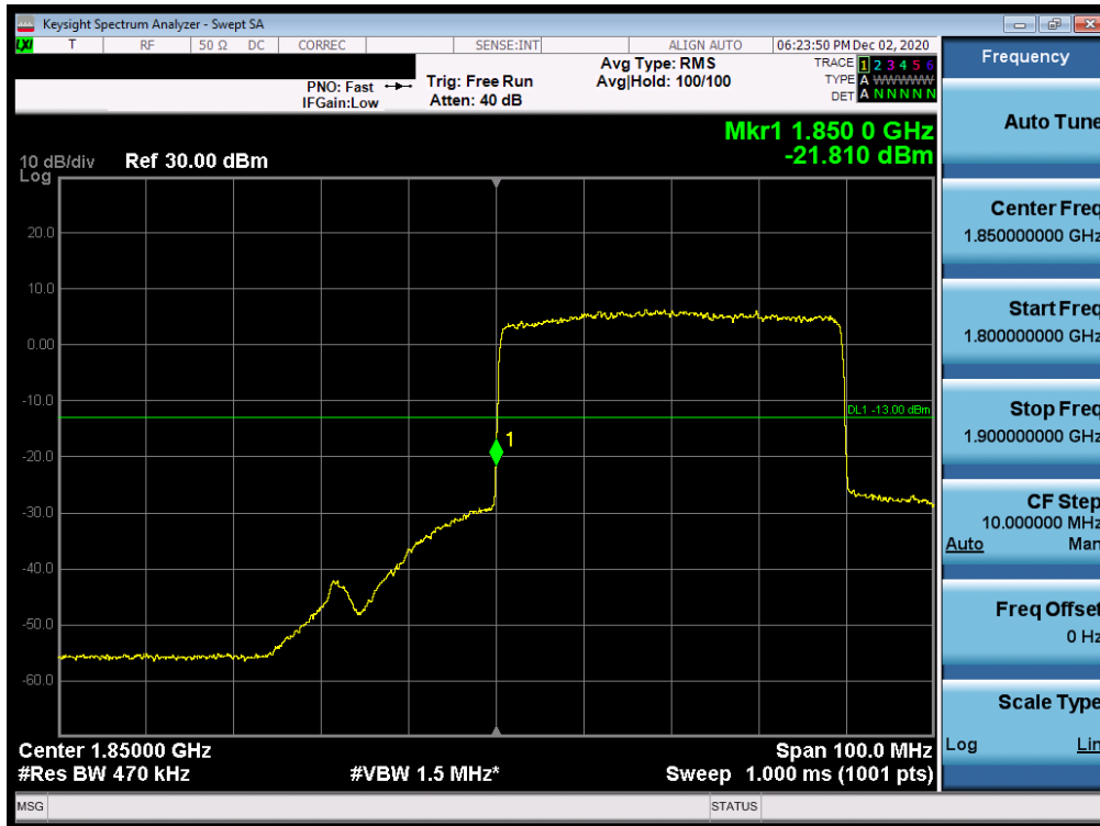
Plot 7-229. Lower Band Edge Plot (NR Band n25 Ant I– 40.0MHz DFT-s-OFDM-QPSK - Full RB)
