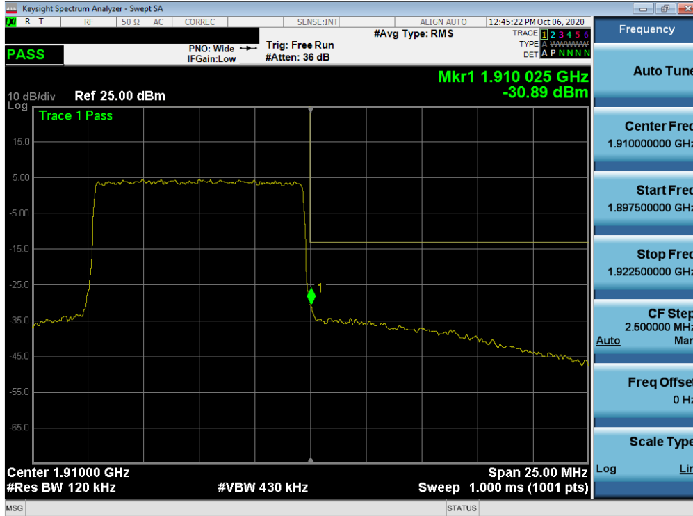
Plot 7-223. Upper Band Edge Plot (NR Band n2 Ant A – 10.0MHz DFT-s-OFDM-QPSK - Full RB)
