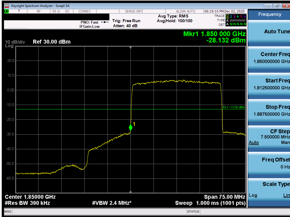
Plot 7-231. Lower Band Edge Plot (NR Band n25 Ant I– 30.0MHz DFT-s-OFDM-QPSK - Full RB)
