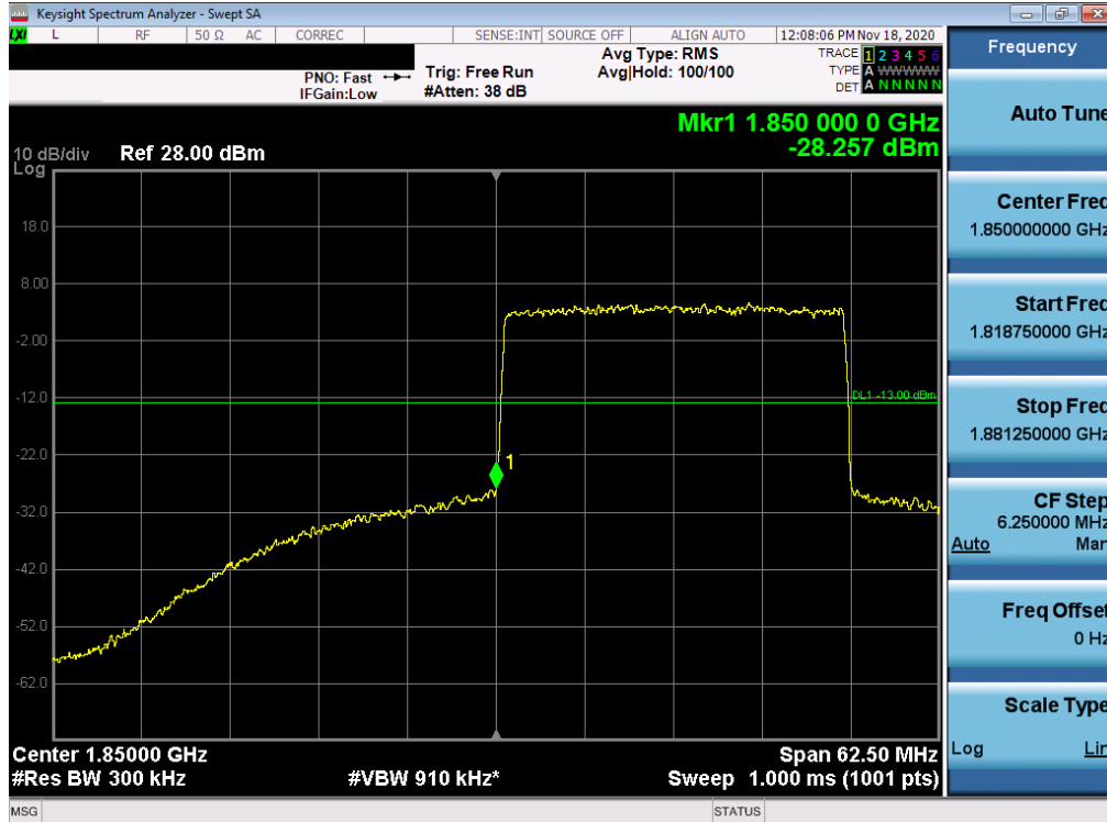
Plot 7-211. Lower Band Edge Plot (NR Band n25 Ant A – 25.0MHz DFT-s-OFDM-QPSK - Full RB)
