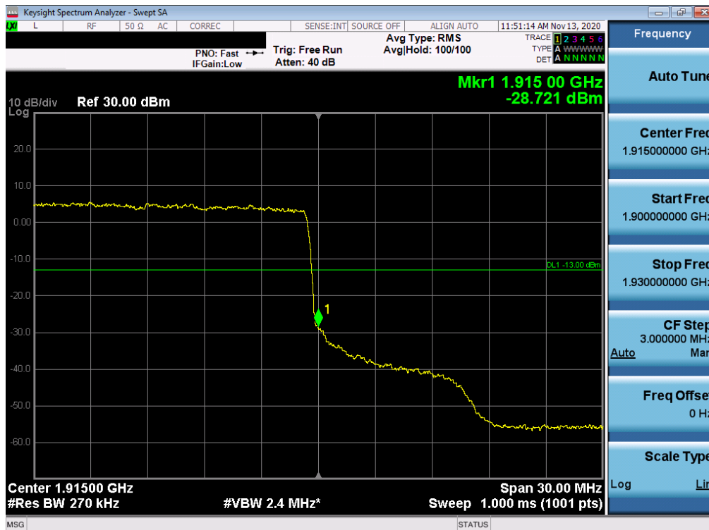
Plot 7-210. Upper Band Edge Plot (NR Band n25 Ant A – 30.0MHz DFT-s-OFDM-QPSK - Full RB)
