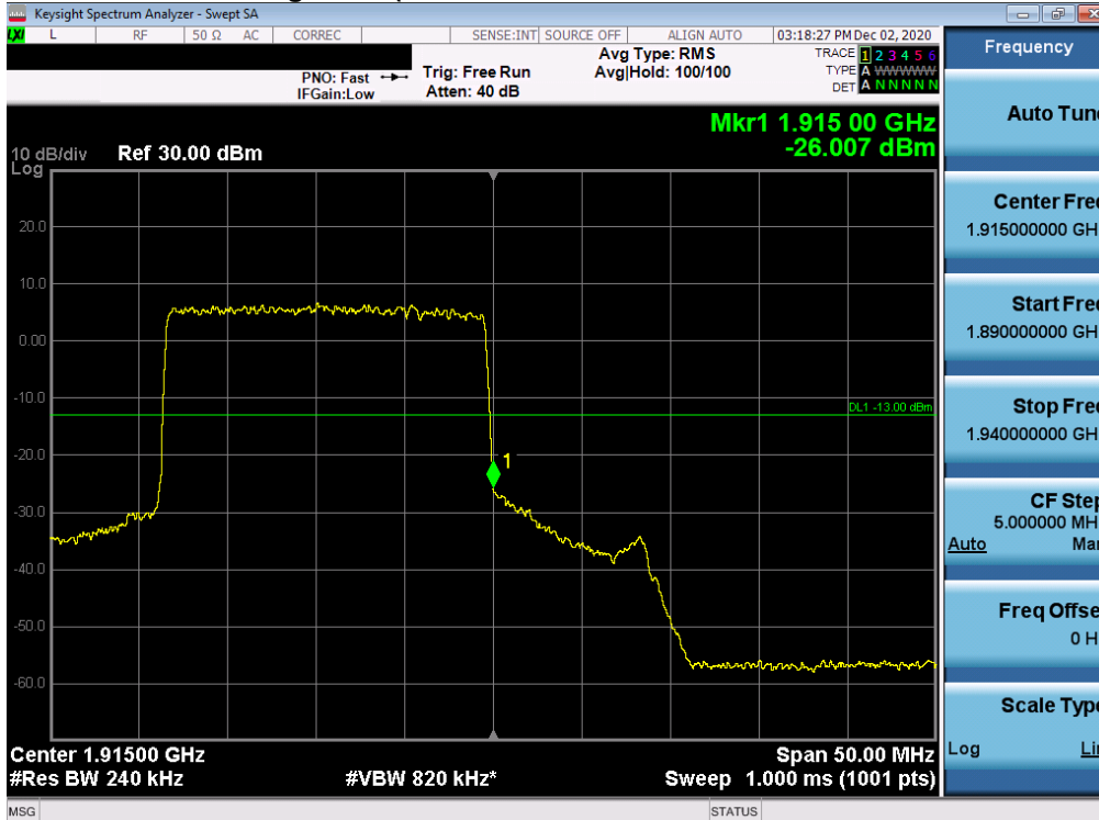
Plot 7-236. Upper Band Edge Plot (NR Band n2 Ant I- 20.0MHz DFT-s-OFDM-QPSK - Full RB)
