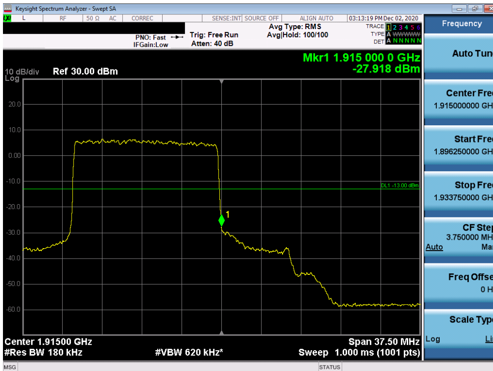
Plot 7-238. Upper Band Edge Plot (NR Band n2 Ant I- 15.0MHz DFT-s-OFDM-QPSK - Full RB)
