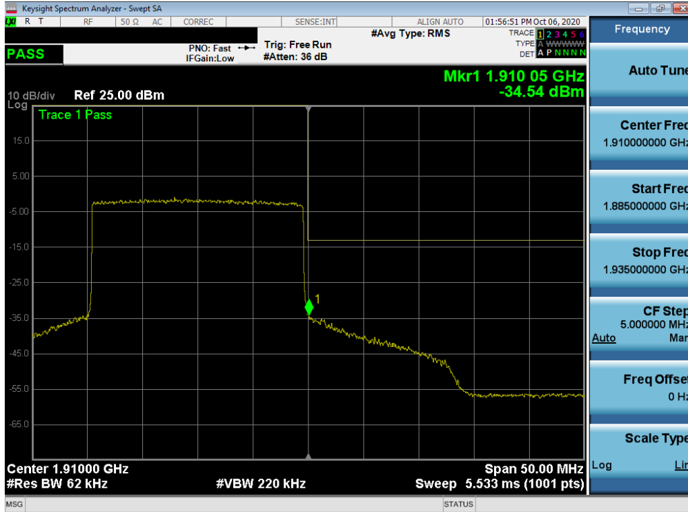
Plot 7-215. Upper Band Edge Plot (NR Band n2 Ant A – 20.0MHz DFT-s-OFDM-QPSK - Full RB)
