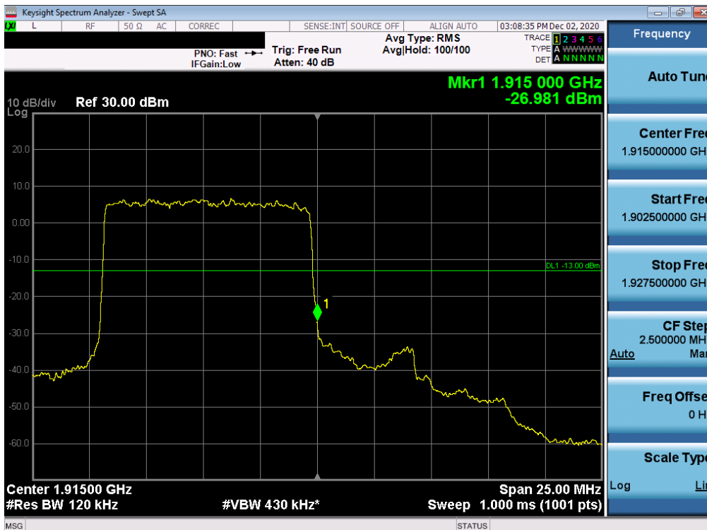
Plot 7-240. Upper Band Edge Plot (NR Band n2 Ant I- 10.0MHz DFT-s-OFDM-QPSK - Full RB)
