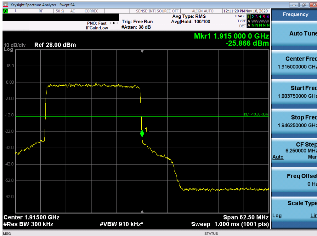
Plot 7-212. Upper Band Edge Plot (NR Band n25 Ant A – 25.0MHz DFT-s-OFDM-QPSK - Full RB)
