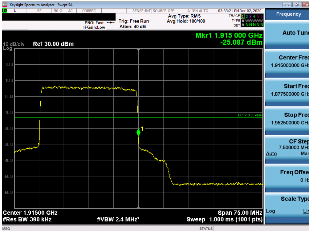
Plot 7-232. Upper Band Edge Plot (NR Band n25 Ant I– 30.0MHz DFT-s-OFDM-QPSK - Full RB)
