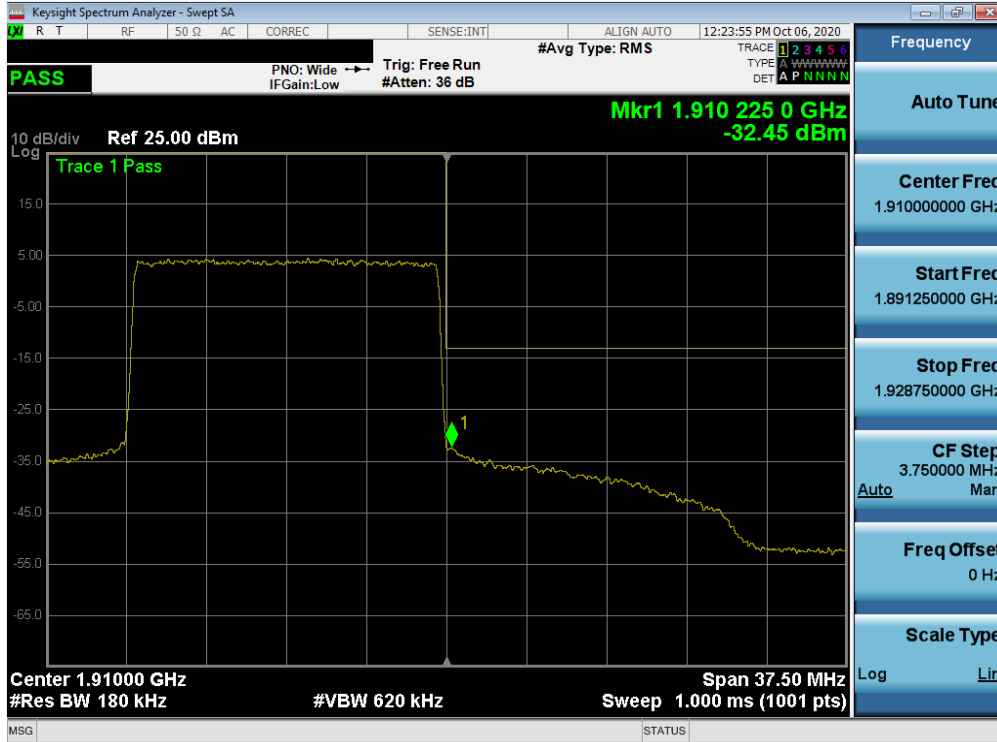
Plot 7-219. Upper Band Edge Plot (NR Band n2 Ant A – 15.0MHz DFT-s-OFDM-QPSK - Full RB)
