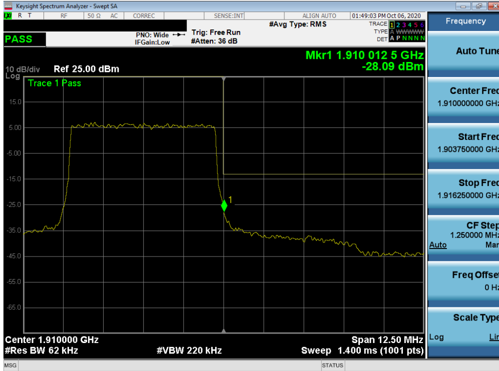
Plot 7-227. Upper Band Edge Plot (NR Band n2 Ant A – 5.0MHz DFT-s-OFDM-QPSK - Full RB)
