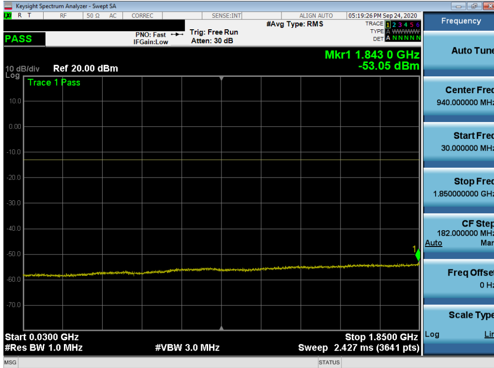
Plot 7-123. Conducted Spurious Plot (NR Band n2 Ant A - 20.0MHz - RB Size 1, RB Offset 0 - High Channel)
