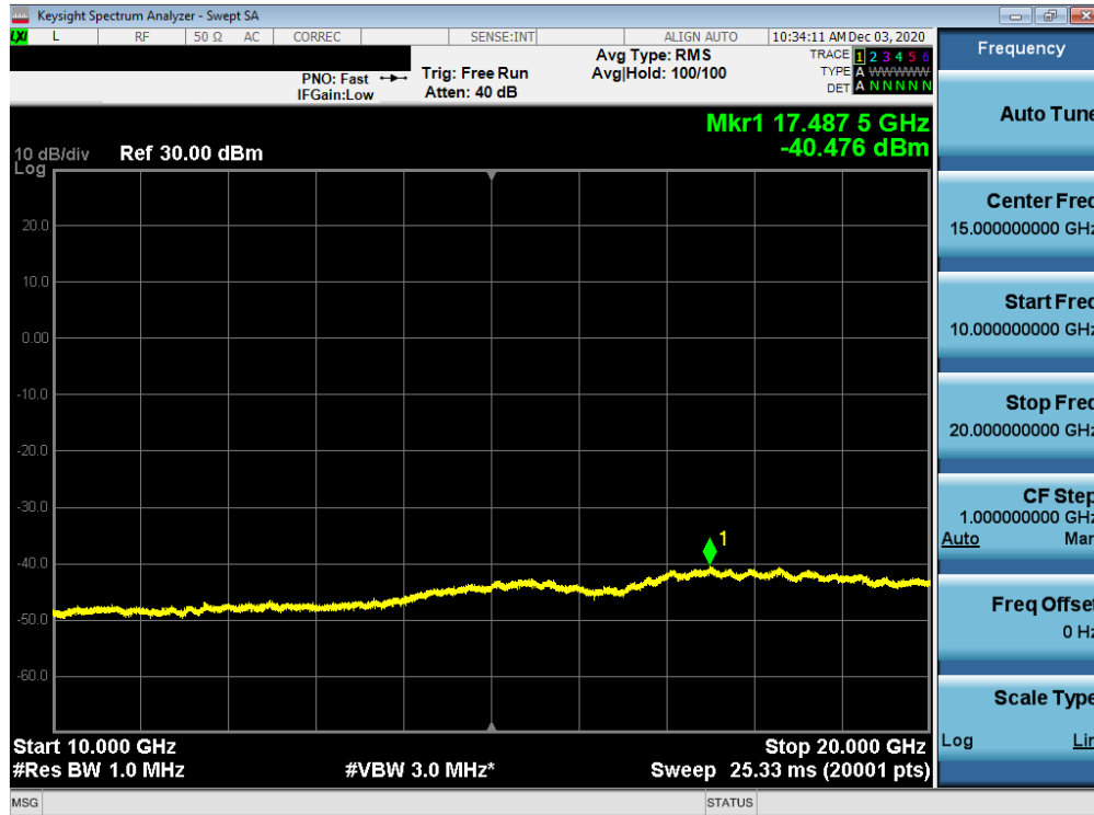
Plot 7-137. Conducted Spurious Plot (NR Band n2 Ant I- 20.0MHz - RB Size 1, RB Offset 0 - Low Channel)
