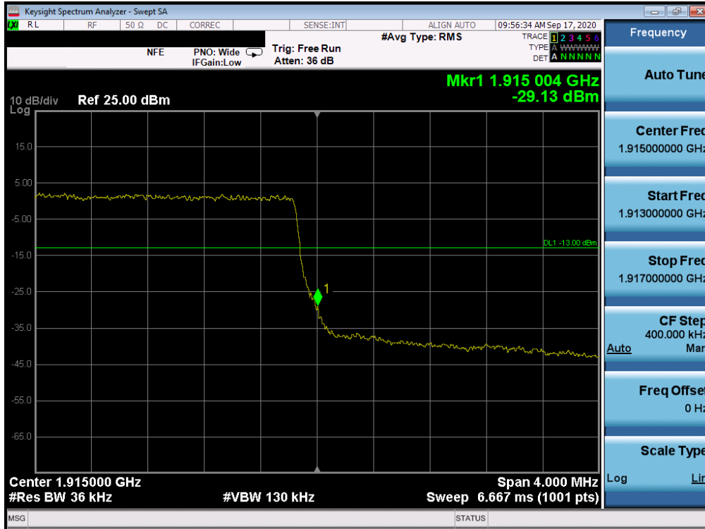
Plot 7-199. Upper Band Edge Plot (LTE Band 25 - 3MHz QPSK – Full RB Configuration)
