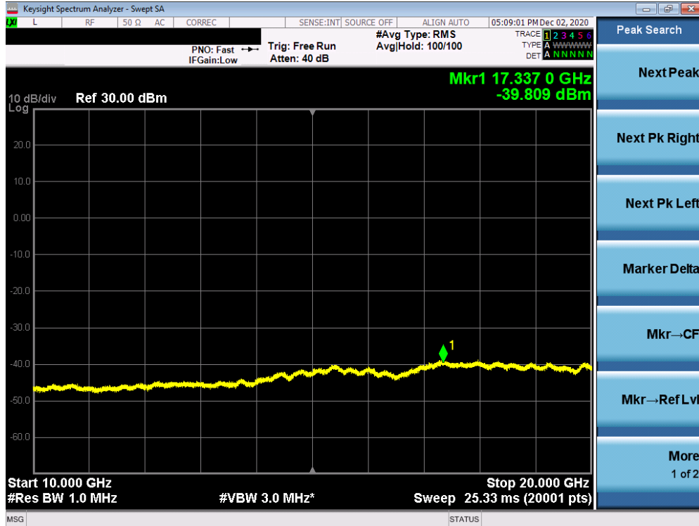
Plot 7-110. Conducted Spurious Plot (NR Band n25 Ant A- 40.0MHz - RB Size 1, RB Offset 0 - Low Channel)
