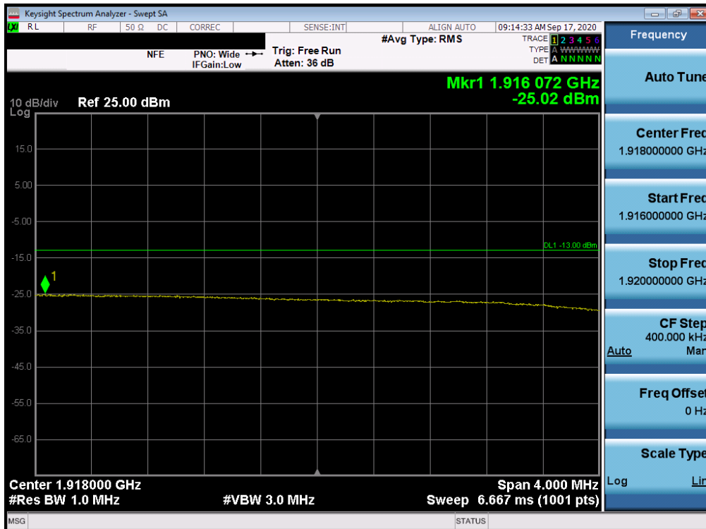
Plot 7-182. Extended Upper Band Edge Plot (LTE Band 25 - 15MHz QPSK – Full RB Configuration)
