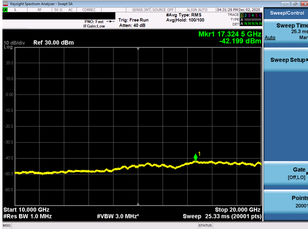
Plot 7-134. Conducted Spurious Plot (NR Band n25 Ant I- 40.0MHz - RB Size 1, RB Offset 0 - High Channel)
