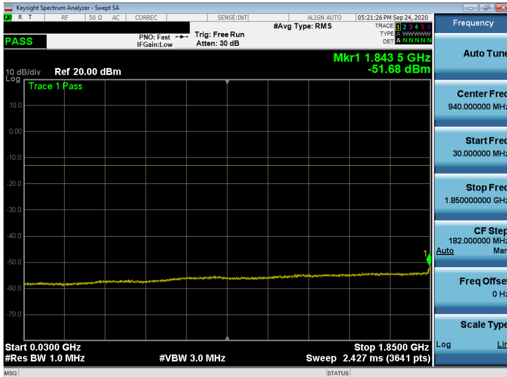
Plot 7-120. Conducted Spurious Plot (NR Band n2 Ant A - 20.0MHz - RB Size 1, RB Offset 0 - Mid Channel)
