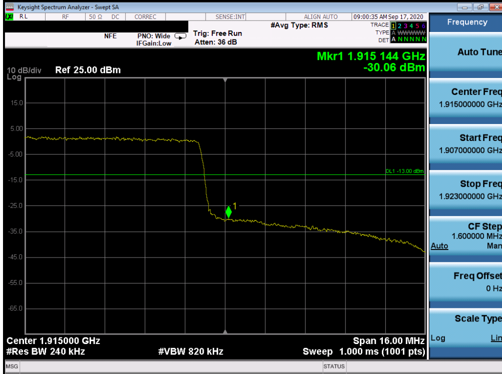
Plot 7-175. Upper Band Edge Plot (LTE Band 25 - 20MHz QPSK – Full RB Configuration)
