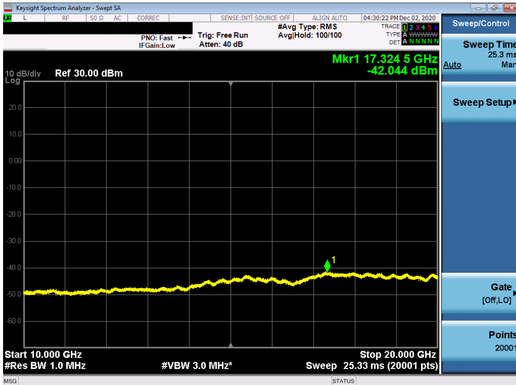
Plot 7-131. Conducted Spurious Plot (NR Band n25 Ant I- 40.0MHz - RB Size 1, RB Offset 0 - Mid Channel)
