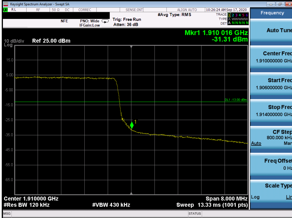
Plot 7-185. Upper Band Edge Plot (LTE Band 2 - 10MHz QPSK – Full RB Configuration)
