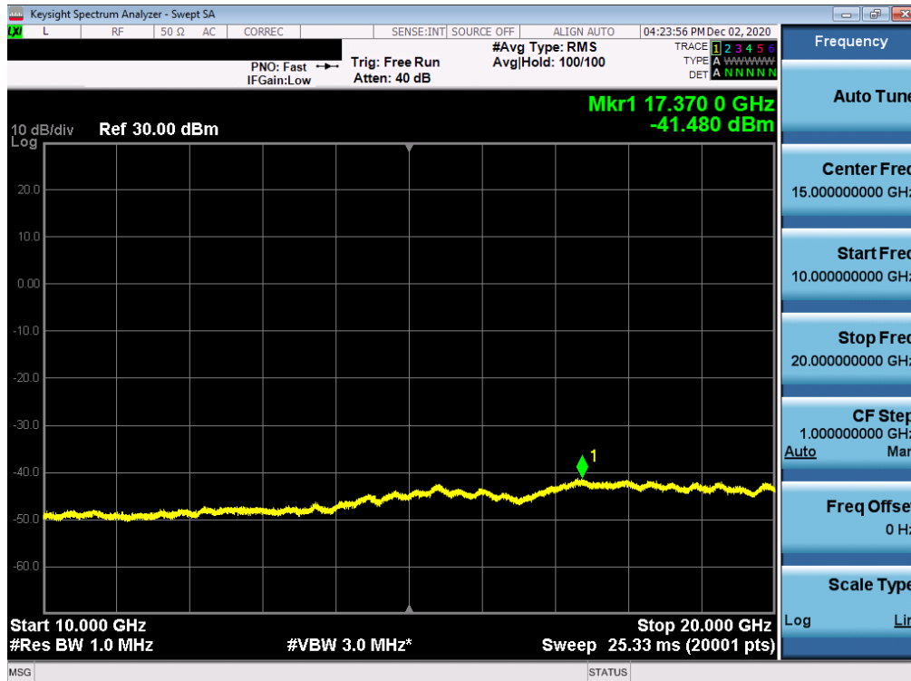
Plot 7-128. Conducted Spurious Plot (NR Band n25 Ant I- 40.0MHz - RB Size 1, RB Offset 0 - Low Channel)
