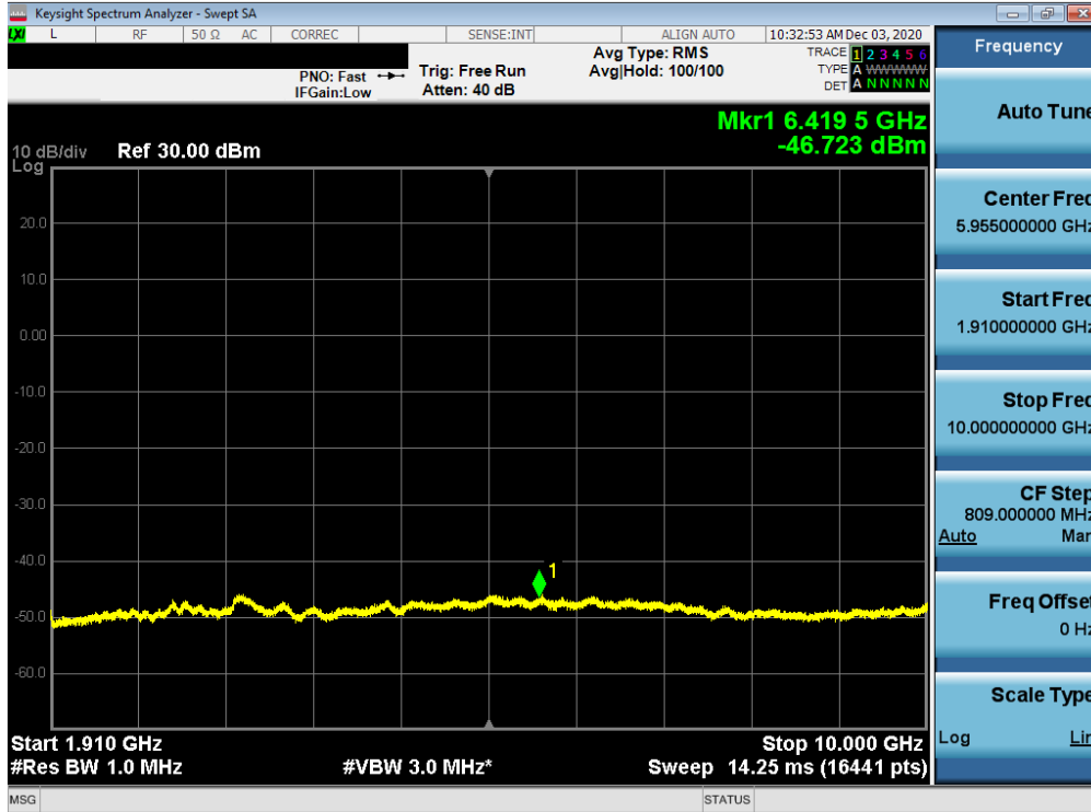
Plot 7-139. Conducted Spurious Plot (NR Band n2 Ant I- 20.0MHz - RB Size 1, RB Offset 0 - Mid Channel)
