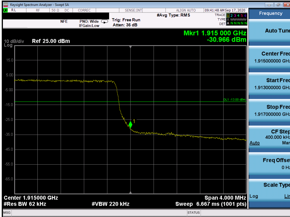
Plot 7-193. Upper Band Edge Plot (LTE Band 25 - 5MHz QPSK – Full RB Configuration)
