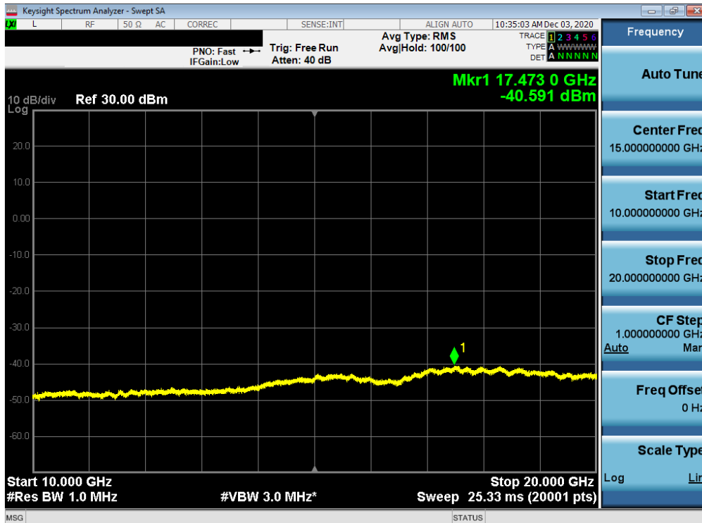
Plot 7-140. Conducted Spurious Plot (NR Band n2 Ant I- 20.0MHz - RB Size 1, RB Offset 0 - Mid Channel)
