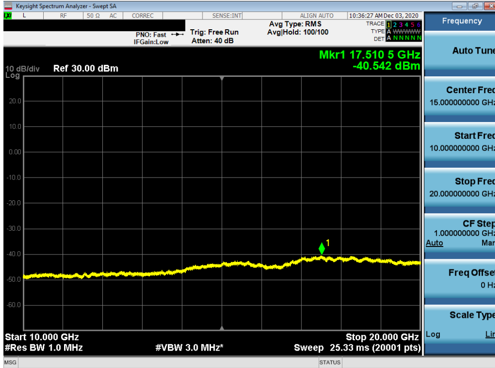
Plot 7-143. Conducted Spurious Plot (NR Band n2 Ant I- 20.0MHz - RB Size 1, RB Offset 0 - High Channel)
