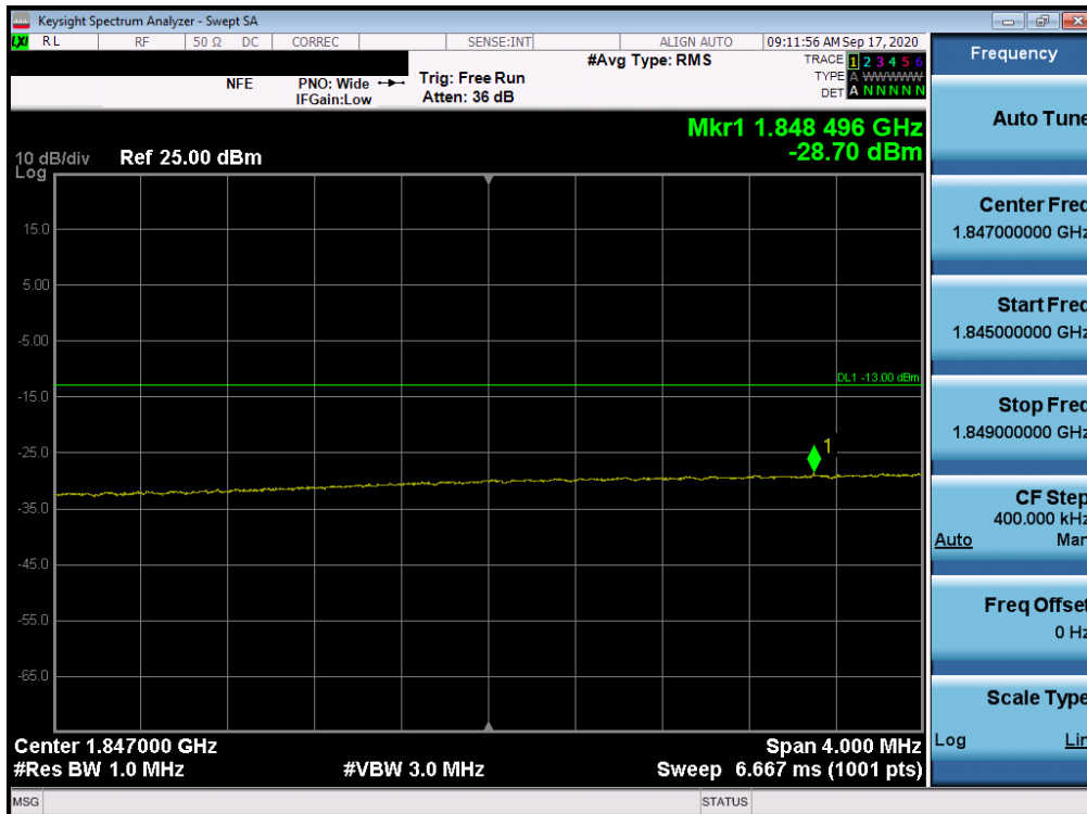
Plot 7-178. Extended Lower Band Edge Plot (LTE Band 25/2 - 15MHz QPSK – Full RB Configuration)
