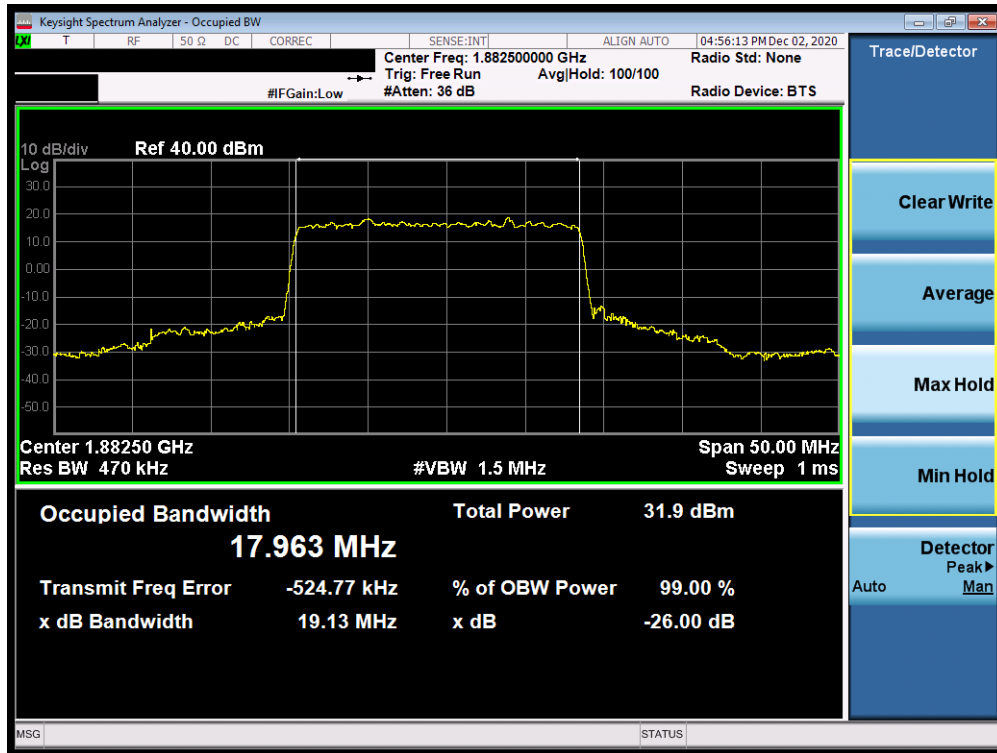
Plot 7-75. Occupied Bandwidth Plot (NR Band n2 Ant I- 20.0MHz DFT-s-OFDM BPSK - Full RB)
