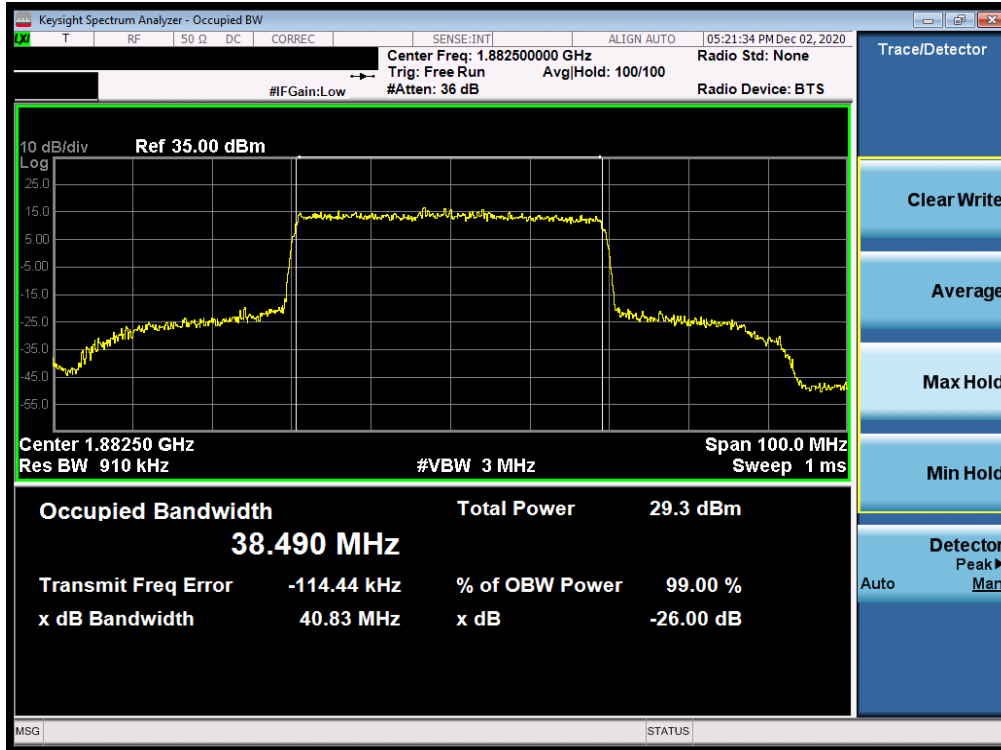
Plot 7-62. Occupied Bandwidth Plot (NR Band n25 Ant I- 40.0MHz CP-OFDM 16QAM - Full RB)
