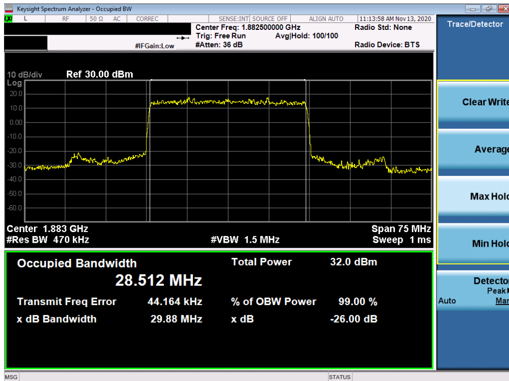
Plot 7-30. Occupied Bandwidth Plot (NR Band n25 Ant A - 30.0MHz DFT-s-OFDM BPSK - Full RB)
