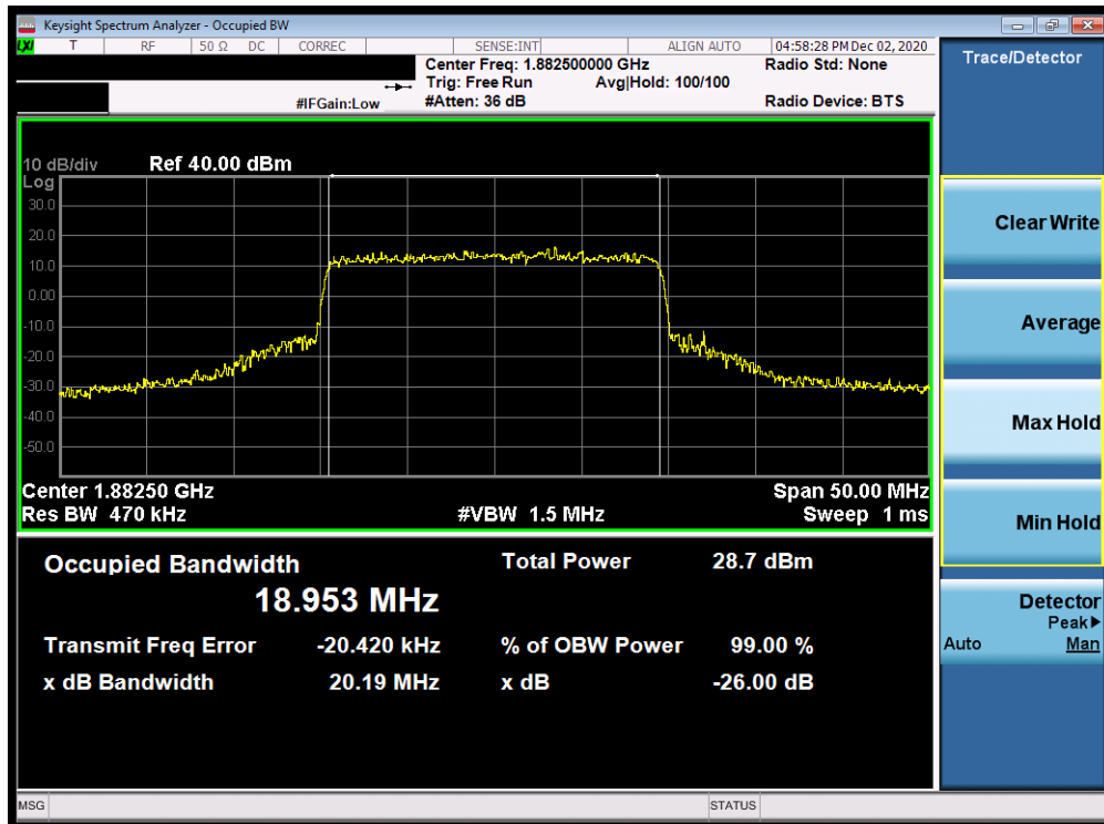
Plot 7-76. Occupied Bandwidth Plot (NR Band n2 Ant I- 20.0MHz CP-OFDM QPSK - Full RB)
