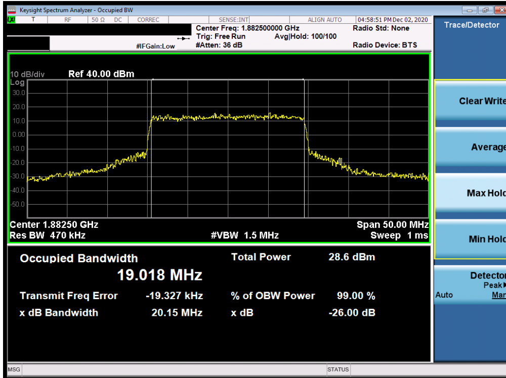
Plot 7-77. Occupied Bandwidth Plot (NR Band n2 Ant I- 20.0MHz CP-OFDM 16QAM - Full RB)
