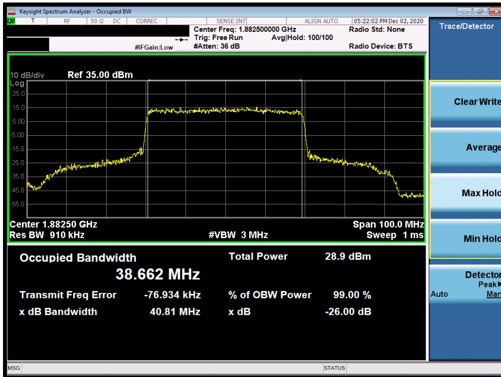
Plot 7-63. Occupied Bandwidth Plot (NR Band n25 Ant I- 40.0MHz CP-OFDM 64QAM - Full RB)
