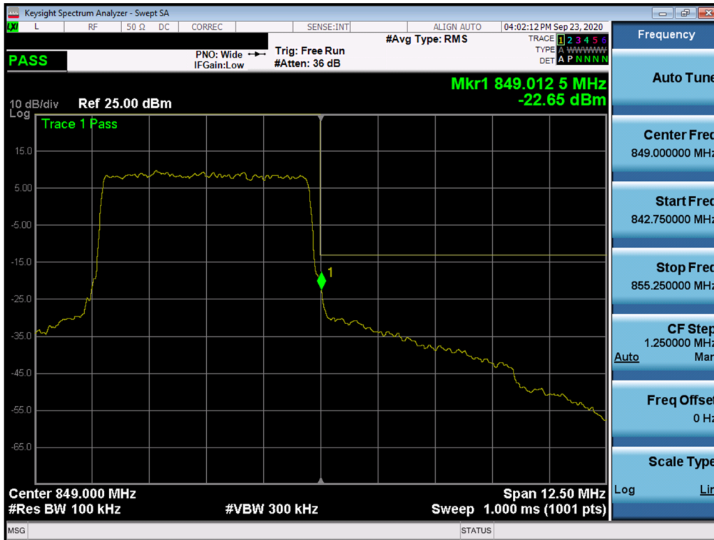
Plot 7-88. Upper Band Edge Plot (NR Band n5 – 5.0MHz - Full RB)
