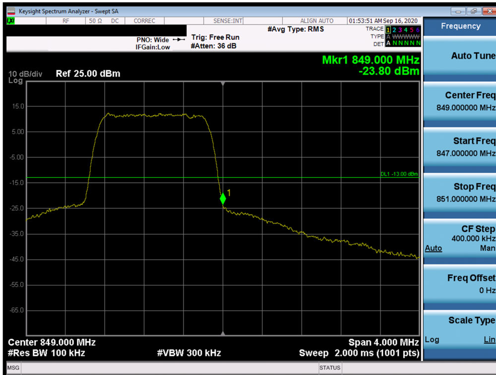
Plot 7-80. Upper Band Edge Plot (LTE Band 26/5 – 1.4MHz QPSK – Full RB Configuration)
