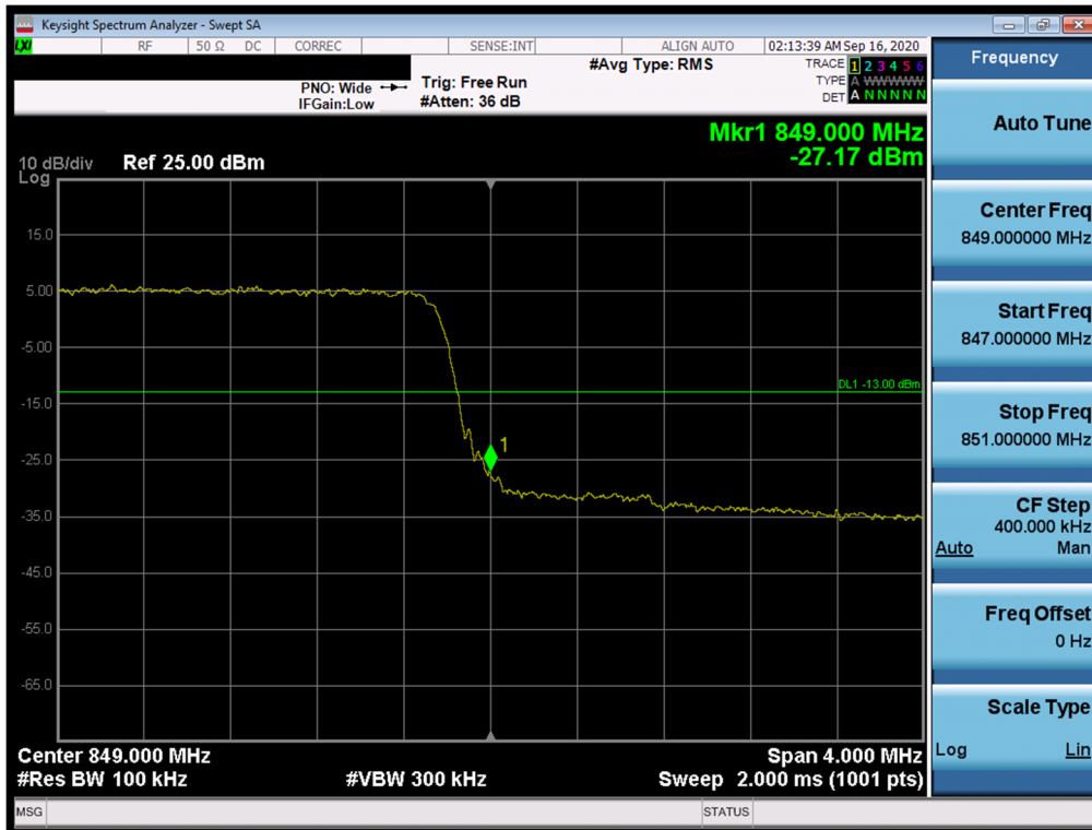
Plot 7-76. Upper Band Edge Plot (LTE Band 26/5 - 5MHz QPSK – Full RB Configuration)
