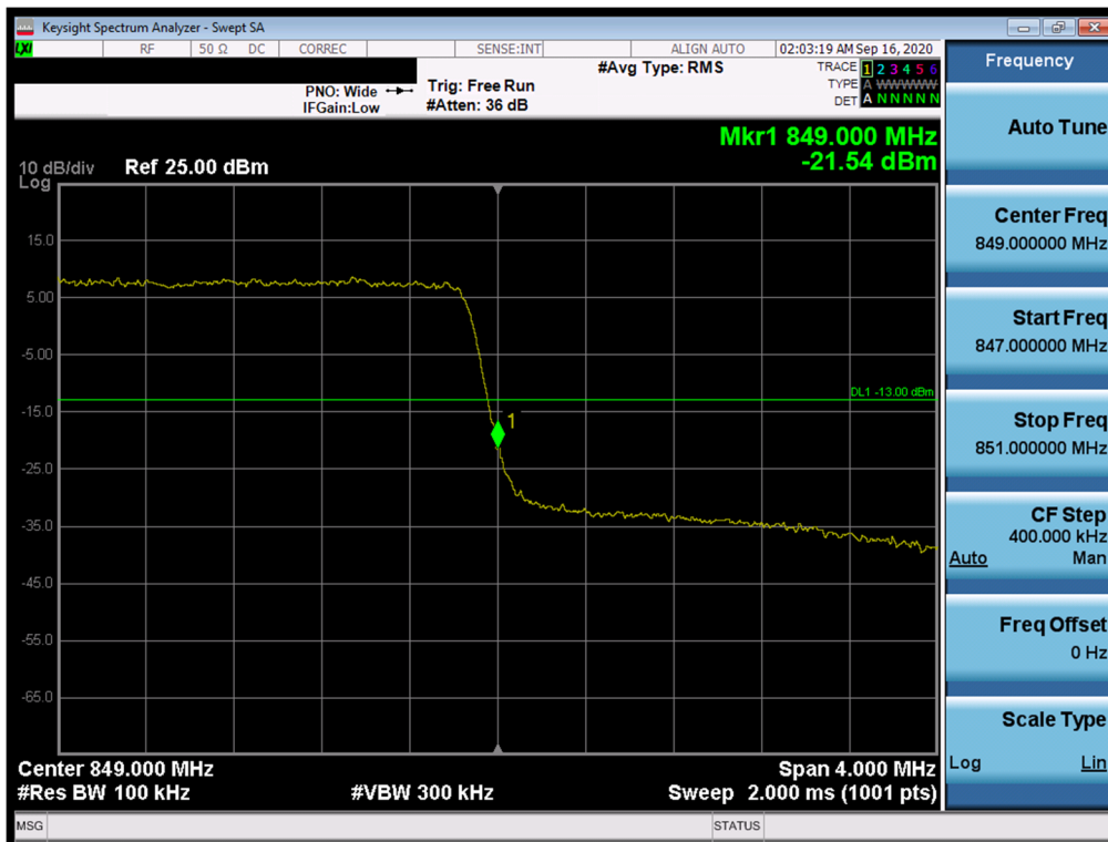
Plot 7-78. Upper Band Edge Plot (LTE Band 26/5 - 3MHz QPSK – Full RB Configuration)
