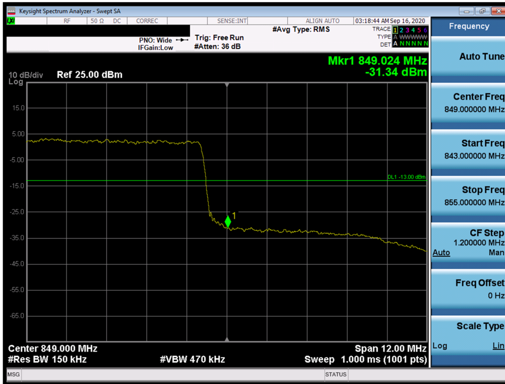
Plot 7-72. Upper Band Edge Plot (LTE Band 26 - 15MHz QPSK – Full RB Configuration)
