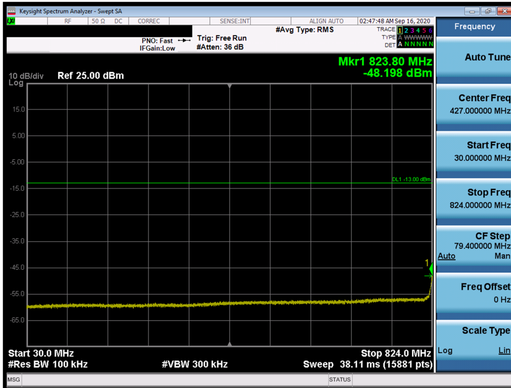
Plot 7-51. Conducted Spurious Plot (LTE Band 26/5 - 10MHz QPSK - RB Size 1, RB Offset 0 - High Channel)
