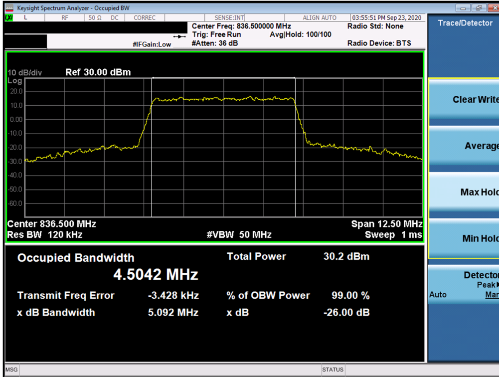
Plot 7-37. Occupied Bandwidth Plot (NR Band n5 - 5MHz QPSK - Full RB Configuration)
