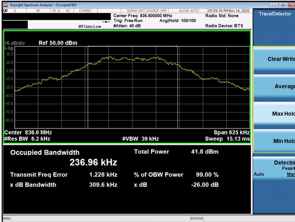
Plot 7-42. Occupied Bandwidth Plot (EDGE, Ch. 190)
