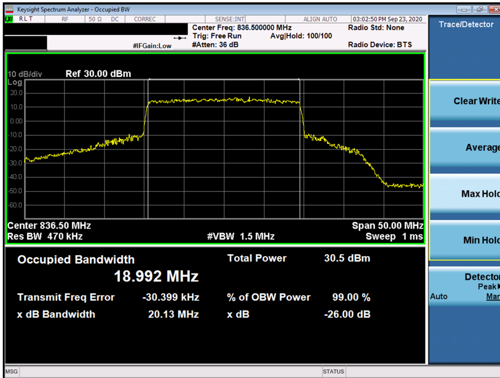
Plot 7-24. Occupied Bandwidth Plot (NR Band n5 - 20MHz 64-QAM - Full RB Configuration)
