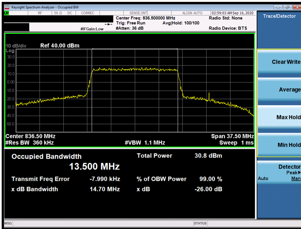
Plot 7-2. Occupied Bandwidth Plot (LTE Band 26 - 15MHz 16-QAM - Full RB Configuration)
