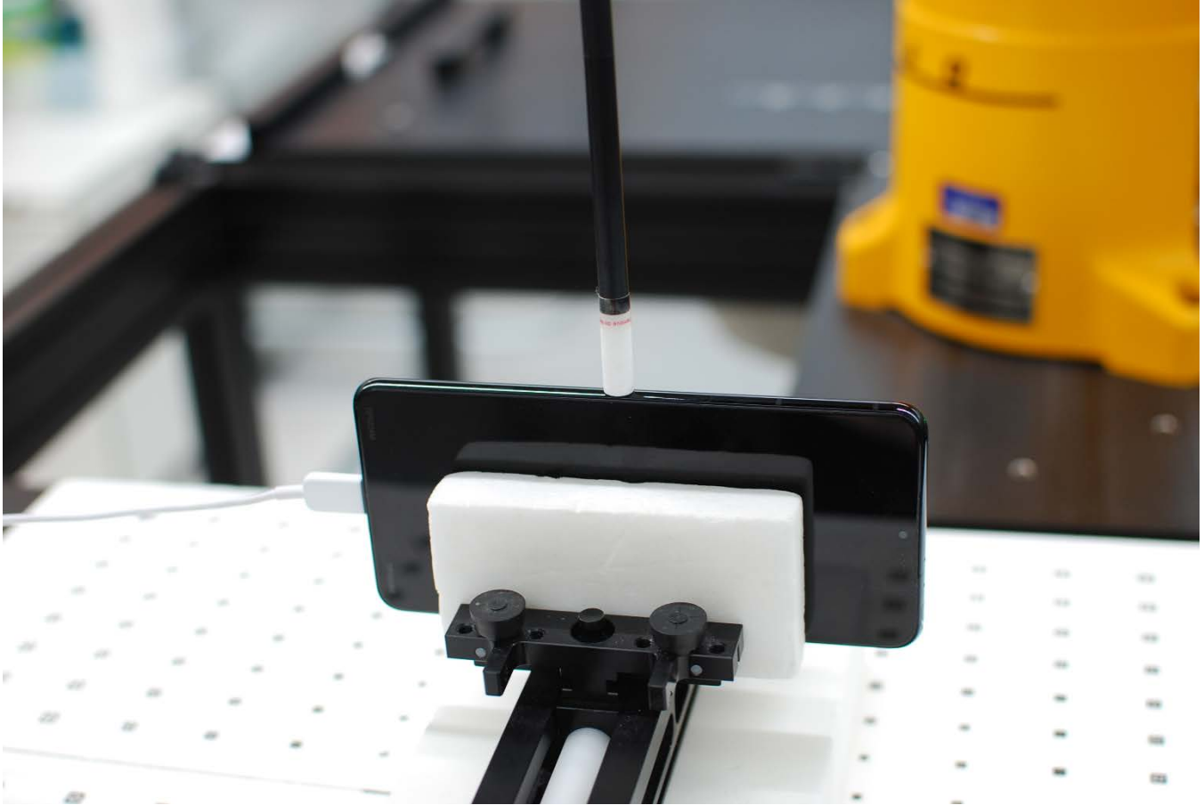
Figure D-4 Near Field Power Density Test Setup Photo – Left Edge at 2 mm
