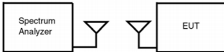
Figure 7-2. Test Instrument and Measurement Setup
