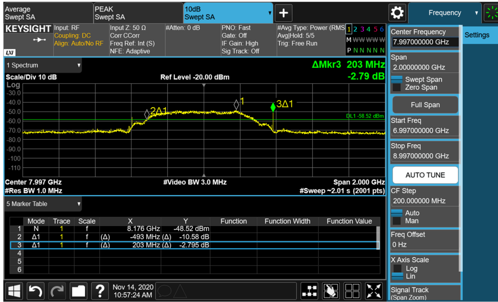
Plot 7-85. BANDWIDTH Plot – ANT1 - CH.9 - SP0 – Preamble 11
