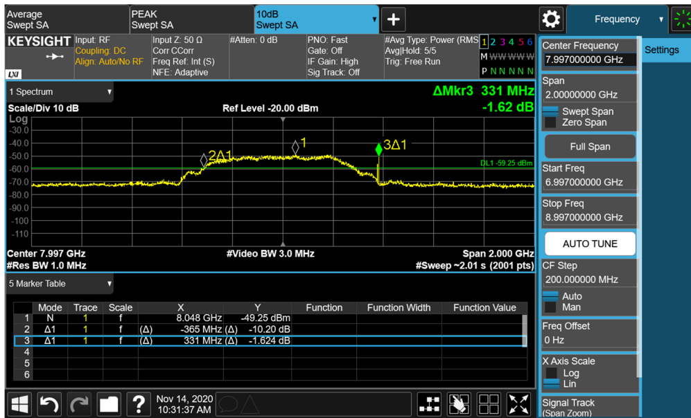
Plot 7-84. BANDWIDTH Plot – ANT2 - CH.9 – SP3 – Preamble 10
