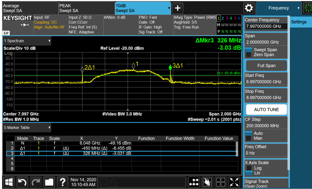
Plot 7-81. BANDWIDTH Plot – ANT1 - CH.9 – SP3 – Preamble 10
