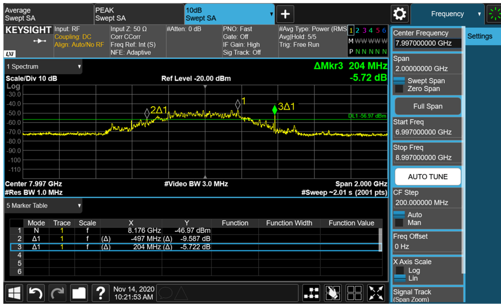
Plot 7-82. BANDWIDTH Plot – ANT2 - CH.9 - SP0 – Preamble 10
