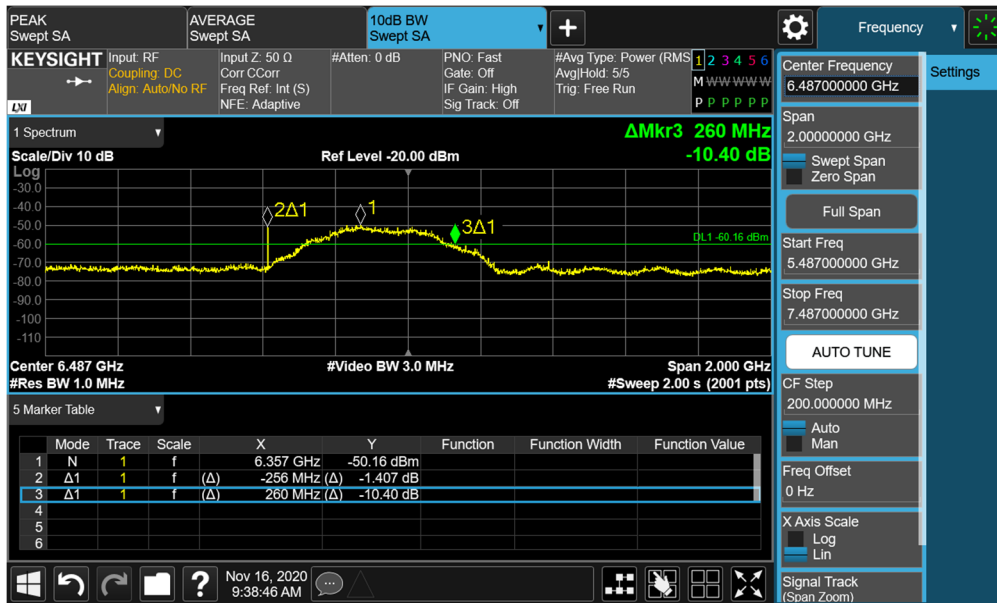
Plot 7-34. BANDWIDTH Plot – ANT2 - CH.5 - SP0 – Preamble 26
