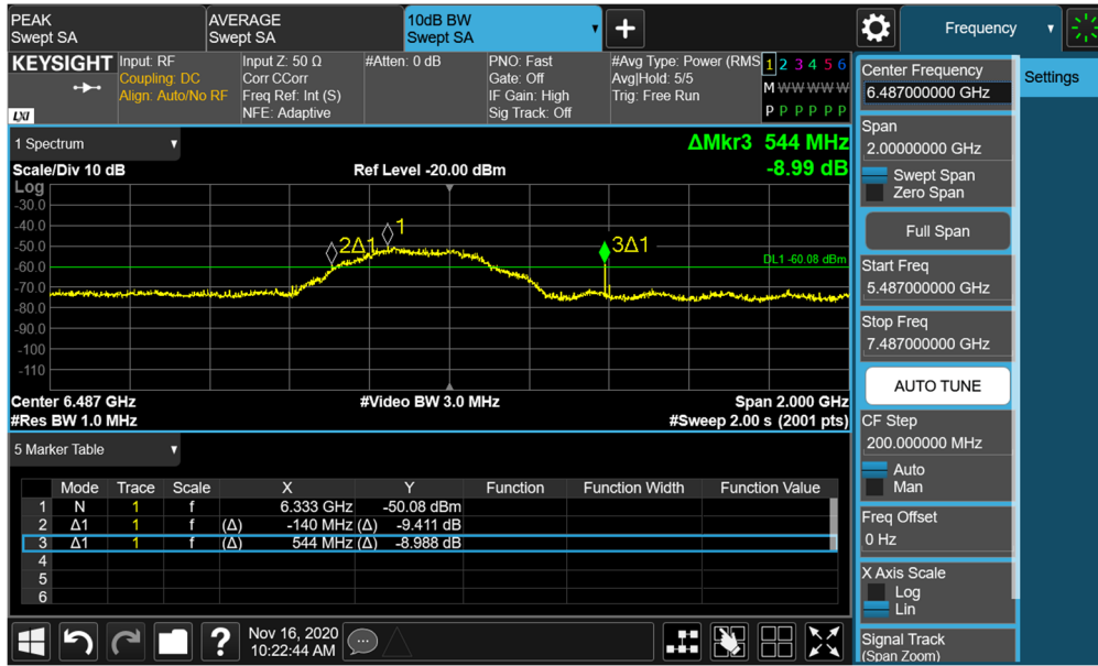
Plot 7-51. BANDWIDTH Plot – ANT1 - CH.5 – SP3 – Preamble 29
