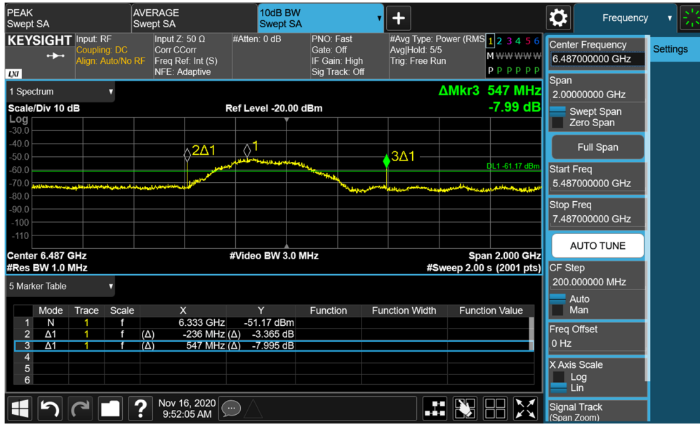
Plot 7-39. BANDWIDTH Plot – ANT1 - CH.5 – SP3 – Preamble 27
