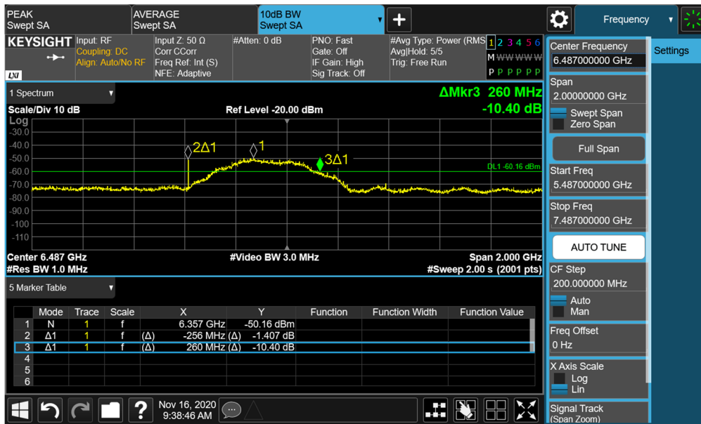
Plot 7-36. BANDWIDTH Plot – ANT2 - CH.5 – SP3 – Preamble 26
