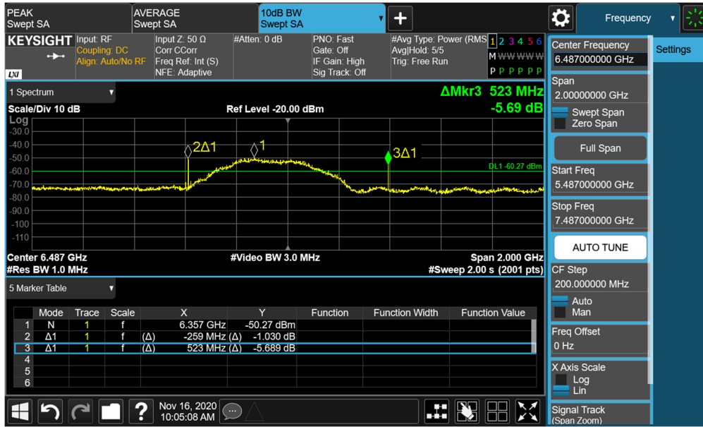
Plot 7-47. BANDWIDTH Plot – ANT2 - CH.5 – SP1 – Preamble 28
