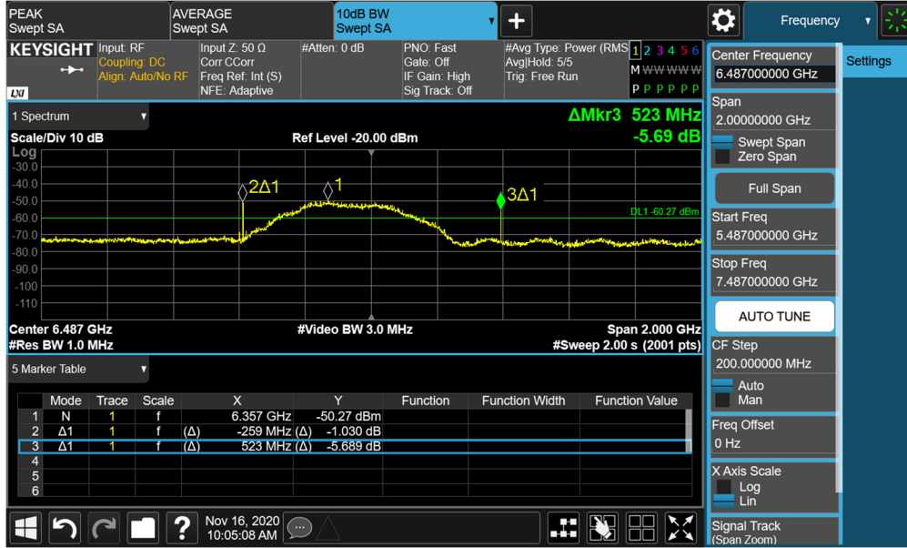
Plot 7-45. BANDWIDTH Plot – ANT1 - CH.5 – SP3 – Preamble 28
