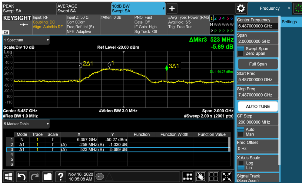
Plot 7-44. BANDWIDTH Plot – ANT1 - CH.5 – SP1 – Preamble 28
