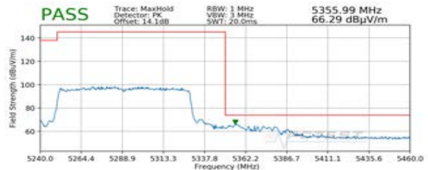
Plot 7-434. Radiated Upper Band Edge Plot MIMO (Peak – UNII Band 2A – 996 Tones)
