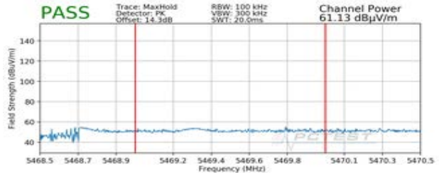
Plot 7-436. Radiated Lower Band Edge Plot MIMO (Peak – UNII Band 2C – 996 Tones)
