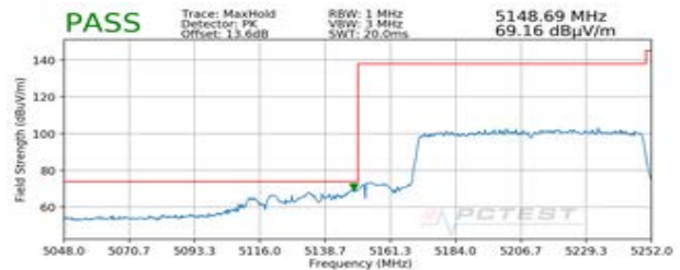
Plot 7-411. Radiated Lower Band Edge Plot SISO ANT2 (Peak – UNII Band 1 – 996 Tones)
