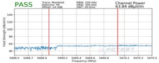
Plot 7-429. Radiated Lower Band Edge Plot MIMO (Peak – UNII Band 2C – 484 Tones)
