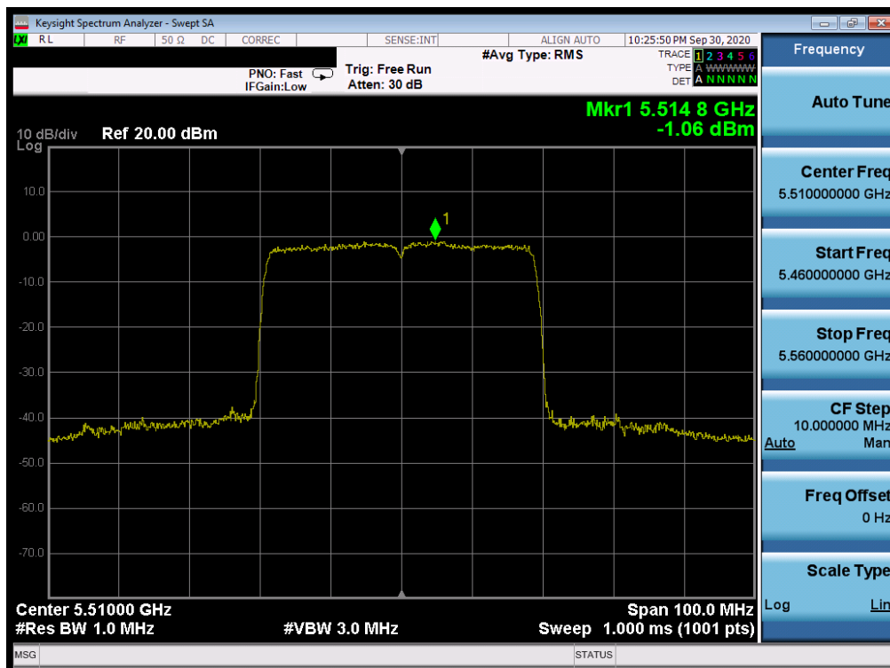
Plot 7-313. Power Spectral Density Plot MIMO ANT2 (40MHz BW 802.11ax – Full Tones (UNII Band 2C) – Ch. 102)
