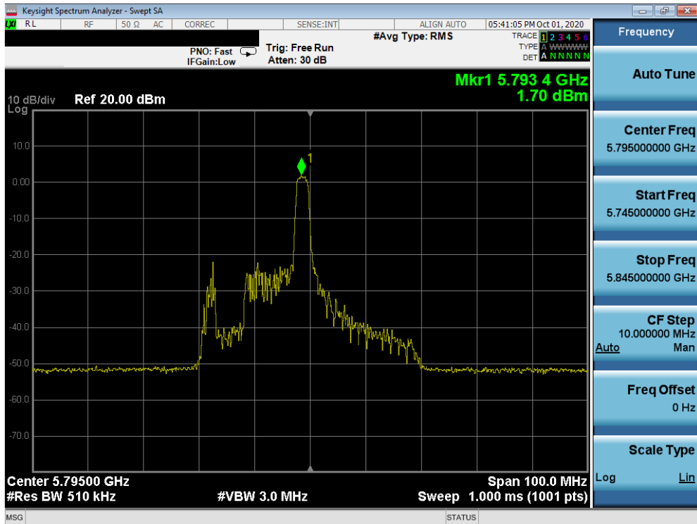
Plot 7-296. Power Spectral Density Plot MIMO ANT2 (40MHz BW 802.11ax – 26 Tones (UNII Band 3) – Ch. 159)
