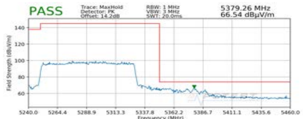
Plot 7-385. Radiated Upper Band Edge Plot SISO ANT1 (Peak – UNII Band 2A – 996 Tones)
