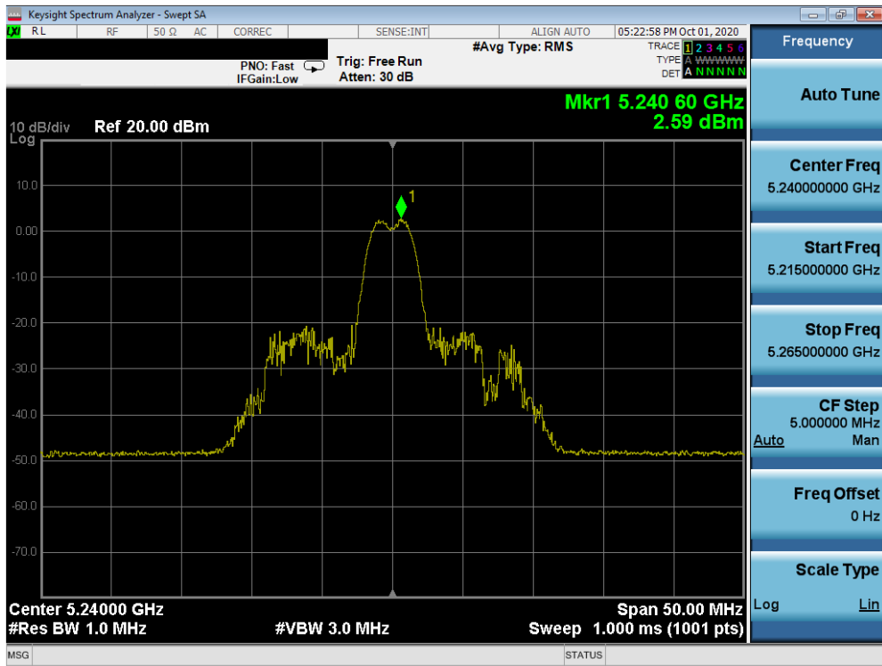
Plot 7-273. Power Spectral Density Plot MIMO ANT2 (20MHz BW 802.11ax – 26 Tones (UNII Band 1) – Ch. 48)
