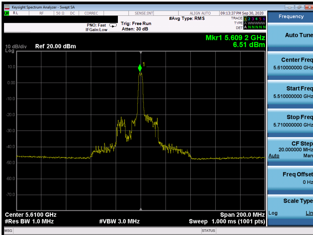
Plot 7-182. Power Spectral Density Plot SISO ANT2 (80MHz BW 802.11ax – 26 Tones (UNII Band 2C) – Ch. 122)
