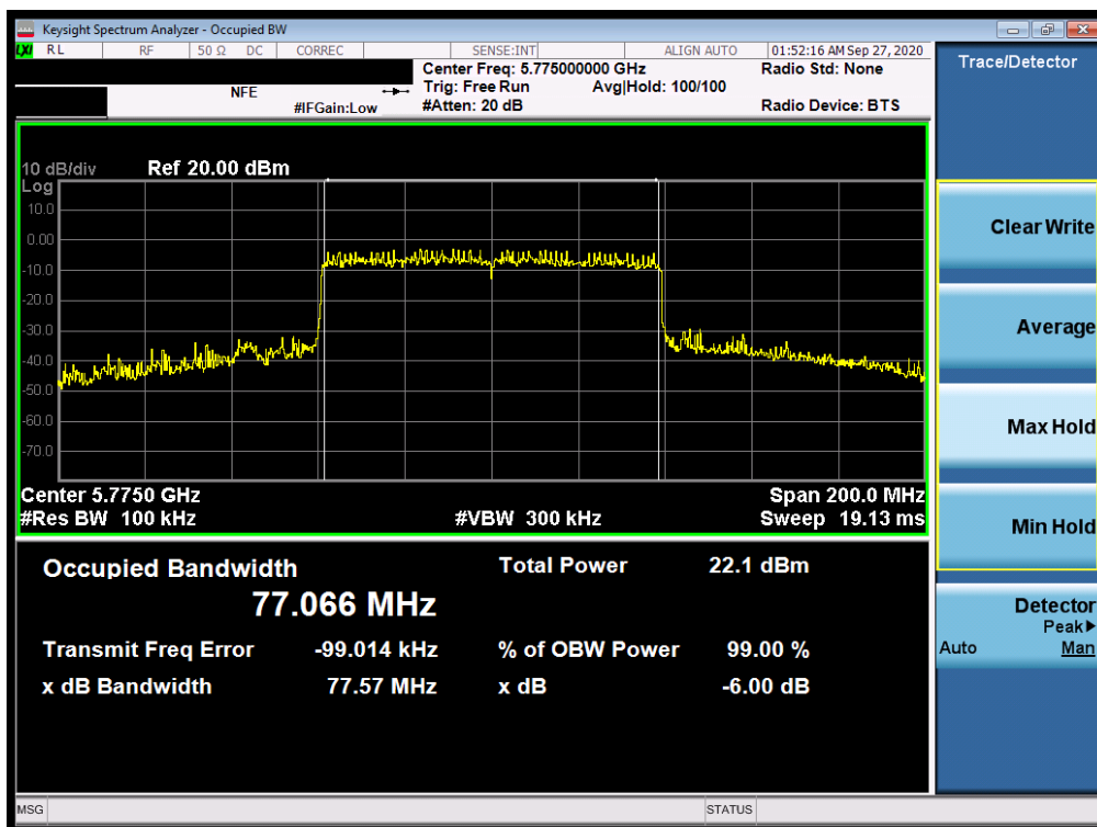
Plot 7-108. 6dB Bandwidth Plot SISO ANT2 (80MHz BW 802.11ax – 996 Tones (UNII Band 3) – Ch. 155)
