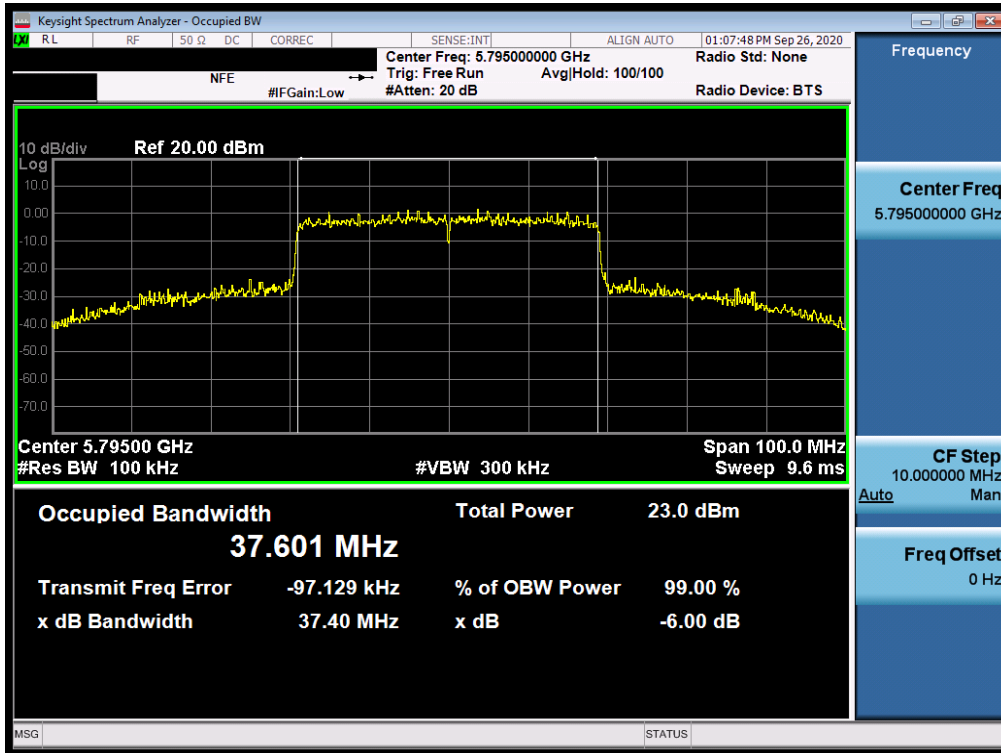
Plot 7-95. 6dB Bandwidth Plot SISO ANT1 (40MHz BW 802.11ax – 484 Tones (UNII Band 3) – Ch. 159)
