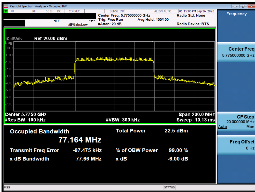
Plot 7-96. 6dB Bandwidth Plot SISO ANT1 (80MHz BW 802.11ax – 996 Tones (UNII Band 3) – Ch. 155)
