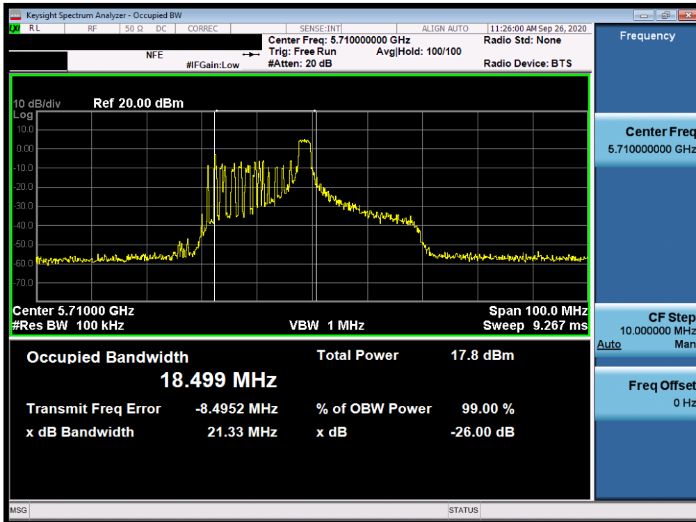
Plot 7-18. 26dB Bandwidth Plot SISO ANT1 (40MHz BW 802.11ax – 26 Tones (UNII Band 2C) – Ch. 142)
