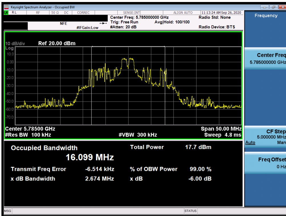
Plot 7-86. 6dB Bandwidth Plot SISO ANT1 (20MHz BW 802.11ax – 26 Tones (UNII Band 3) – Ch. 157)
