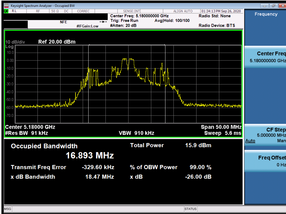
Plot 7-1. 26dB Bandwidth Plot SISO ANT1 (20MHz BW 802.11ax – 26 Tones (UNII Band 1) – Ch. 36)
