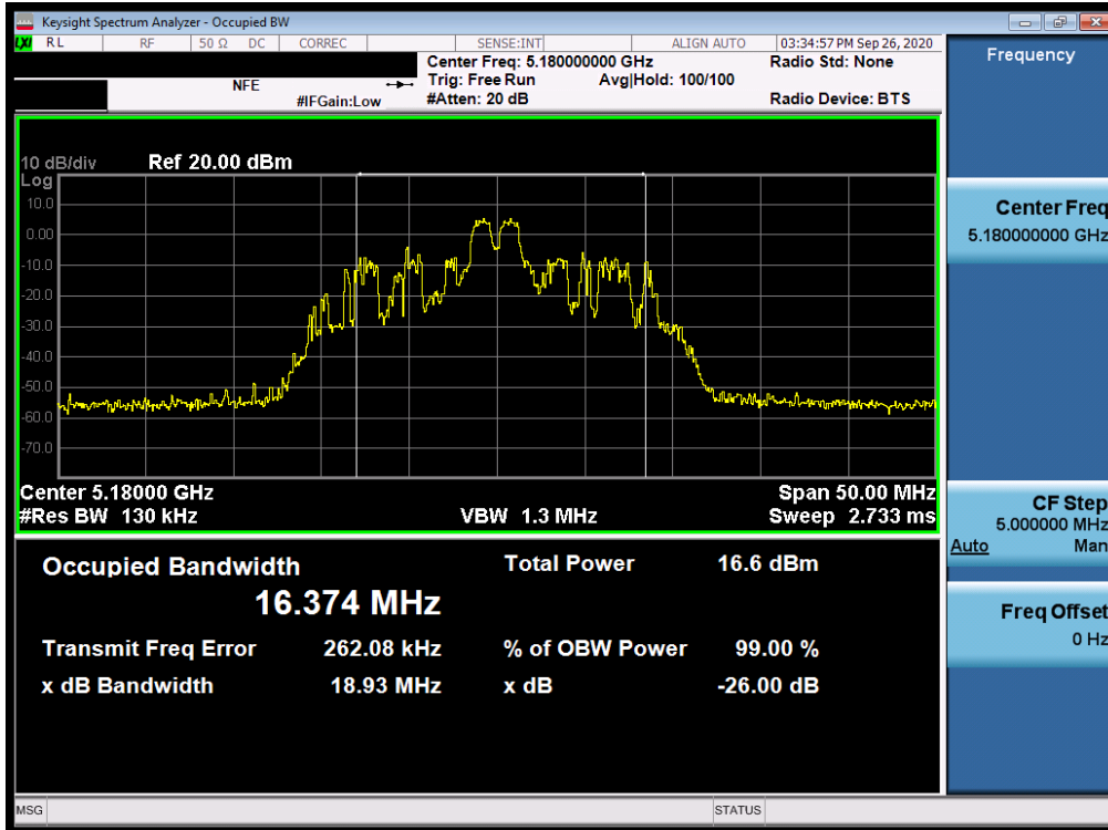
Plot 7-43. 26dB Bandwidth Plot SISO ANT2 (20MHz BW 802.11ax – 26 Tones (UNII Band 1) – Ch. 36)
