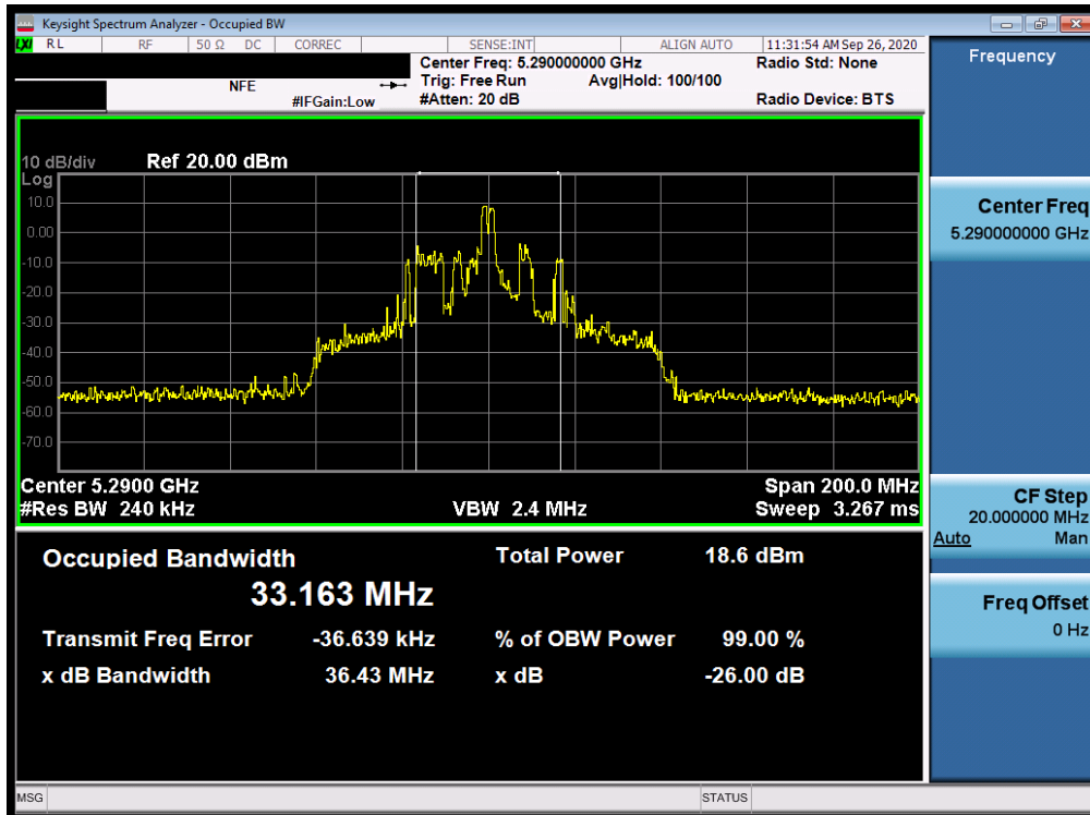
Plot 7-12. 26dB Bandwidth Plot SISO ANT1 (80MHz BW 802.11ax – 26 Tones (UNII Band 2A) – Ch. 58)
