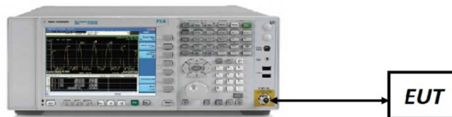
Figure 7-3. Test Instrument & Measurement Setup
