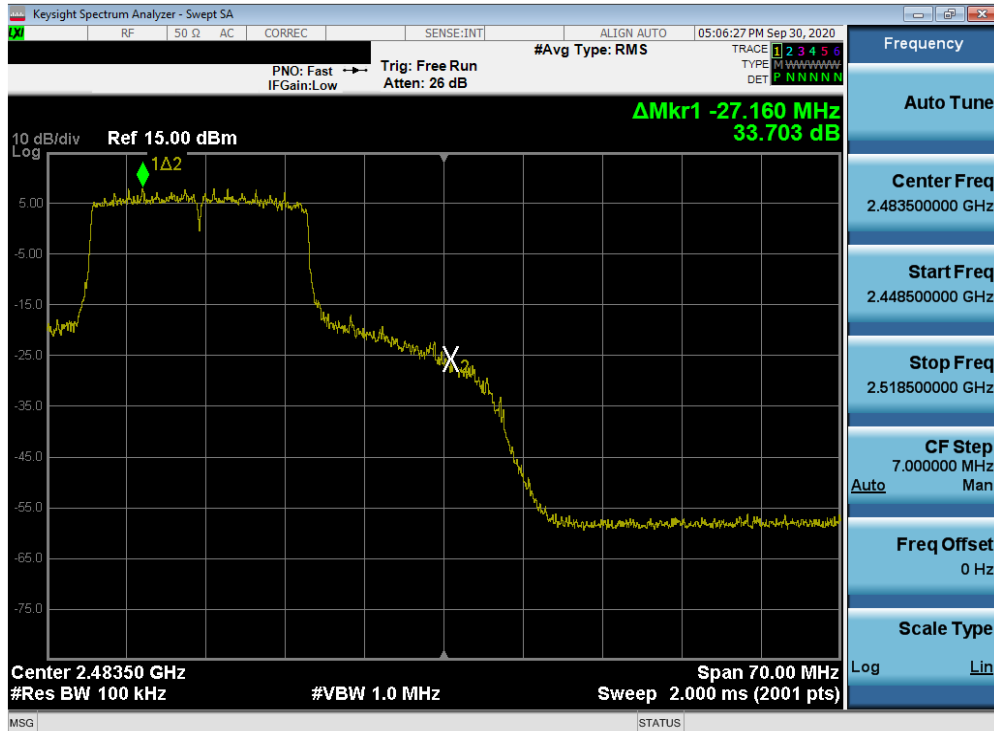
Plot 7-40. Band Edge Plot SISO ANT1 (802.11ax OFDMA – 242 Tones – Ch. 11)
