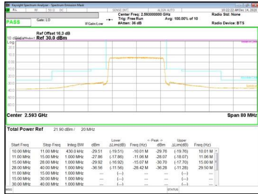
16QAM Mid channel FRB
