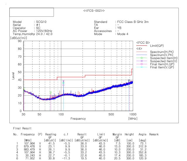
\* Radiated emissions (Rx frequency 107.964 MHz) from the transceiver shall be ignored
