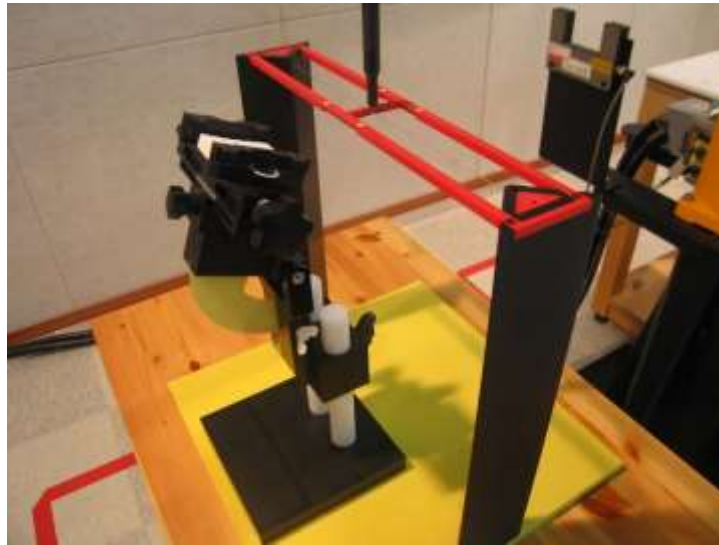
Figure 2. HAC Phantom & Device Holder
