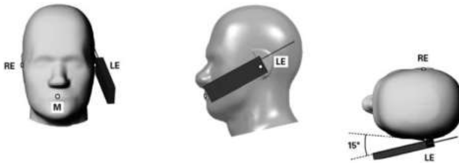
Figure 8.5. Tilt 15°position of the wireless device
