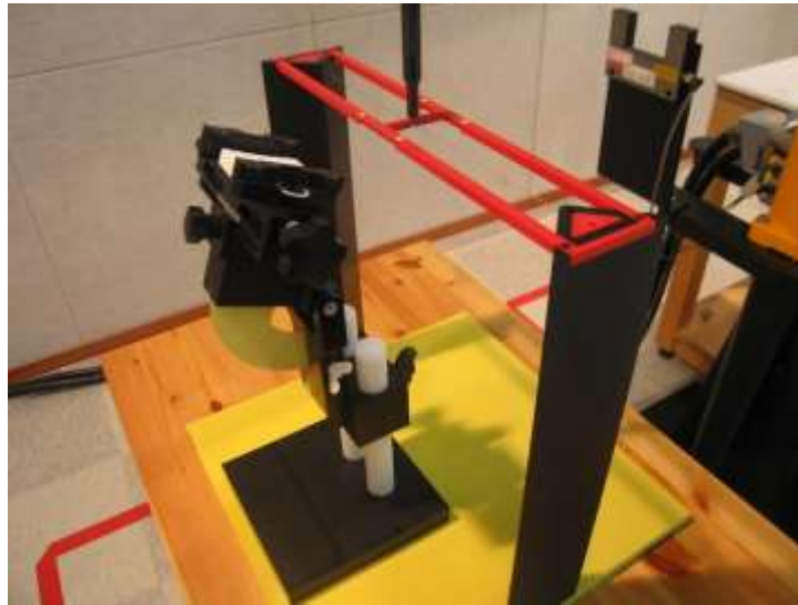
Figure 2. HAC Phantom & Device Holder
