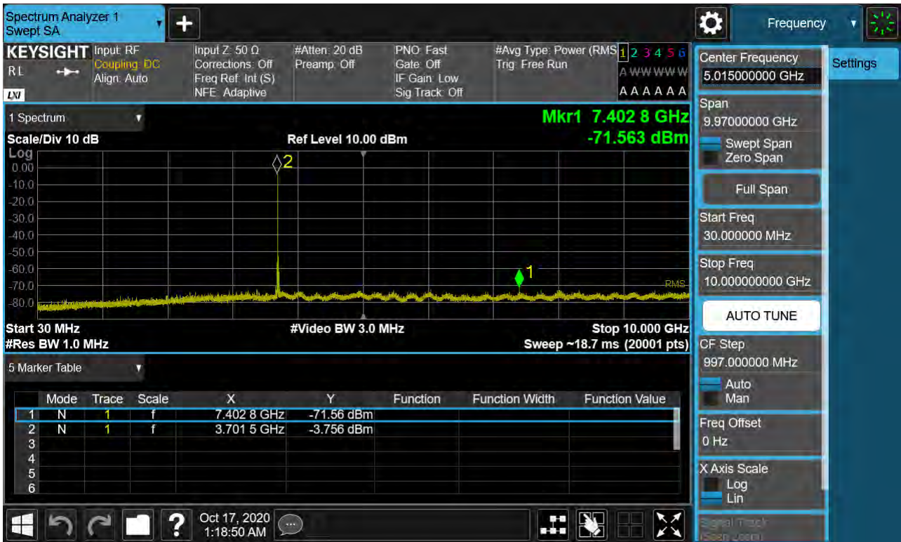
Sub6 n77. Conducted Spurious Plot_1 (648000ch_40MHz_BPSK)
