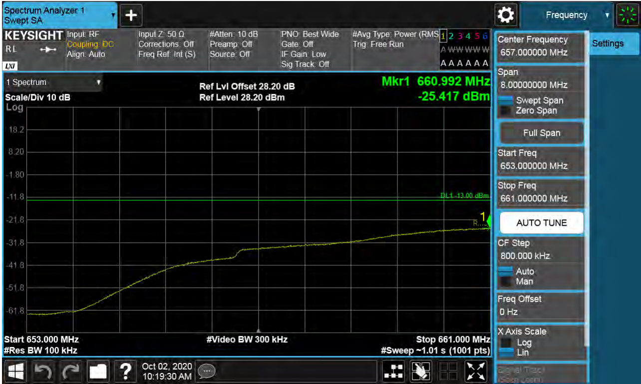
Sub6 n71. Lower Extended Band Edge Plot (15M BW Ch.134100 BPSK_RB25_0)
