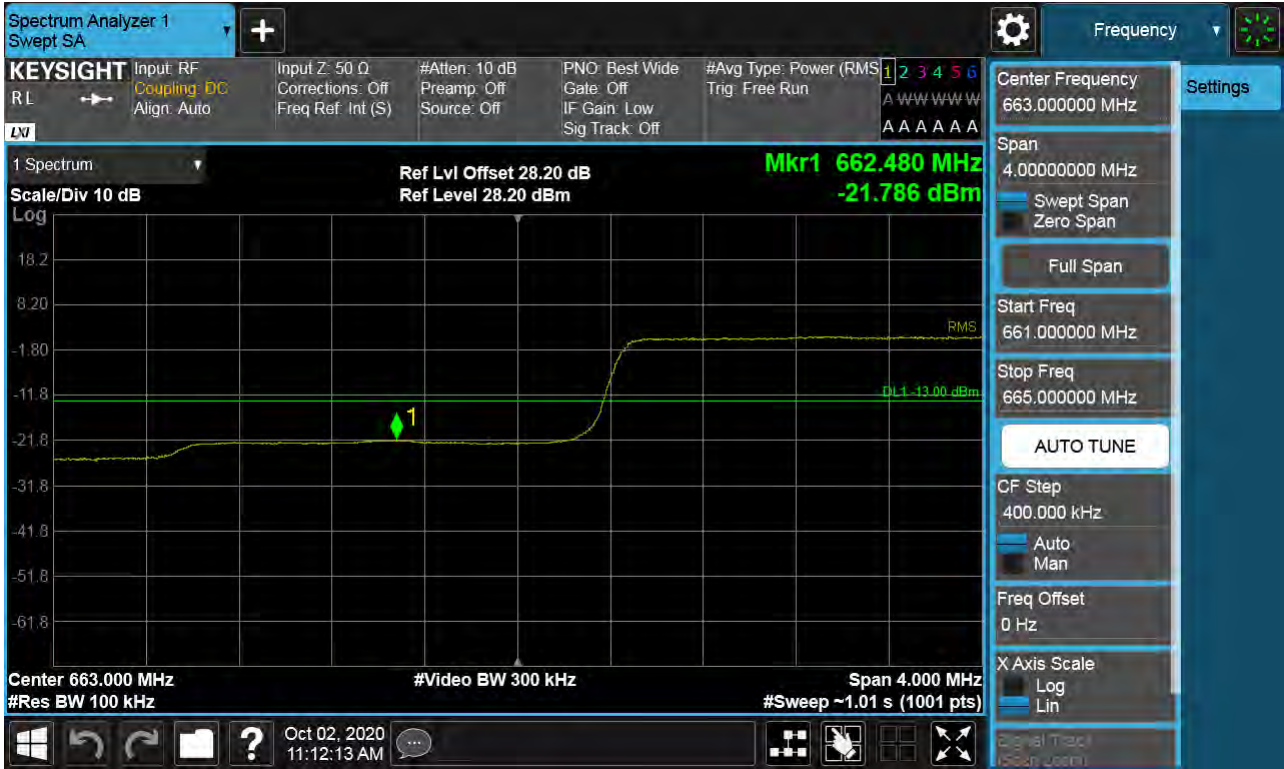
Sub6 n71. Lower Band Edge Plot (20M BW Ch.134600 BPSK_RB50_Offset 0)
