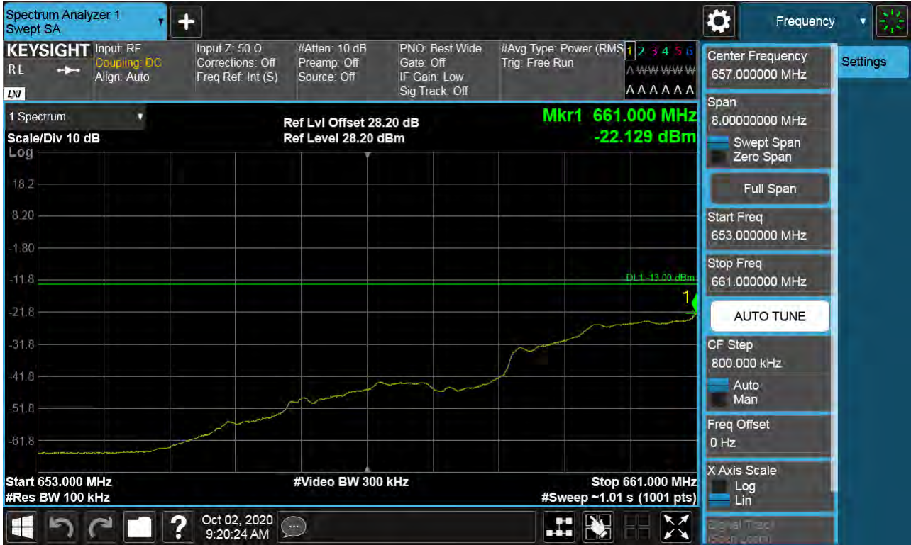
Sub6 n71. Lower Extended Band Edge Plot (5M BW Ch.133100 BPSK_RB6_0)
