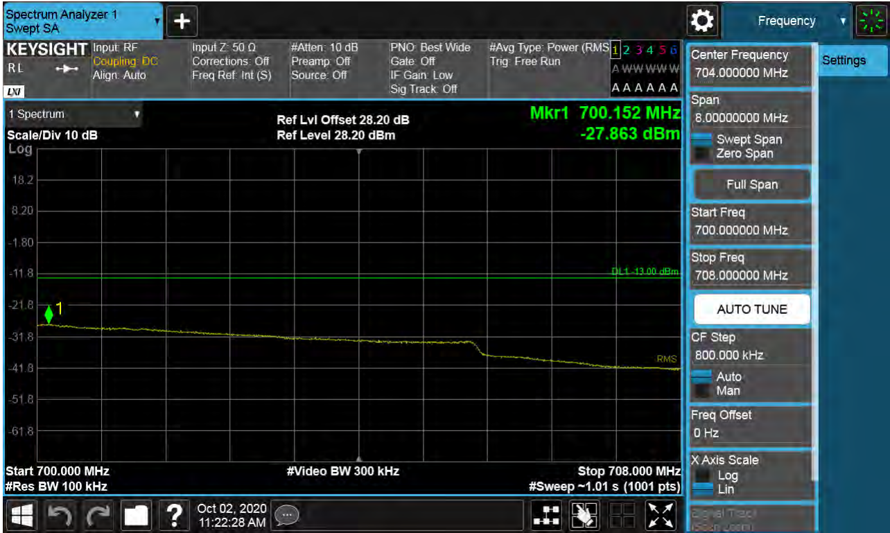
Sub6 n71. Upper Extended Band Edge Plot (20M BW Ch.137600 BPSK_RB50_0)
