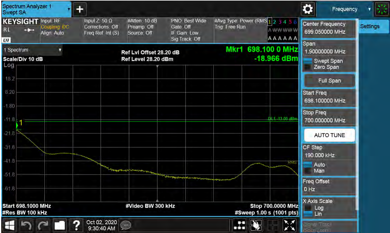
Sub6 n71. Upper Band Edge Plot (5M BW Ch.139100 BPSK_RB1_Offset 5)_2
