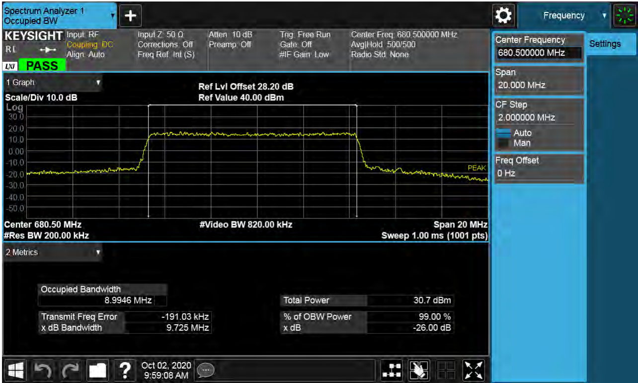
Sub6 n71. Occupied Bandwidth Plot (10M BW Ch.136100 64QAM_RB15_0)
