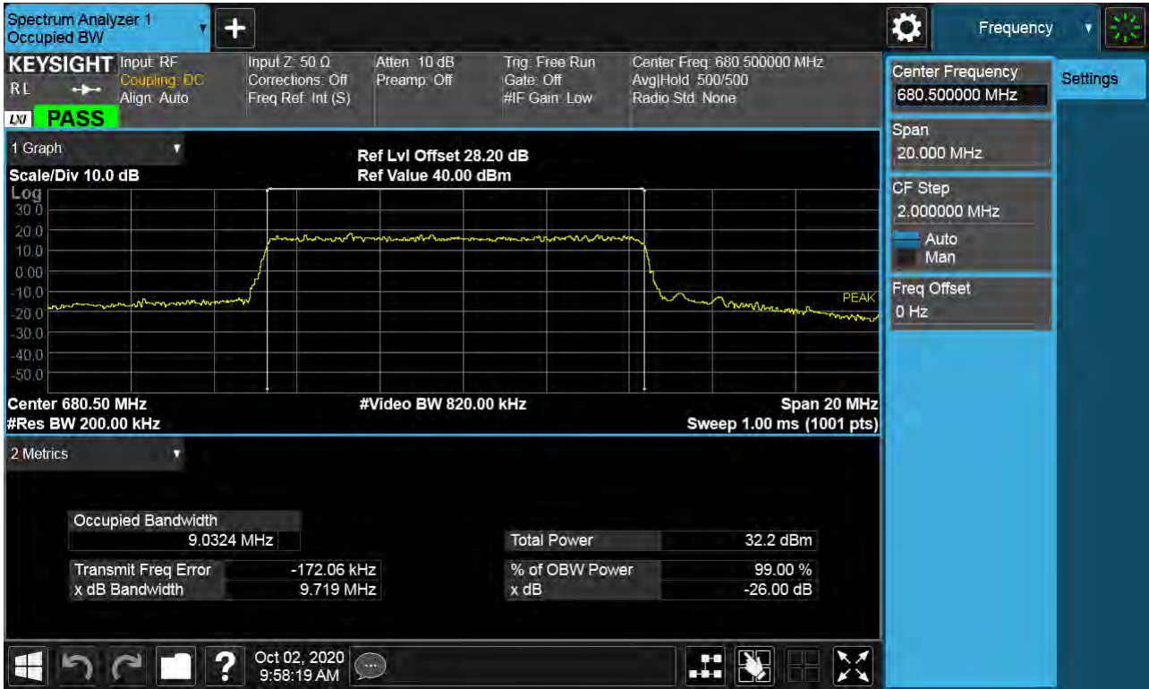
Sub6 n71. Occupied Bandwidth Plot (10M BW Ch.136100 QPSK_RB15_0)
