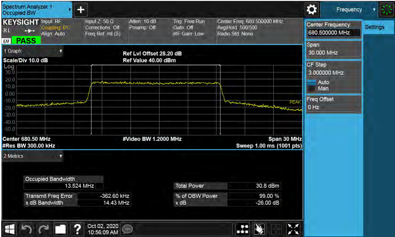
Sub6 n71. Occupied Bandwidth Plot (15M BW Ch.136100 64QAM_RB25_0)
