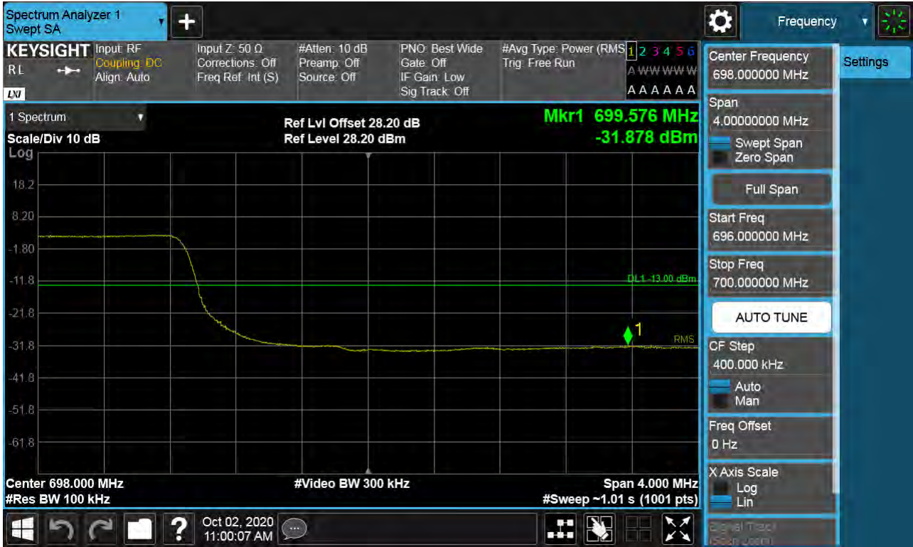
Sub6 n71. Upper Band Edge Plot (15M BW Ch.138100 BPSK_RB25_Offset 0)
