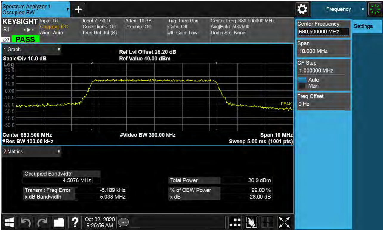
Sub6 n71. Occupied Bandwidth Plot (5M BW Ch.136100 64QAM_RB6_0)
