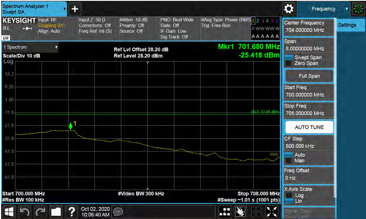
Sub6 n71. Upper Extended Band Edge Plot (10M BW Ch.138600 BPSK_RB15_0)
