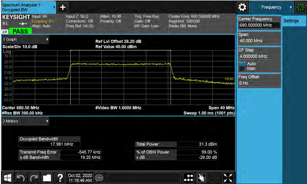
Sub6 n71. Occupied Bandwidth Plot (20M BW Ch.136100 16QAM_RB50_0)
