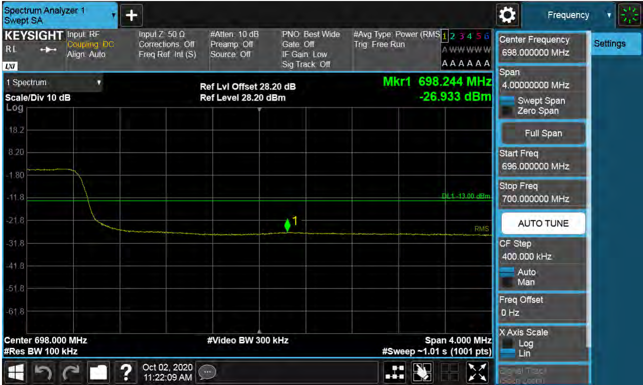
Sub6 n71. Upper Band Edge Plot (20M BW Ch.137600 BPSK_RB50_Offset 0)
