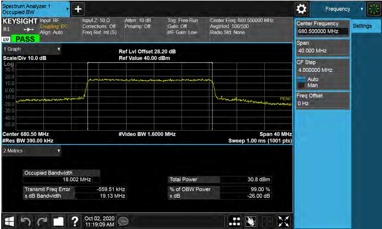
Sub6 n71. Occupied Bandwidth Plot (20M BW Ch.136100 64QAM_RB50_0)
