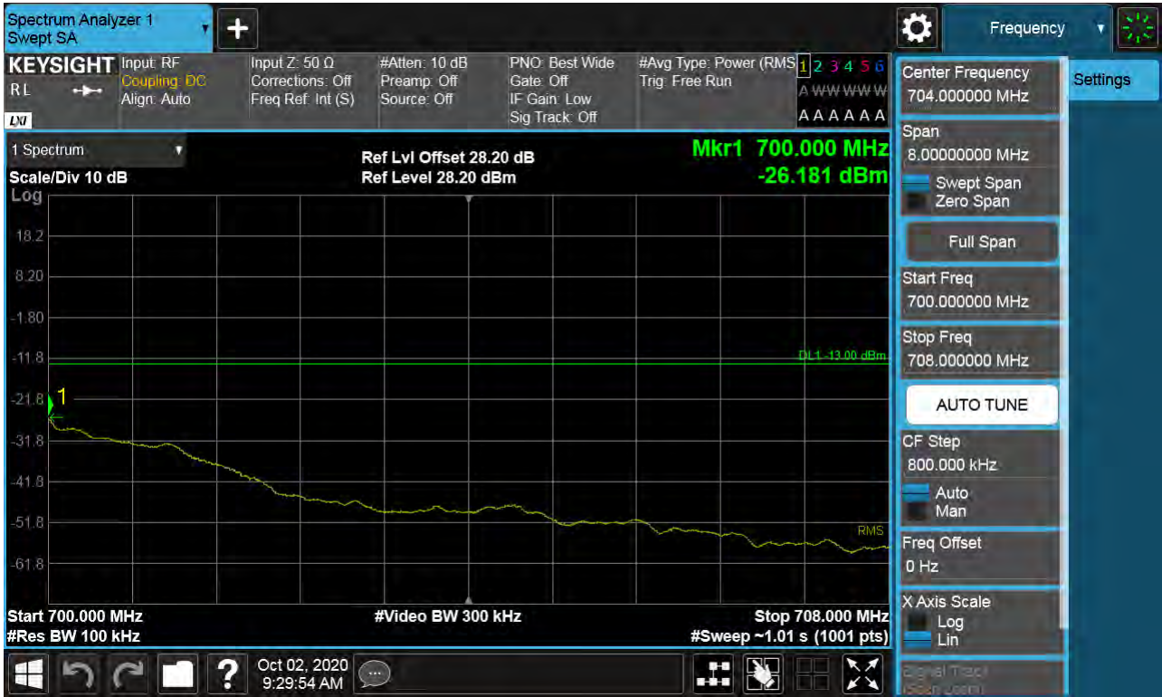
Sub6 n71. Upper Extended Band Edge Plot (5M BW Ch.139100 BPSK_RB6_0)
