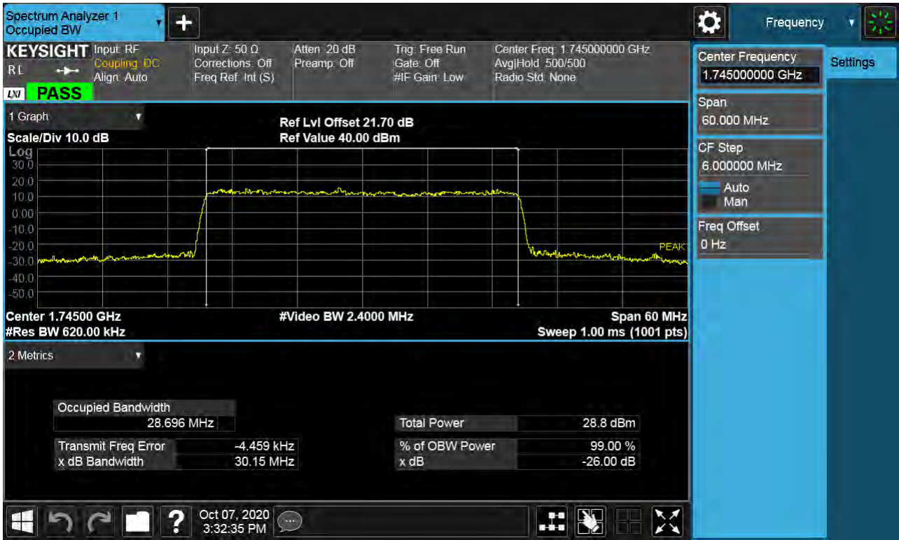
Sub6 n66. Occupied Bandwidth Plot (30M BW Ch.349000 256QAM RB 160)
