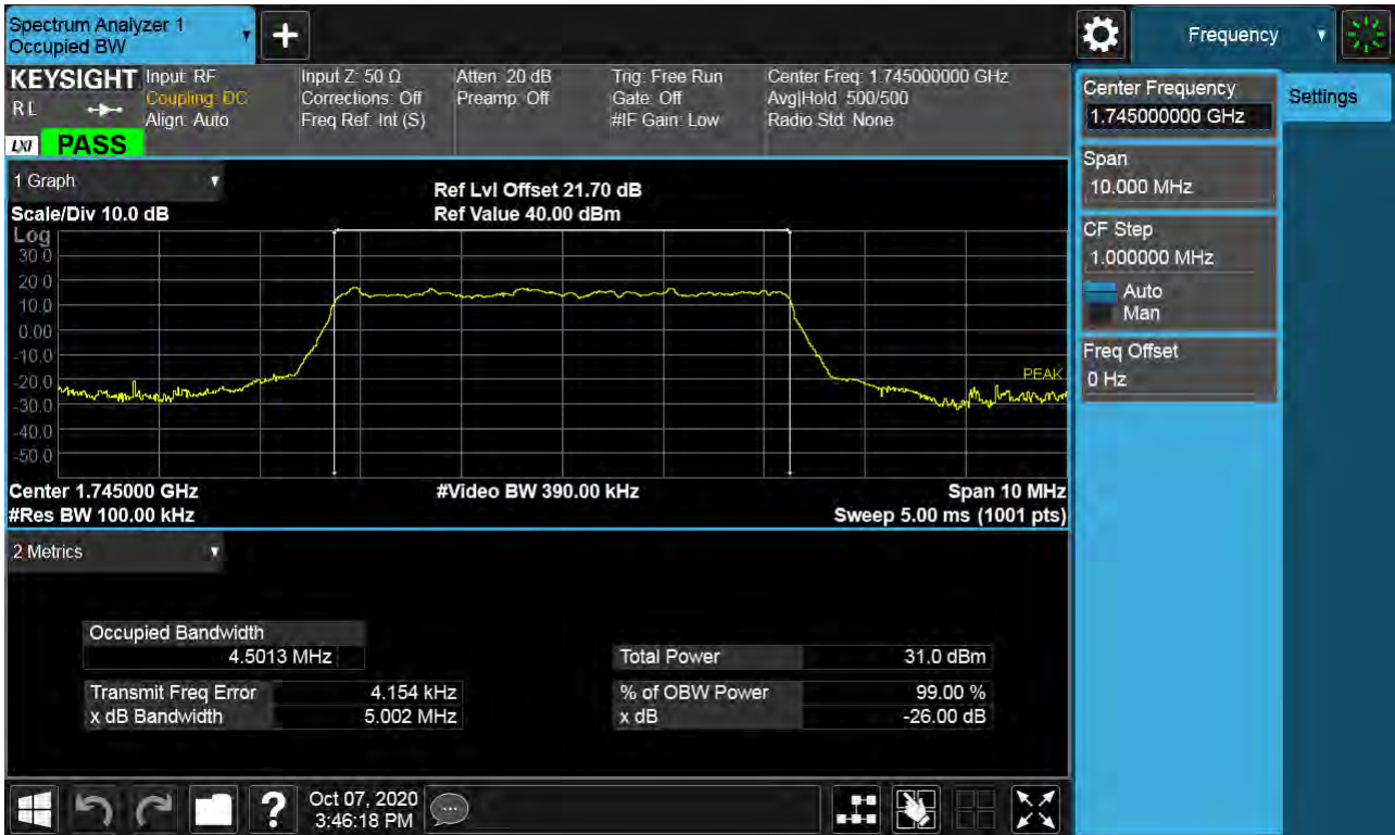
Sub6 n66. Occupied Bandwidth Plot (5M BW Ch.349000 QPSK RB 25)
