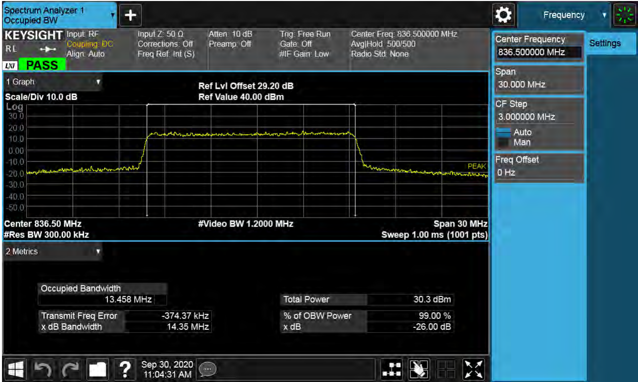
Sub6 n5. Occupied Bandwidth Plot (15M BW Ch.167300 64QAM_RB25_0)
