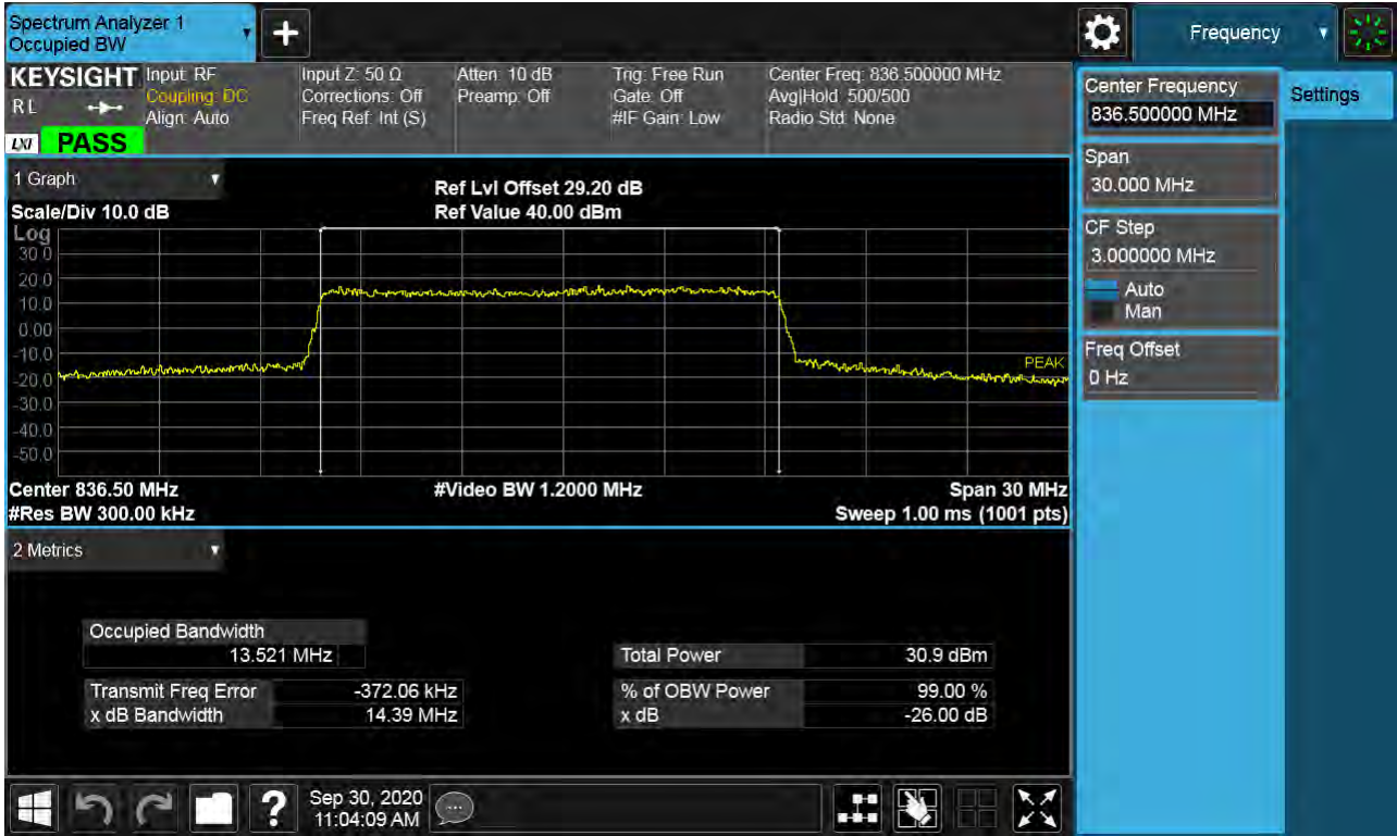
Sub6 n5. Occupied Bandwidth Plot (15M BW Ch.167300 16QAM_RB25_0)
