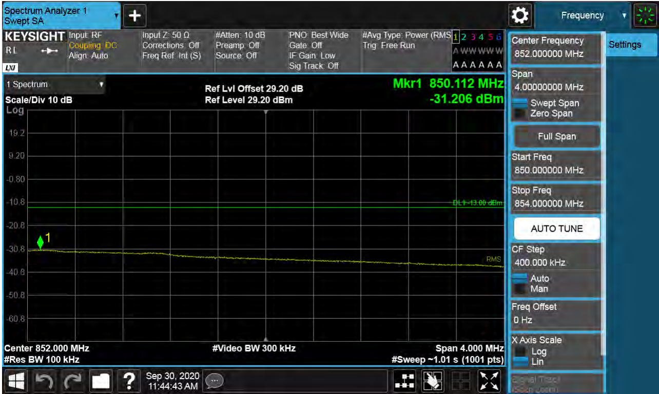
Sub6 n5. Upper Extended Band Edge Plot (20M BW Ch.167800 BPSK_RB100_0)
