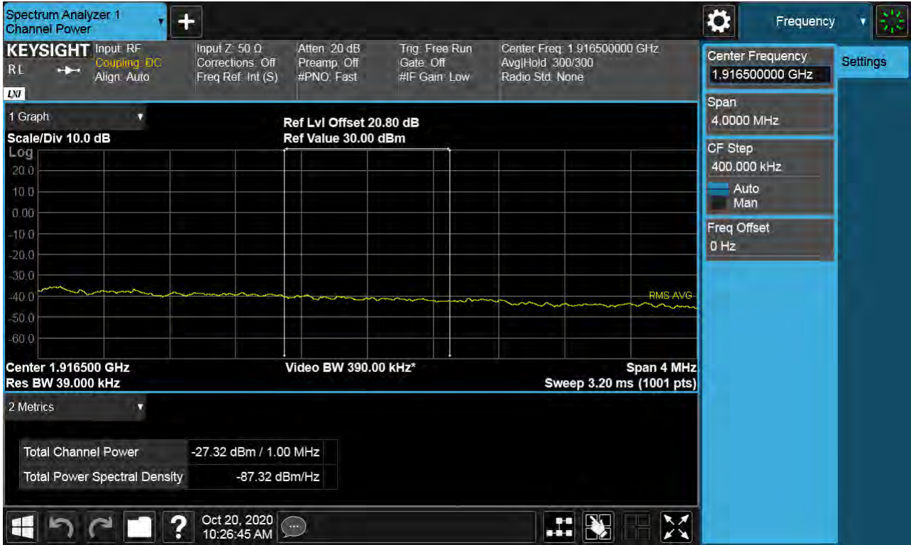
Sub6 n25(2). Upper Extended Band Edge Plot (25M BW Ch.380500 BPSK_RB128_0) -2
