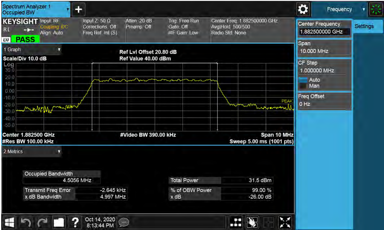
Sub6 n25(2). Occupied Bandwidth Plot (5M BW Ch.376500 BPSK )
