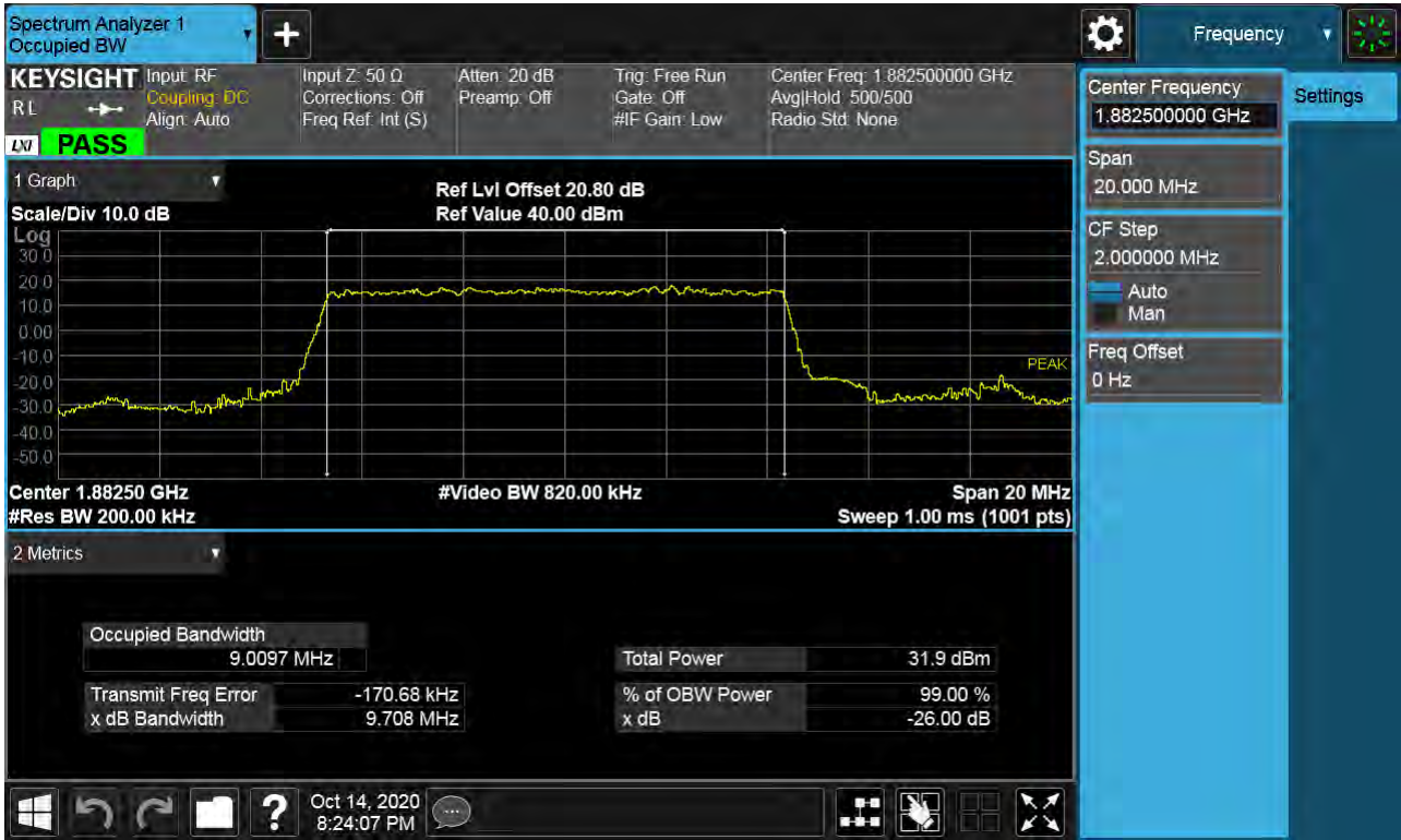
Sub6 n25(2). Occupied Bandwidth Plot (10M BW Ch.376500 BPSK RB 50_0)
