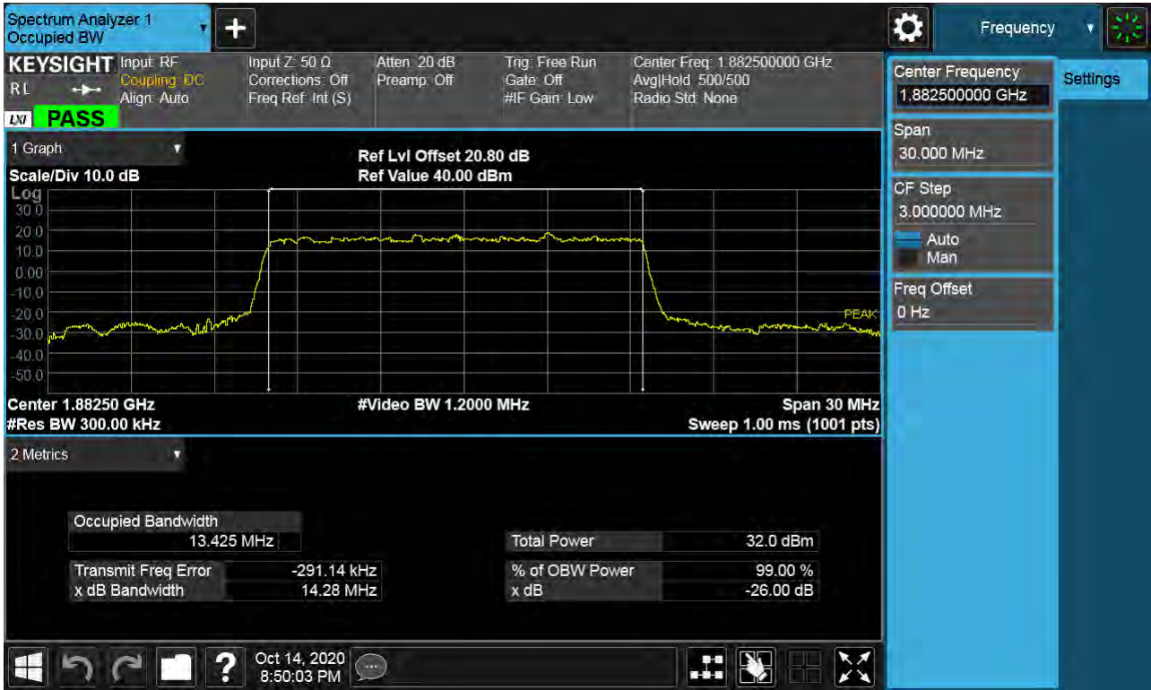
Sub6 n25(2). Occupied Bandwidth Plot (15M BW Ch.376500 BPSK RB 75_0)
