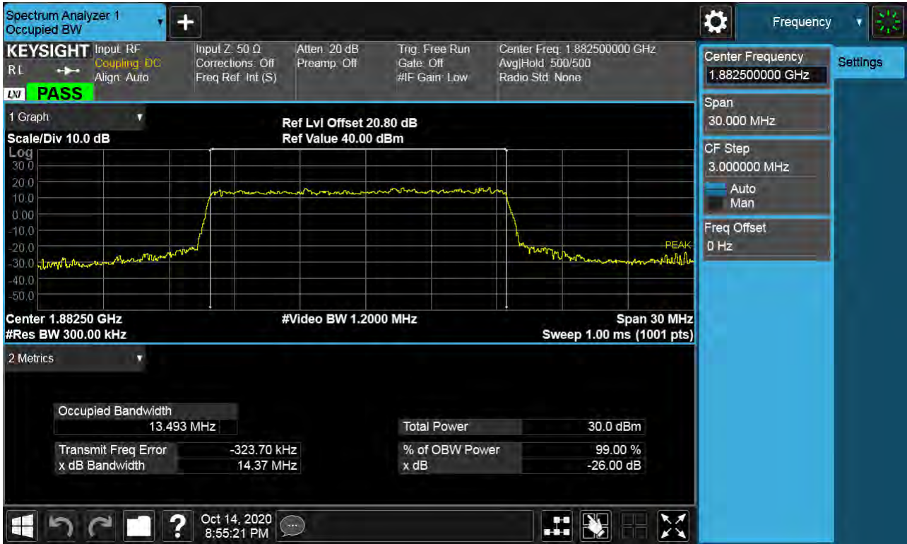
Sub6 n25(2). Occupied Bandwidth Plot (15M BW Ch.376500 64QAM RB 75_0)
