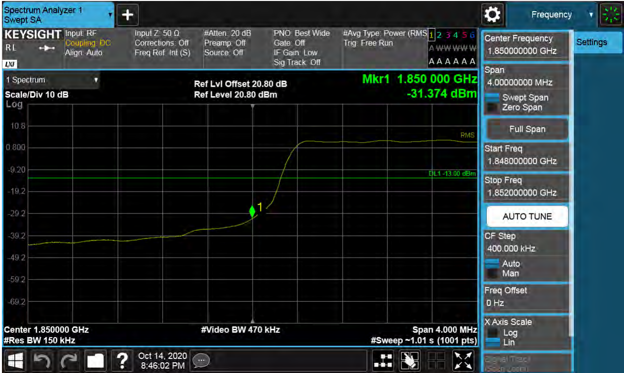
Sub6 n25(2). Lower Band Edge Plot (15M BW Ch.371500 BPSK_RB75_Offset 0) -1
