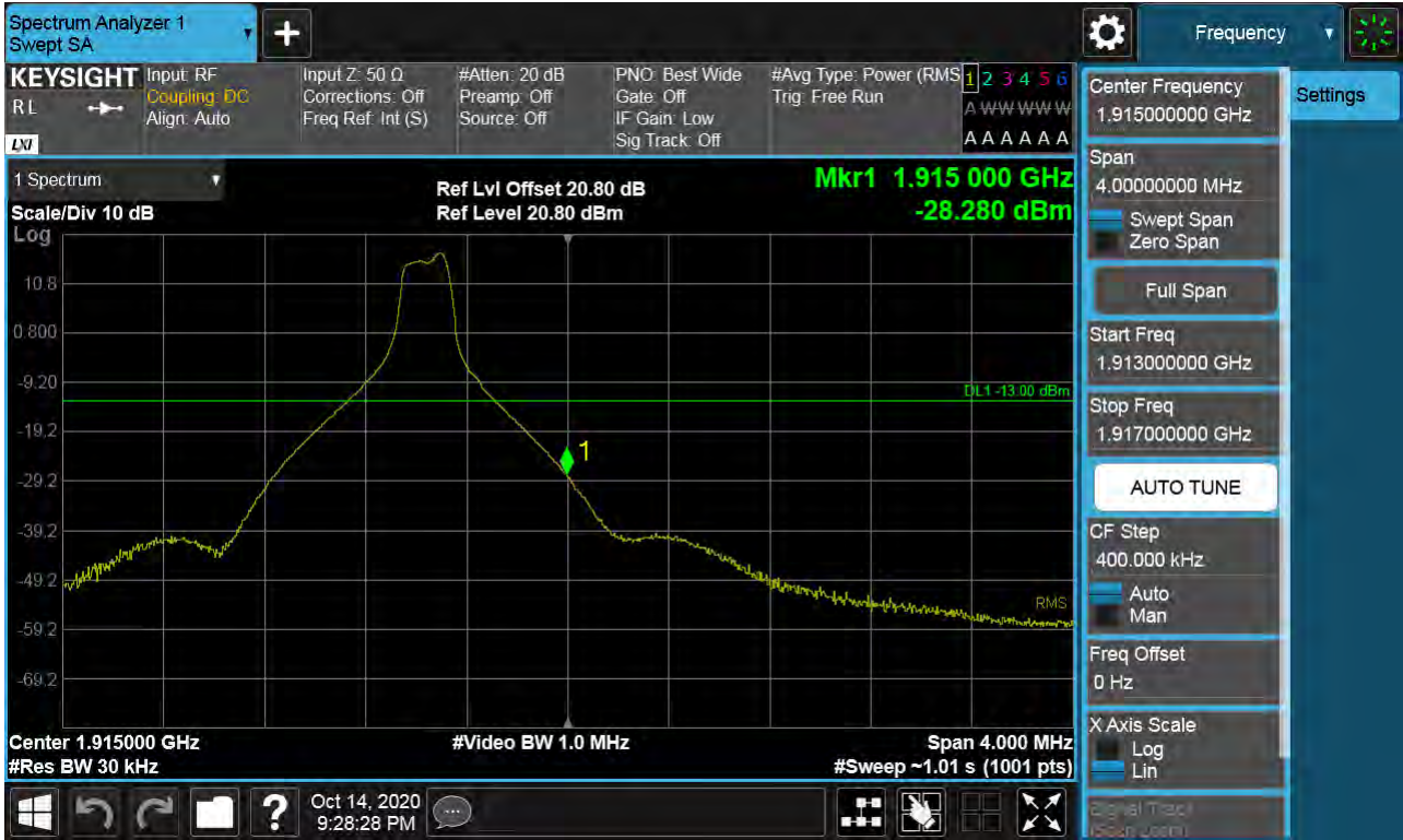
Sub6 n25(2). Upper Band Edge Plot (20M BW Ch.381000 BPSK_RB1_Offset 99)
