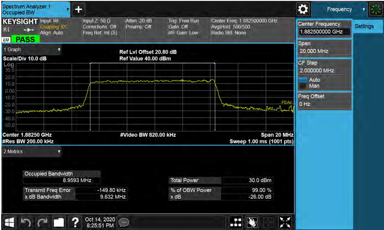
Sub6 n25(2). Occupied Bandwidth Plot (10M BW Ch.376500 64QAM RB 50_0)
