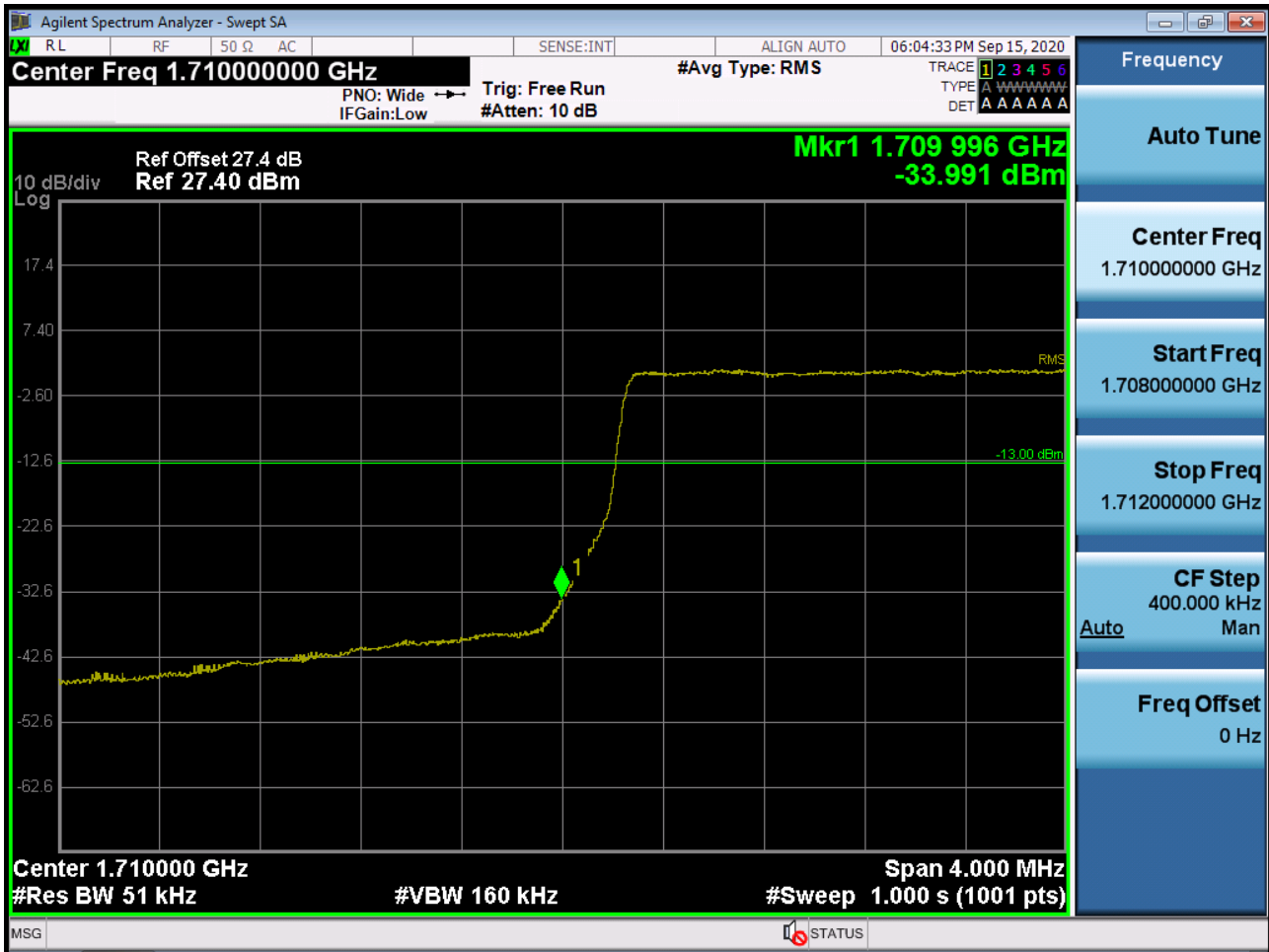
BAND 66/4. Lower Band Edge Plot (5M BW Ch.131997 QPSK RB 25_0) -2
