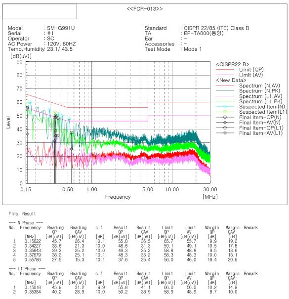
Note 1) Two graphs measured for both Live(L1) and Neutral(N) of the LISN are combined into one graph Note 2) Level (QP and/or CAV) = Meter Reading (QP and/or CAV) + Corr. (LISN Insertion Loss + Cable Loss) Margin (QP and/or CAV) = Limit – Level (QP and/or CAV)
