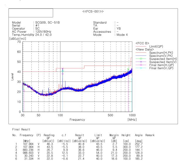
\* Radiated emissions (Rx frequency 107.964 MHz) from the transceiver shall be ignored
