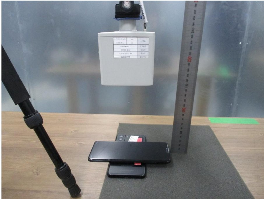
Top charger below client (20cm distance)
