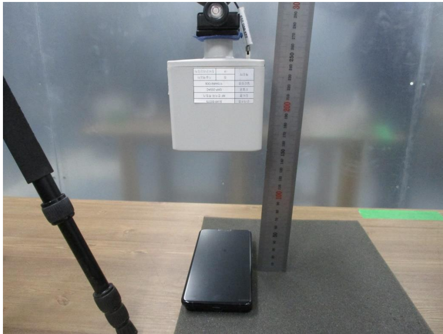
Top charger below client (20cm distance)
