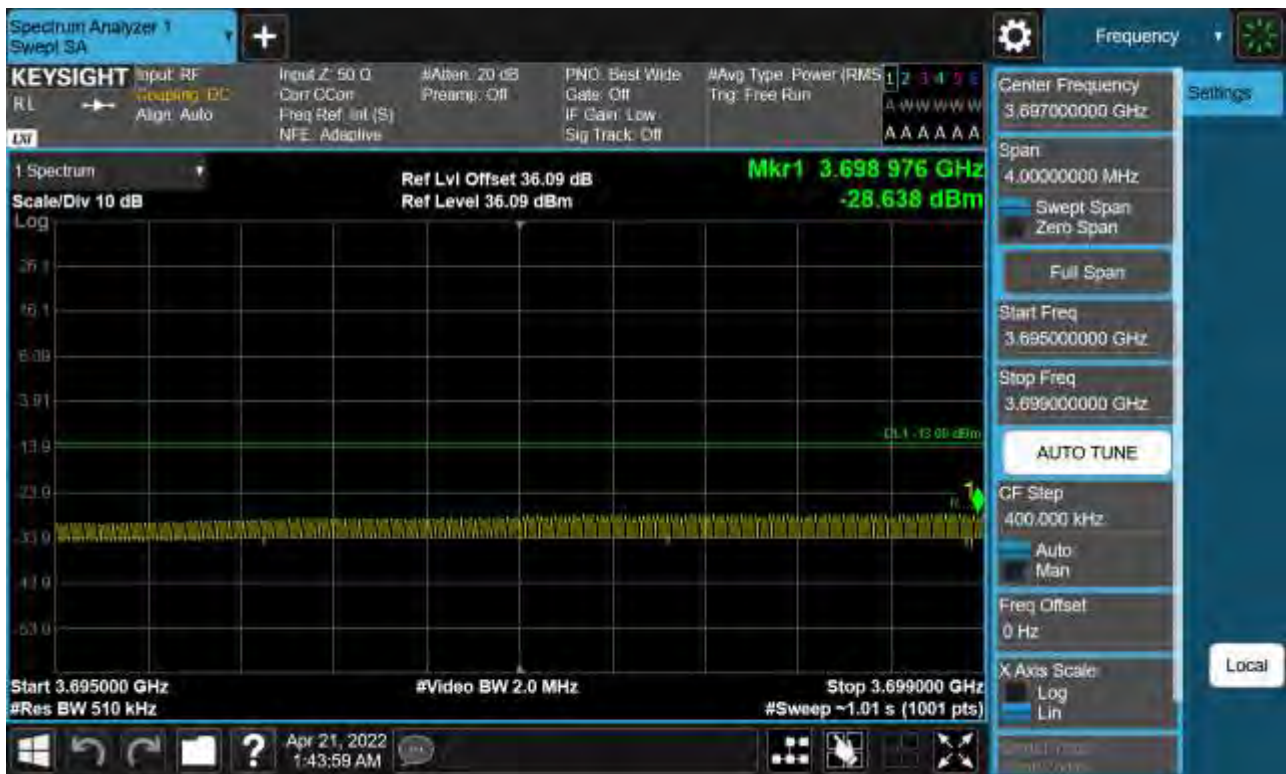
Sub6 n77. Low Band Edge Plot (80 M BW Ch.649334 BPSK FullRB)(2)
