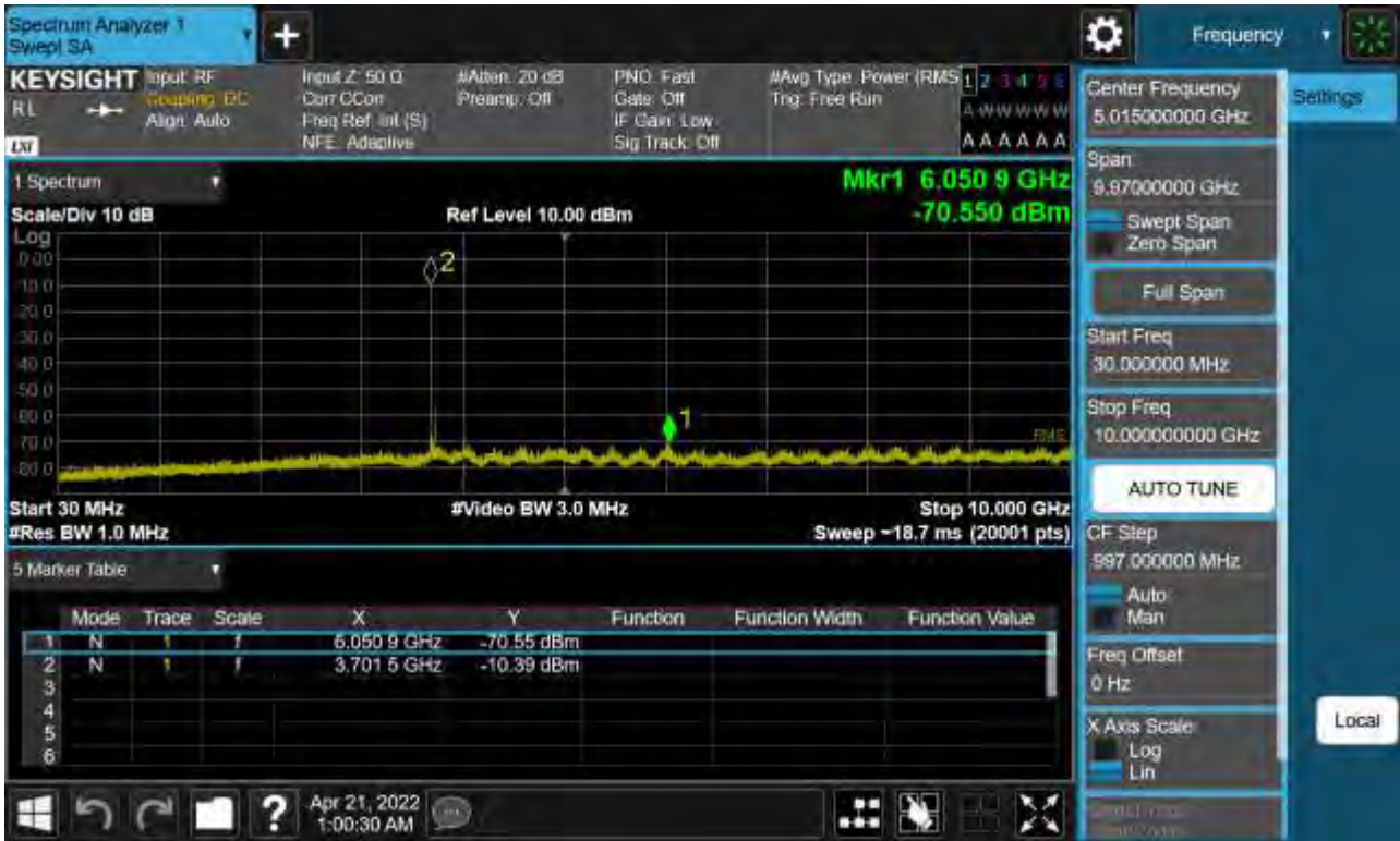
Sub6 n77. Conducted Spurious Plot_1 (648334ch_50 MHz_BPSK)
