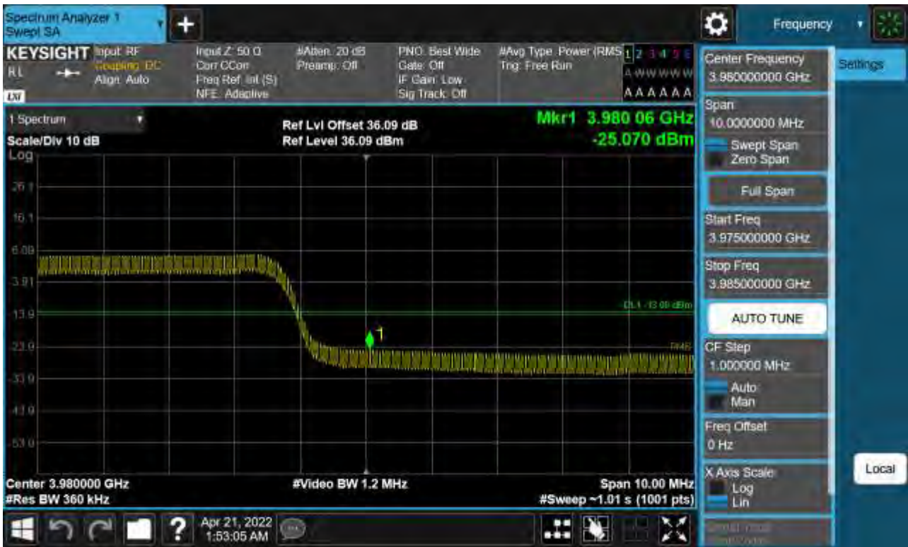
Sub6 n77. High Band Edge Plot (80 M BW Ch.662666 BPSK FullRB)(1)
