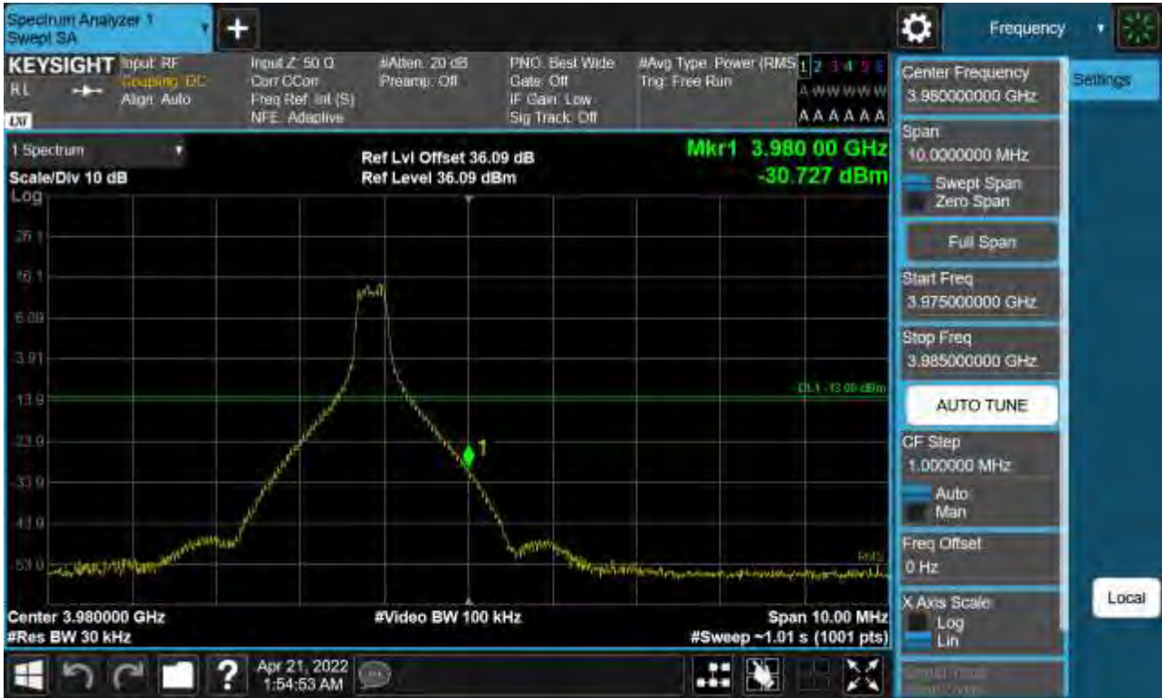
Sub6 n77. High Band Edge Plot (80 M BW Ch.662666 BPSK 1RB)(1)
