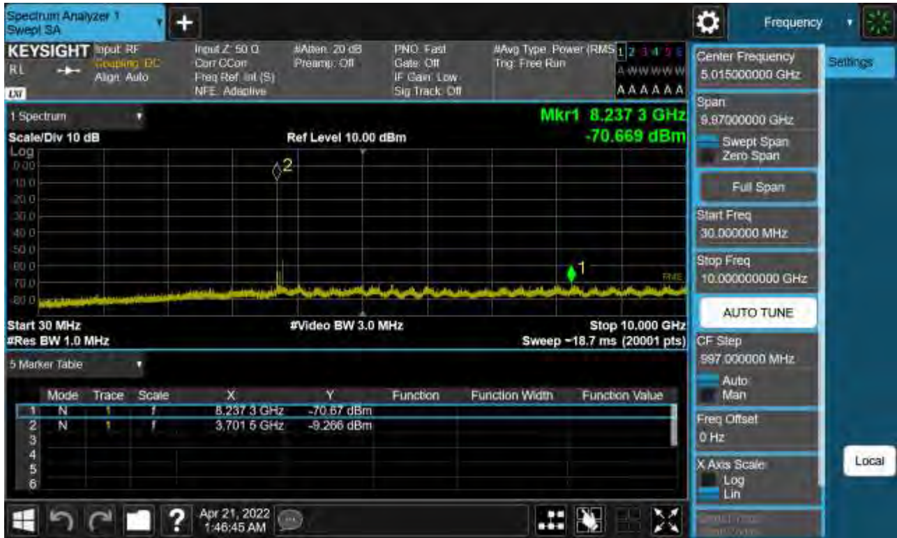
Sub6 n77. Conducted Spurious Plot_1 (649334ch_80 MHz_BPSK)
