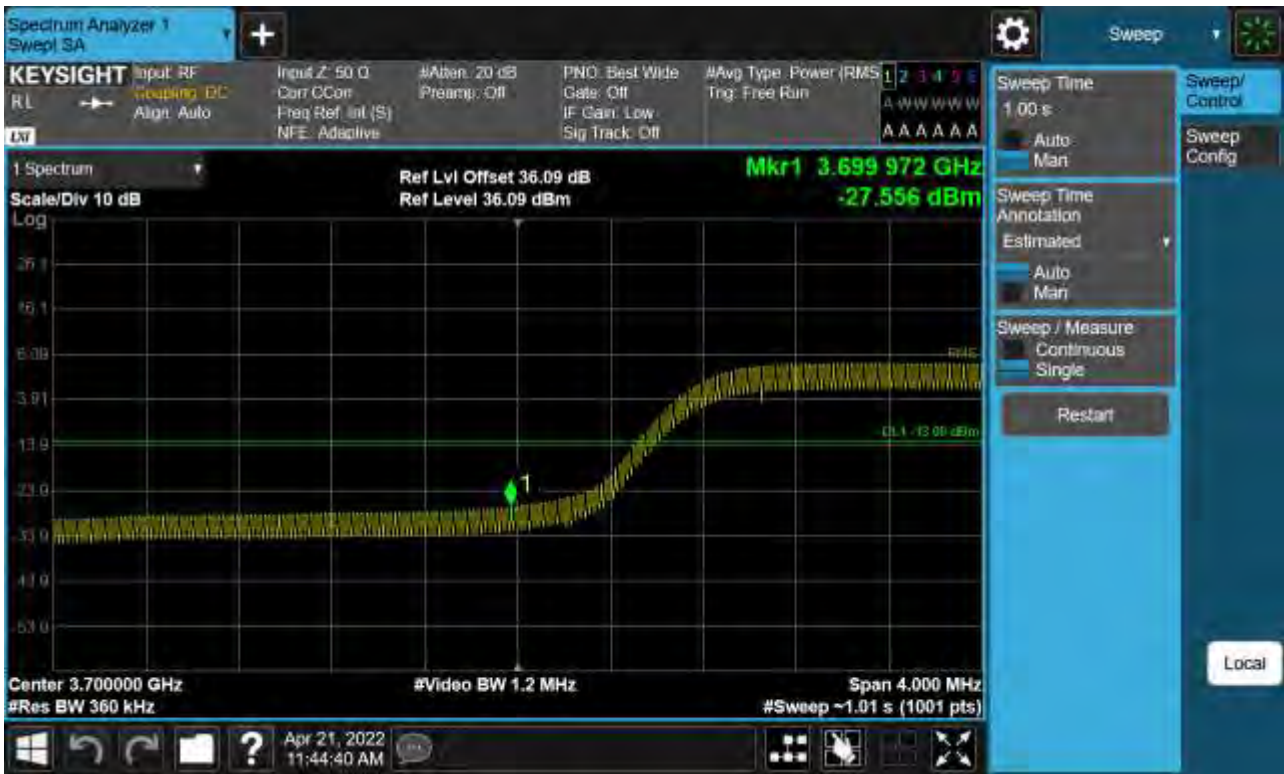
Sub6 n77. Low Band Edge Plot (100 M BW Ch.650000 BPSK FullRB)(1)
