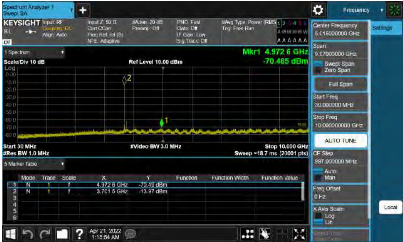
Sub6 n77. Conducted Spurious Plot_1 (648668ch_60 MHz_BPSK)
