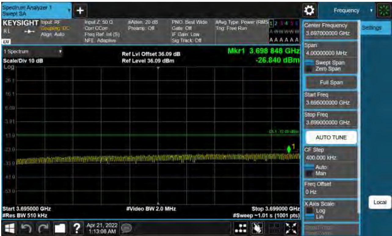
Sub6 n77. Low Band Edge Plot (60 M BW Ch.648668 BPSK FullRB)(2)
