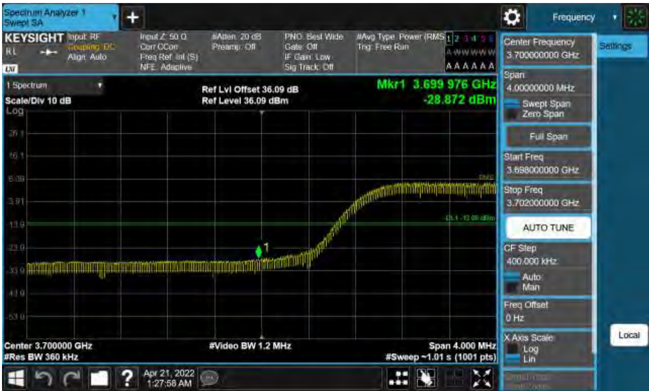
Sub6 n77. Low Band Edge Plot (70 M BW Ch.649000 BPSK FullRB)(1)
