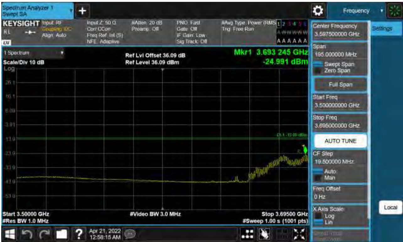
Sub6 n77. Low Band Edge Plot (50 M BW Ch.648334 BPSK FullRB)(3)
