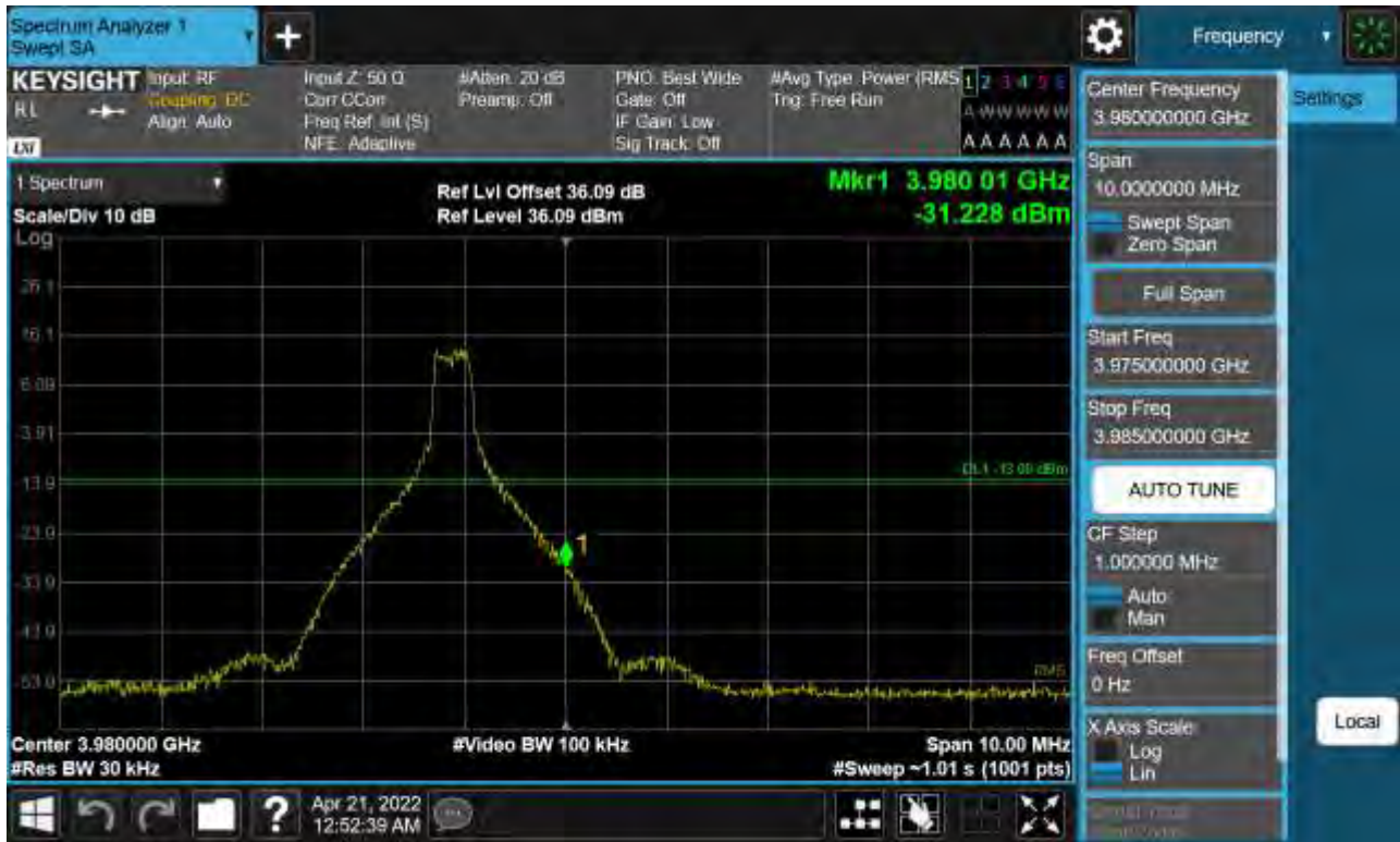
Sub6 n77. High Band Edge Plot (40 M BW Ch.664000 BPSK 1RB)(1)
