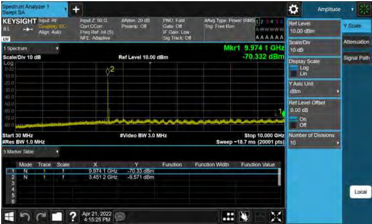
Sub6 n77. Conducted Spurious Plot_1 (632000ch_60 MHz_BPSK)
