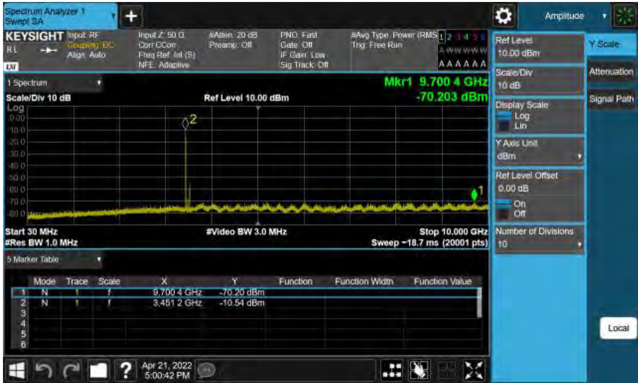
Sub6 n77. Conducted Spurious Plot_1 (633000ch_90 MHz_BPSK)
