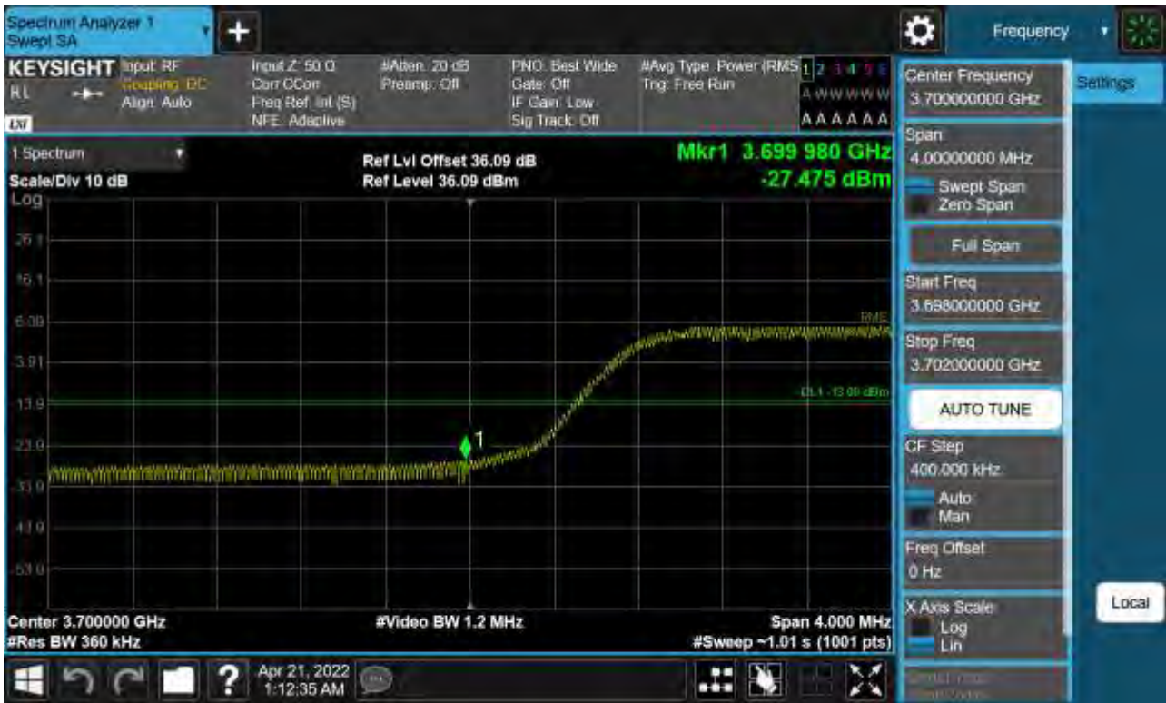
Sub6 n77. Low Band Edge Plot (60 M BW Ch.648668 BPSK FullRB)(1)
