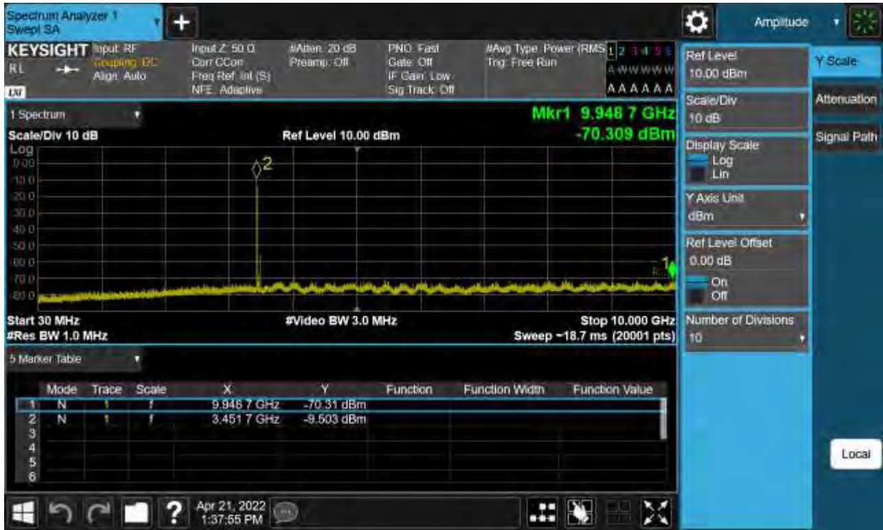
Sub6 n77. Conducted Spurious Plot_1 (631668ch_50 MHz_BPSK)
