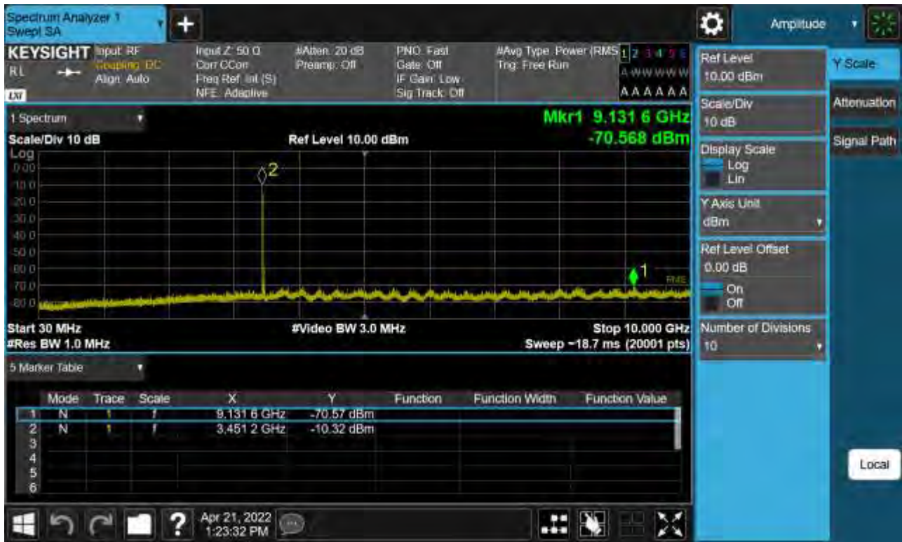
Sub6 n77. Conducted Spurious Plot_1 (631334ch_40 MHz_BPSK)
