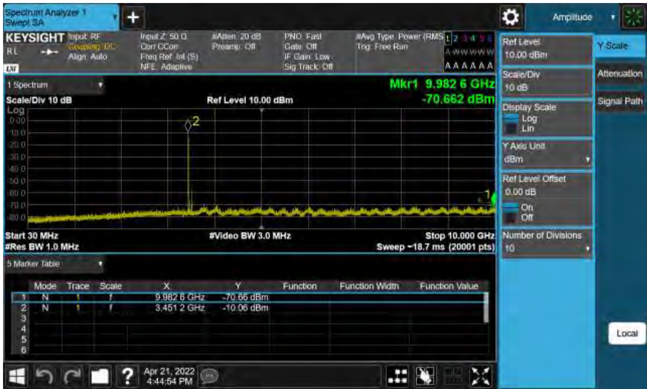
Sub6 n77. Conducted Spurious Plot_1 (632668ch_80 MHz_BPSK)
