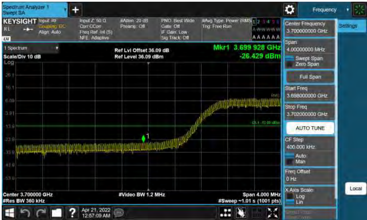
Sub6 n77. Low Band Edge Plot (50 M BW Ch.648334 BPSK FullRB)(1)
