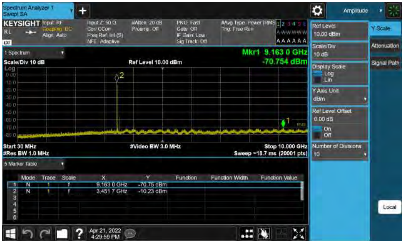
Sub6 n77. Conducted Spurious Plot_1 (632334ch_70 MHz_BPSK)
