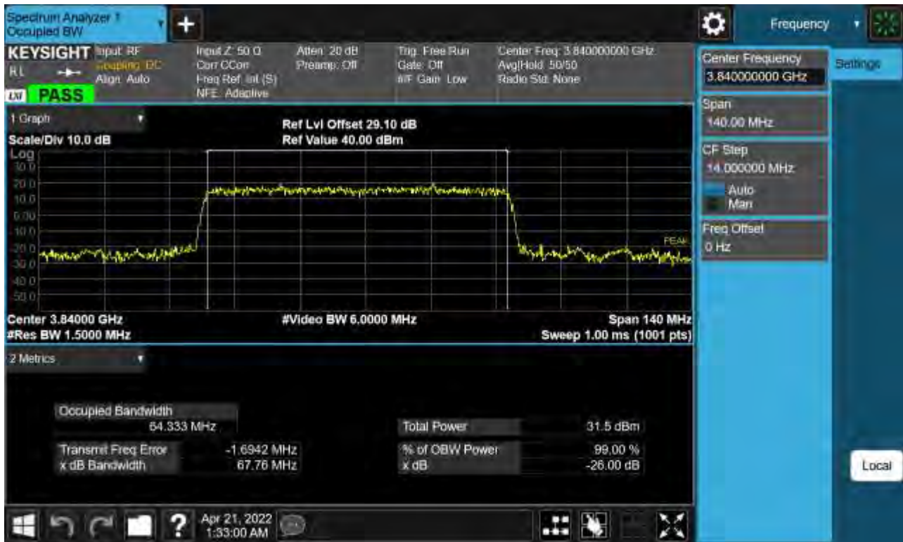
Sub6 n77. Occupied Bandwidth Plot (70 M BW Ch.656000 BPSK )
