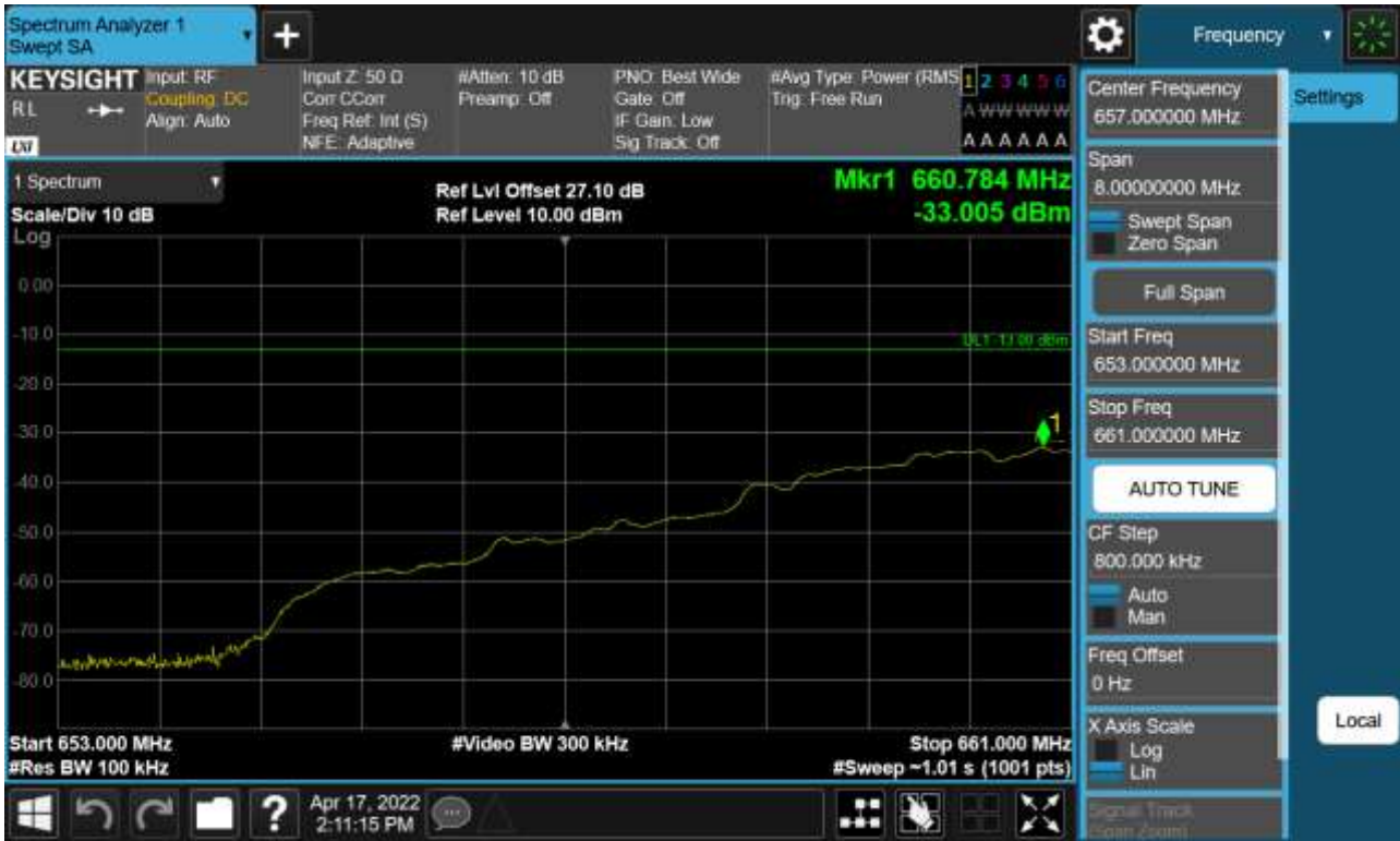
Sub6 n71. Lower Extended Band Edge Plot (10 M BW Ch.133600 BPSK_ Full RB)
