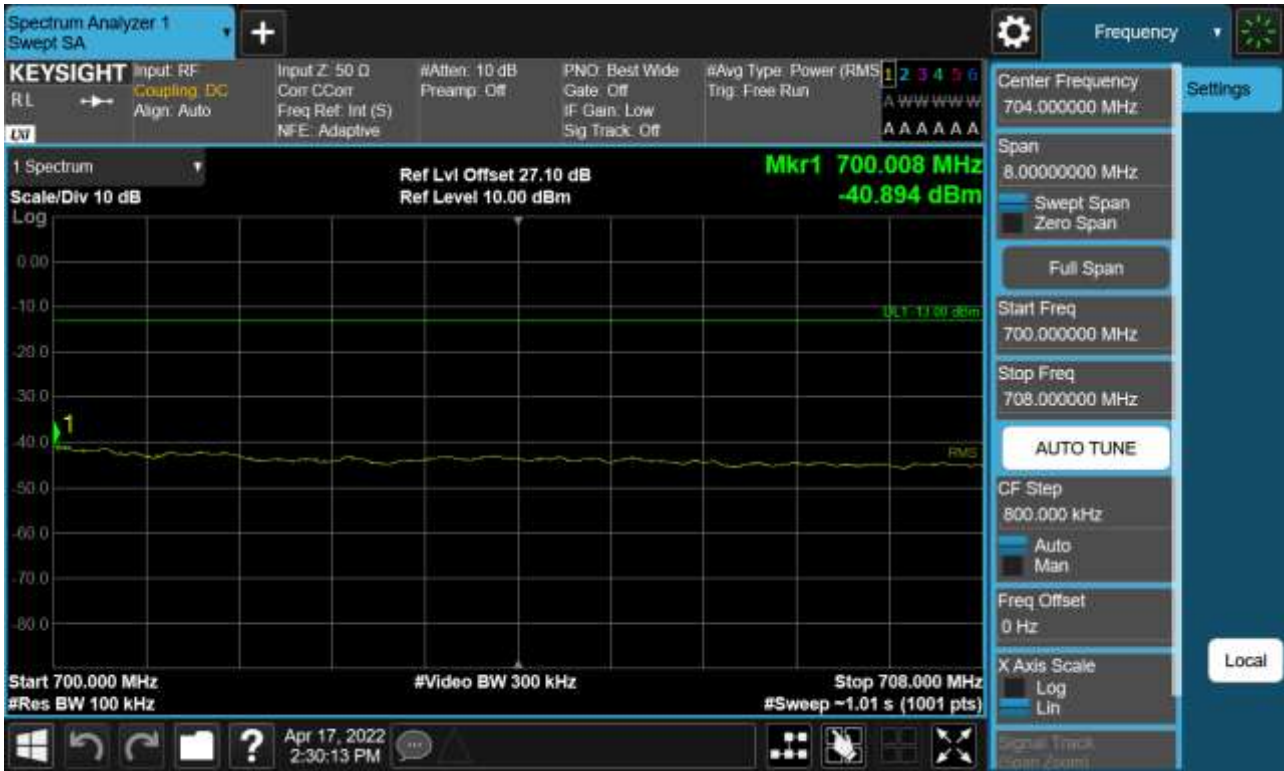
Sub6 n71. Upper Extended Band Edge Plot (15 M BW Ch.138100 BPSK_ Full RB)
