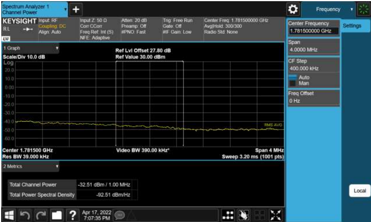
Sub6 n66. Upper Extended Band Edge Plot (15 M BW Ch.354500 BPSK_ Full RB) -3
