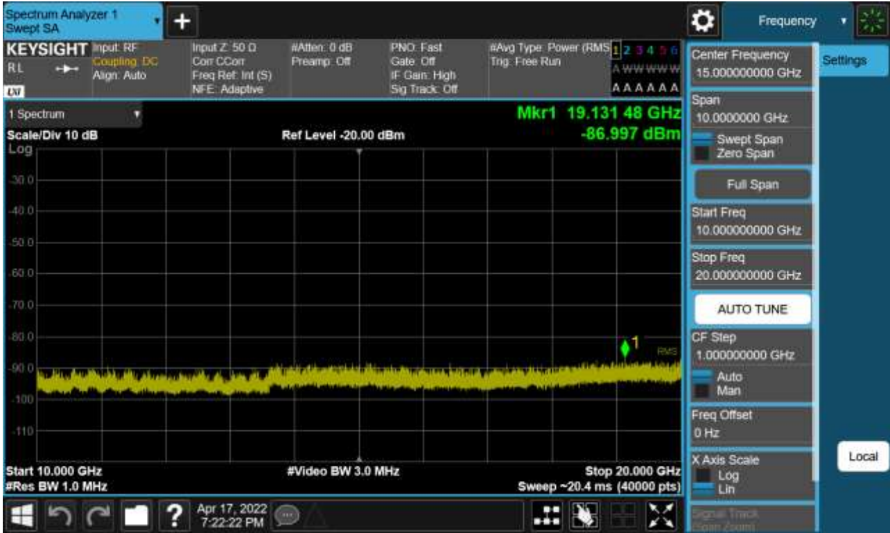
Sub6 n66. Conducted Spurious Plot_2 (345000ch_30 MHz_BPSK_RB 1_1)
