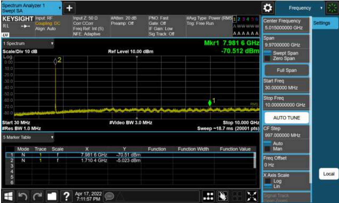
Sub6 n66. Conducted Spurious Plot_1 (344000ch_20 MHz_BPSK_RB 1_1)
