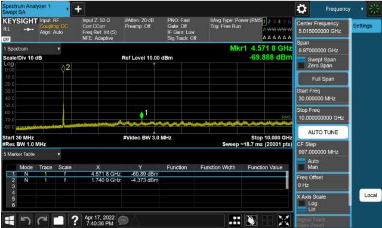
Sub6 n66. Conducted Spurious Plot_1 (352000ch_40 MHz_BPSK_RB 1_1)
