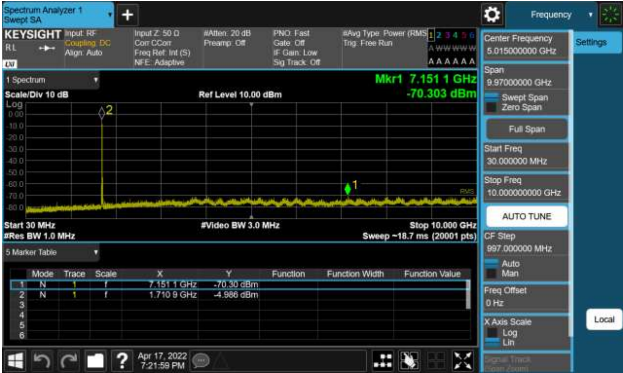
Sub6 n66. Conducted Spurious Plot_1 (345000ch_30 MHz_BPSK_RB 1_1)
