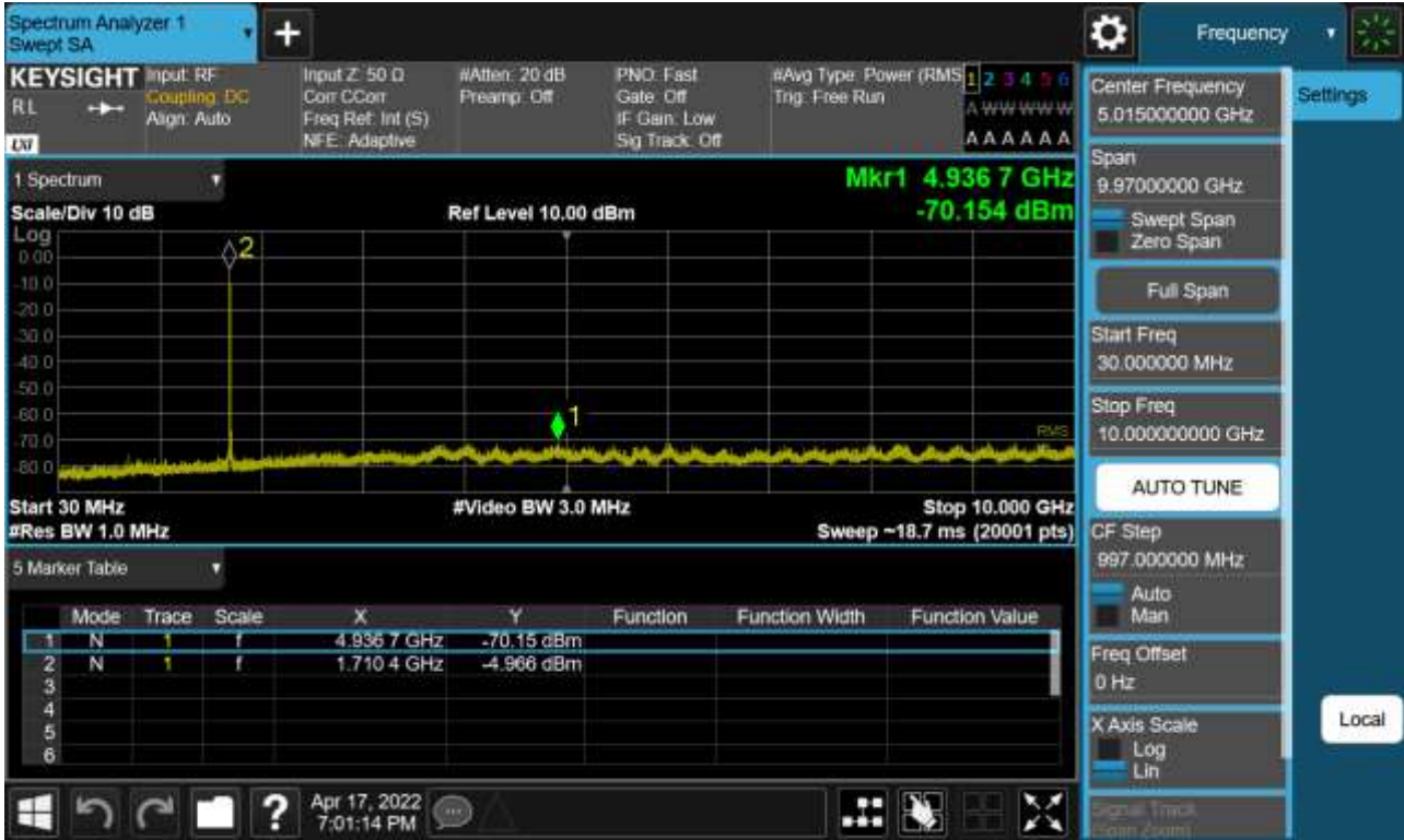
Sub6 n66. Conducted Spurious Plot_1 (343500ch_15 MHz_BPSK_RB 1_1)
