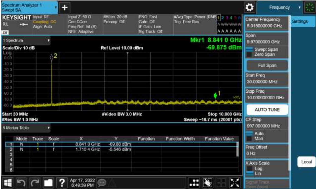
Sub6 n66. Conducted Spurious Plot_1 (343000ch_10 MHz_BPSK_RB 1_1)
