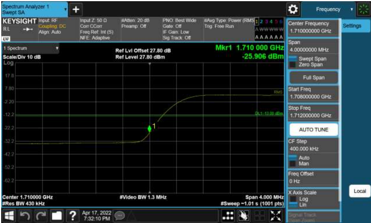
Sub6 n66. Lower Band Edge Plot (40 M BW Ch.346000 BPSK Full RB) -2
