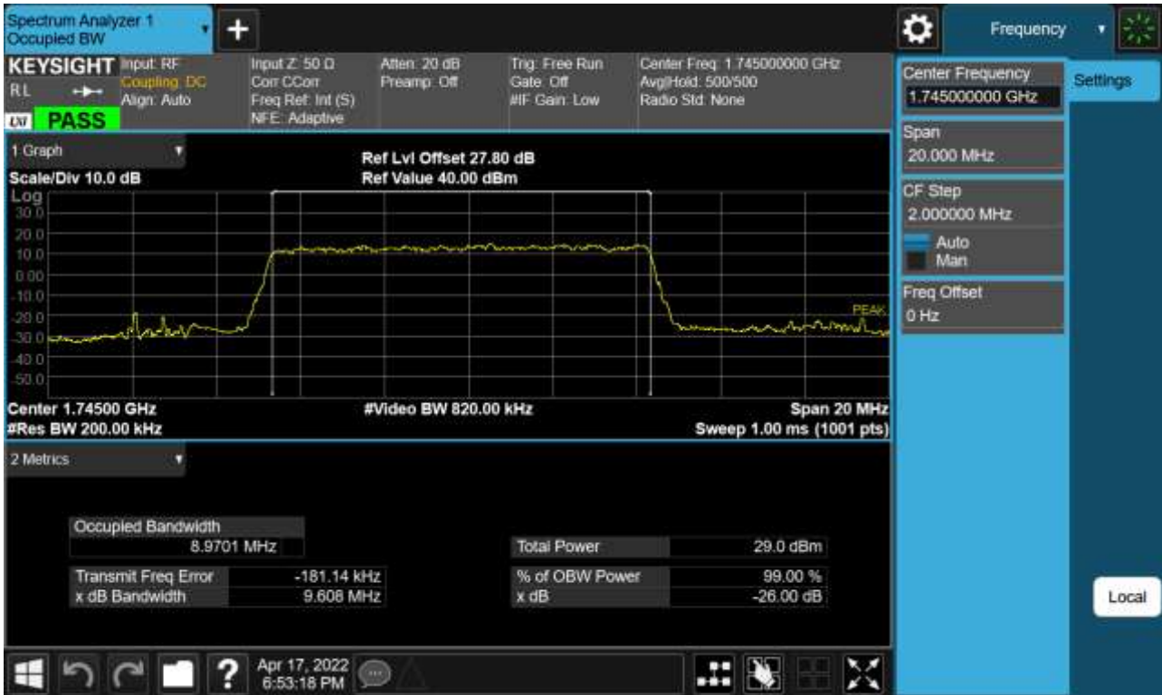
Sub6 n66. Occupied Bandwidth Plot (10 M BW Ch.349000 64QAM Full RB)
