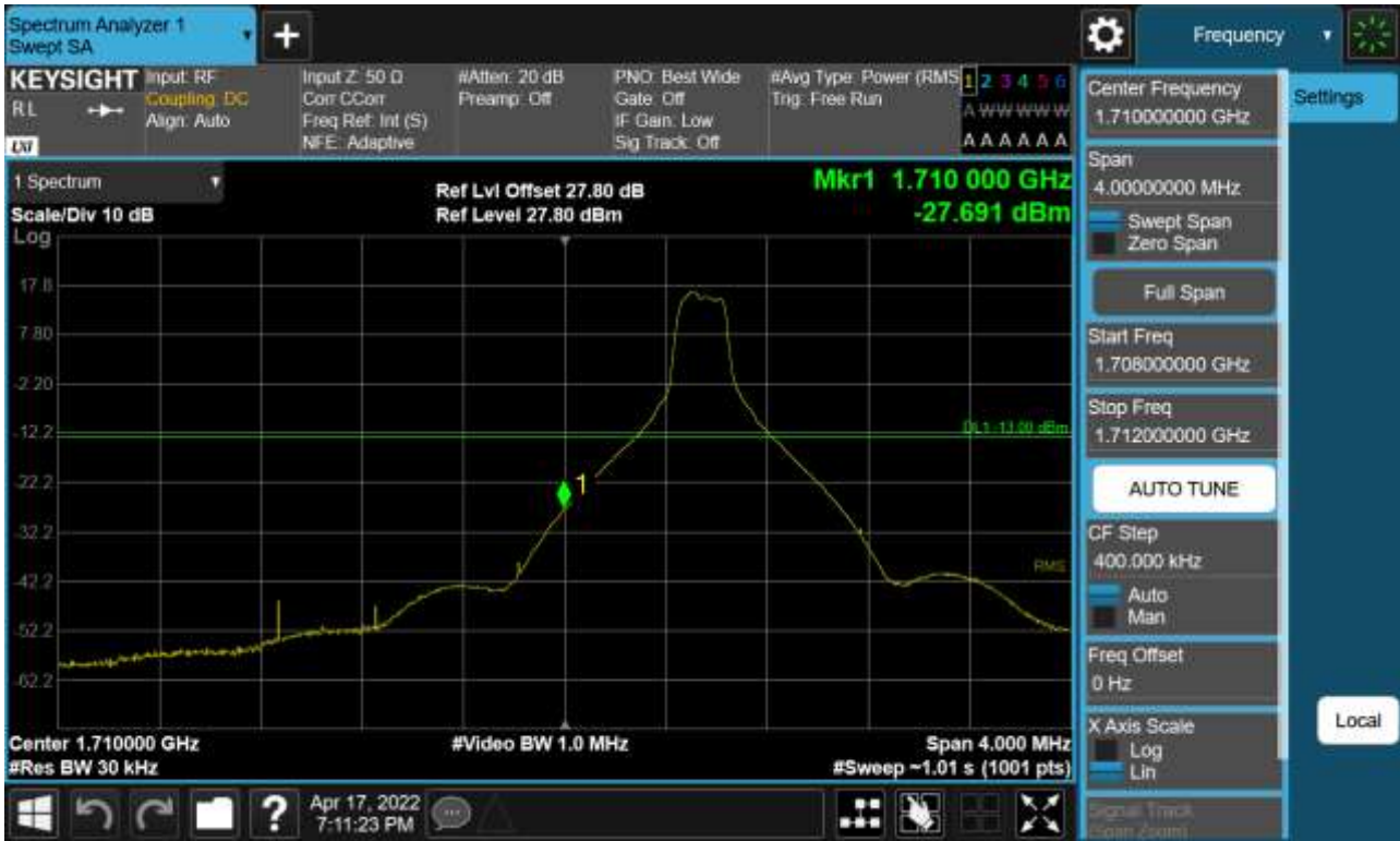
Sub6 n66. Lower Band Edge Plot (20 M BW Ch.344000 BPSK RB 1, Offset 0) -1
