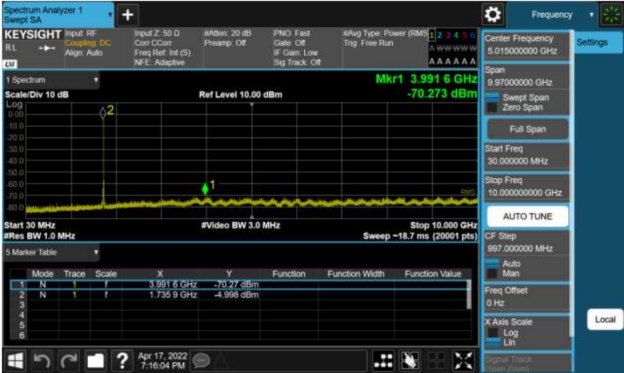
Sub6 n66. Conducted Spurious Plot_1 (349000ch_20 MHz_BPSK_RB 1_1)
