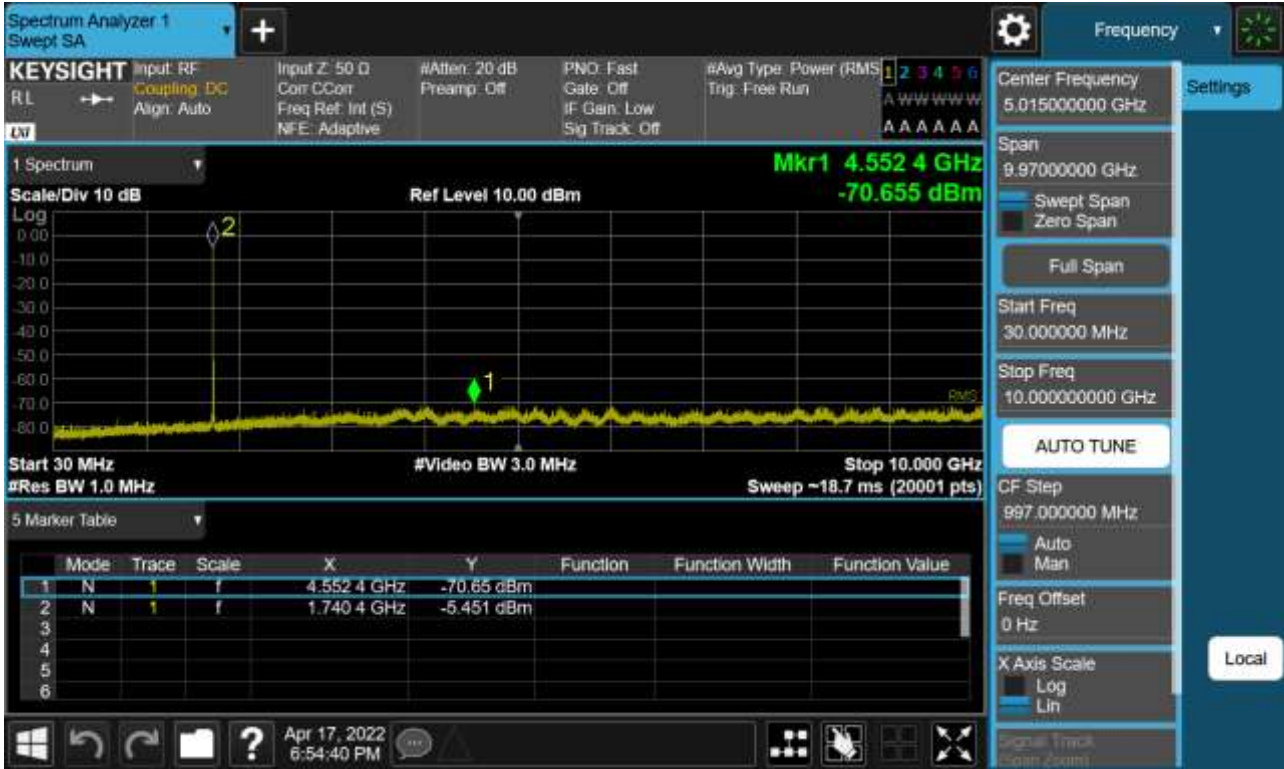
Sub6 n66. Conducted Spurious Plot_1 (349000ch_10 MHz_BPSK_RB 1_1)
