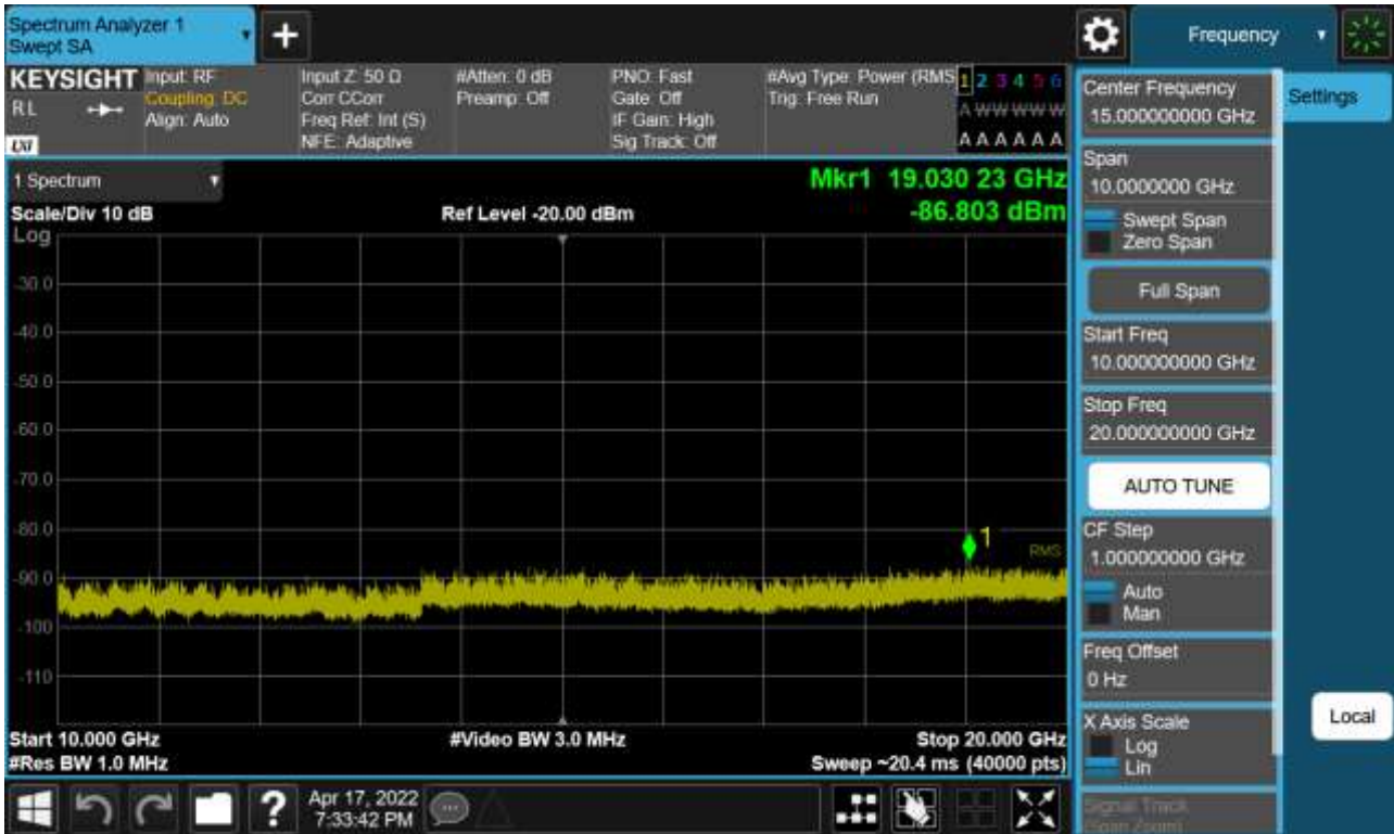
Sub6 n66. Conducted Spurious Plot_2 (346000ch_40 MHz_BPSK_RB 1_1)
