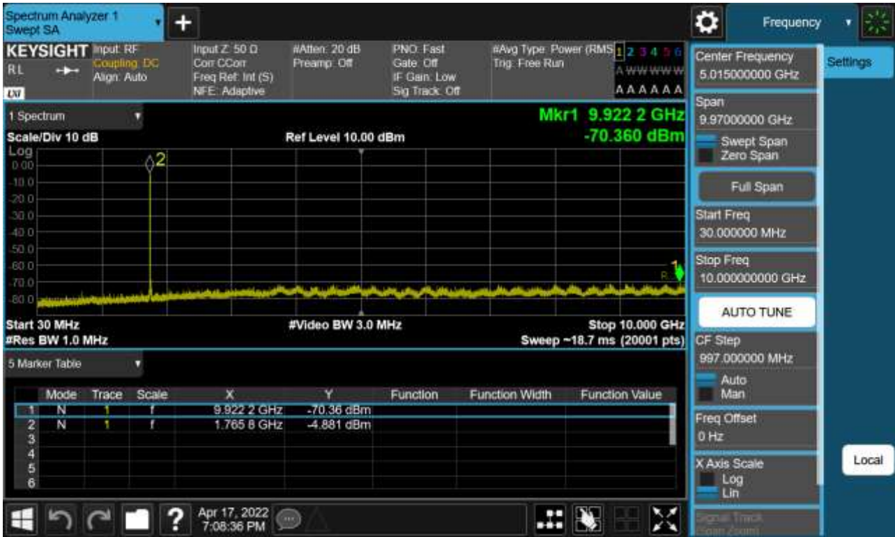
Sub6 n66. Conducted Spurious Plot_1 (354500ch_15 MHz_BPSK_RB 1_1)
